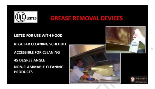
Grease removal devices must be listed for use with the cooking appliances. A regular schedule of cleaning should be established based on the accumulation of grease. The filters should be easily accessible and removable for cleaning and installed at an angle not less than 45 degrees from the horizontal. Any solutions used for cleaning must be non-flammable.
