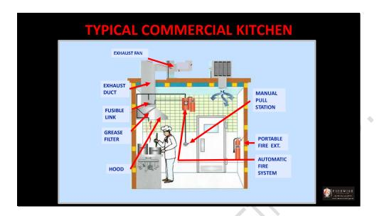
In this Unit we will discuss hood systems required over commercial cooking equipment, the purpose of grease filters and the various types, fusible links that melt to cause activation of the automatic fire suppression system, manual pull stations to activate the system, the exhaust duct and the exhaust fan and the "K" class portable fire extinguisher that is required in the kitchen.
