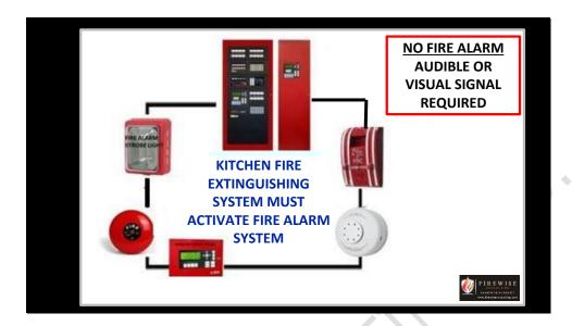
If the building is equipped with a fire alarm system activation of the kitchen fire extinguishing system must automatically activate the fire alarm. In buildings without a fire alarm system an audible alarm or visual indicator must provide notification that the system has activated.
