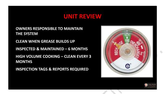
It is important to remember that it is the owner's responsibility to inspect, test and maintain the commercial kitchen operations. Any time there is a grease buildup the system must be cleaned. In most cases regular cleaning should be done by a qualified person every 6 months. One exception is high volume cooking in 24 hour operations which need to be cleaned every 3 months.
