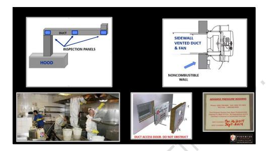
Kitchen duct systems vent directly above the roof or through non-combustible side walls. If the duct is not straight inspection panels must be installed at each change in direction and at each floor level. The inspection panels should be marked "Access Panel-Do Not Obstruct" and be large enough to allow for proper cleaning. When the cleaning company removes access panels for cleaning a label or tag with the company name and date must be provided near the affected access panel.
