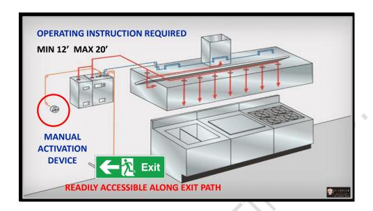
Manual activation of the automatic fire extinguishing systems must also be possible. At least one activation device must be located a minimum of 12' and a maximum of 20' feet from the kitchen appliance being protected. It must be readily accessible and should be located along the path of travel to an exit to prevent a person being trapped. Instruction must be provided to employees on the use of the manual activation device for the fire extinguishing system.
