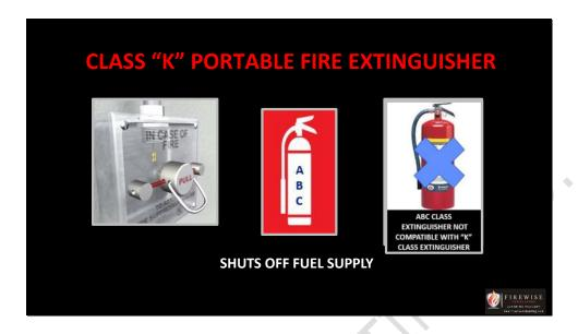
The automatic kitchen fire suppression system protects the hood, duct, and appliances from fire. The combination of the kitchen fire suppression system and a Class "K" wet chemical extinguisher provides additional protection against a fire that could result in temporary or permanent loss of business.
