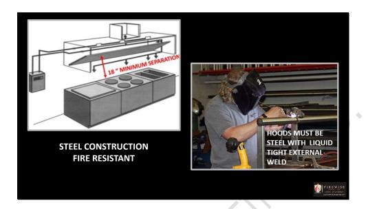
At least 18 inches of clearance is required between the grease filter and the cooking surface.
