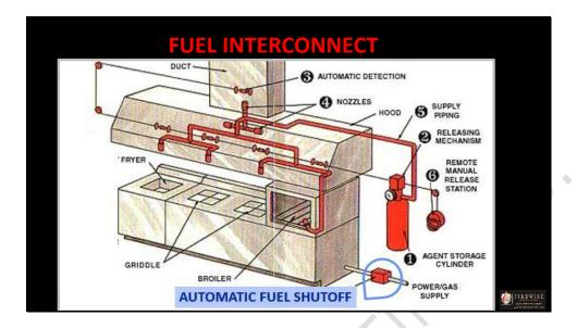
Another component of the system is the fuel and electric power shutoff. Upon activation of the fire extinguishing system the fuel supply and electric power to the cooking appliances must automatically shut off. The shutoff device must be manually reset after each activation.
