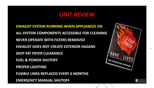
Exhaust systems must be operating whenever the cooking appliances are on. All exhaust system components including the fan must be accessible or have removable access panels for cleaning and inspection.
