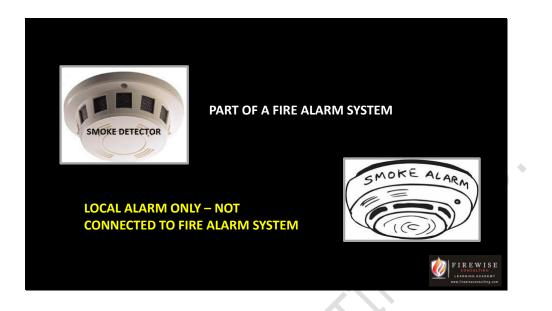
A smoke detector is a device that senses smoke, typically as an indicator of fire. Smoke detectors are part of a fire alarm system that, when activated, sends a signal to the fire alarm control panel. Smoke alarms on the other hand are a local alarm only and are not connected to the fire alarm system.
