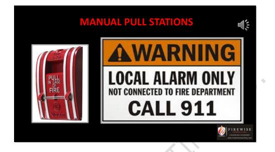
A pull station, when activated, initiates an alarm on a fire alarm system. In its simplest form, the user activates the alarm by pulling the handle down, which completes an electrical circuit and locks the handle in the activated position, sending a signal to the fire alarm control panel.
