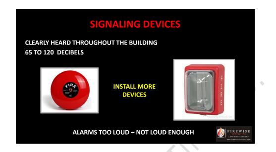
Fire alarm evacuation signals generally consist of a fire alarm gong or bell combined with visual strobe lights for the hearing impaired and are located in all common areas of the building.
