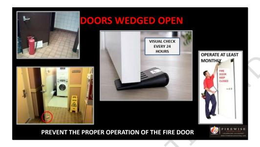
Objects like this fire extinguisher should never be used to keep the door in the open position because they prevent the door from closing and allow the fire to spread unchecked.
