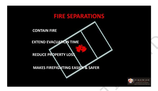
Fire separations are intended to contain the fire in the room where it started. If they work effectively they will extend the time people have to safely evacuate the building. When fire separations contain the fire they reduce the amount of fire loss to the structure making it easier to repair and put back in use. Fire separations also make it safer for firefighters as they act as a barrier to fire travel.
