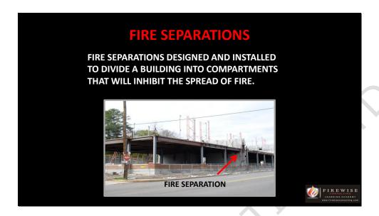
Fire separations are designed and installed in the construction phase to divide a building into compartments that will inhibit the spread of fire. They are part of the building design and construction but must be maintained after the building is occupied to work effectively.
