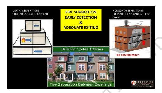
Fire separations along with early fire detection and adequate exiting are the three most import aspects of a fire safe building. Fire separations are structural elements made in accordance to building code requirements that prevent the spread of fire for a given period of time. Fire separations are provided in buildings to limit the spread of fire and the premature collapse of the building under fire conditions.
