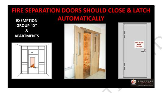
If the door does not close fire, smoke and hot gases can quickly spread to the rest of the compartment.
