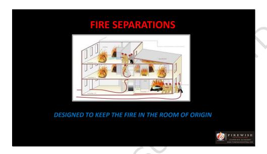
Fire separations are designed to divide buildings into compartments so that a fire starting in one area will not spread to other compartments in the building.
