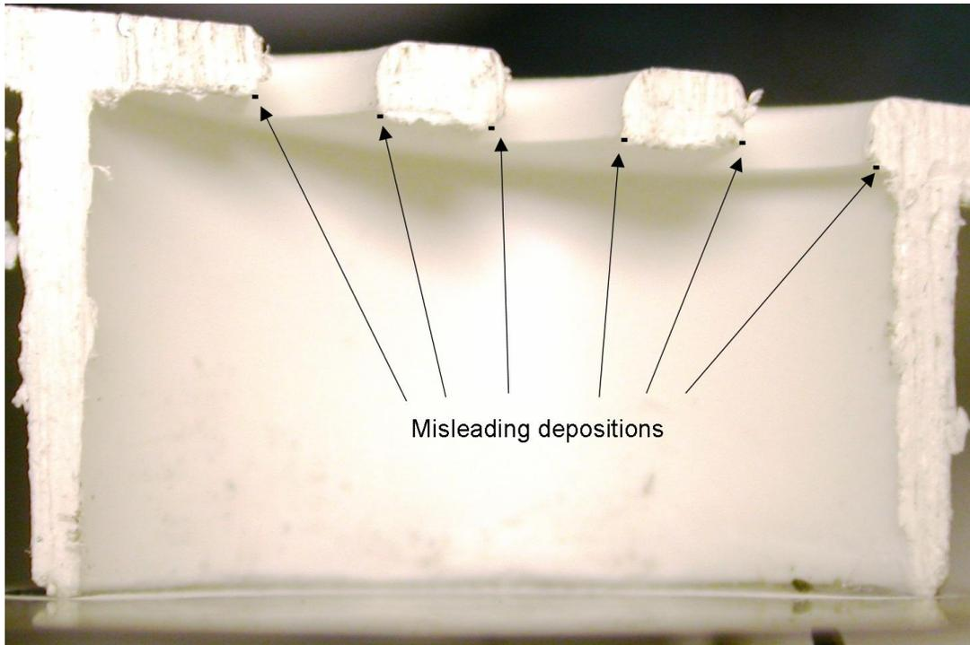
**Figure 7.17 This is a cross-section of an FBI horn chamber with an illustration of misleading depositions on the corners between the internal and vertical faces of the smoke alarm horn opening. The markings in the figure are roughly proportional to the actual width of the misleading depositions. Note the extension of the deposits into the horn opening and the positioning of the deposition more on the corner than either of the sheer faces.**
