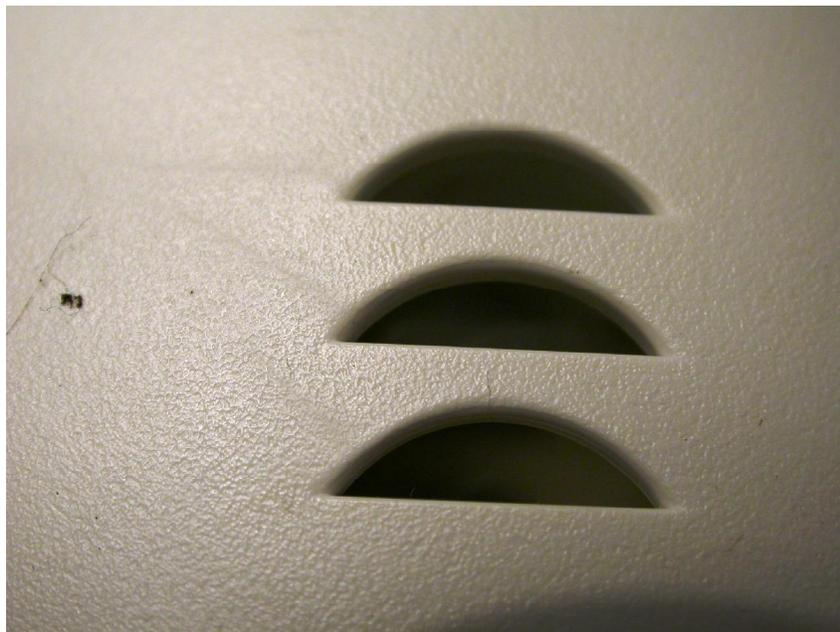
**Figure 22.6** This is a macroscopic view of the alarm horn openings from the alarm pictured in figure 22.5. This alarm did not sound during the exposure and shows no evidence of enhanced deposition.
