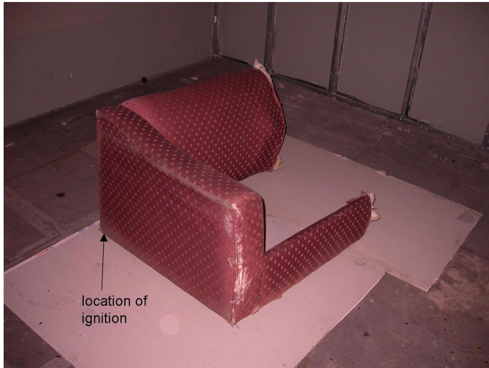
**Figure 6.20** This figure shows the couch section used in Experiment 4.2, pre-test. The couch was ignited with a butane lighter in the location labeled. Most of the couch was consumed before it was extinguished.
