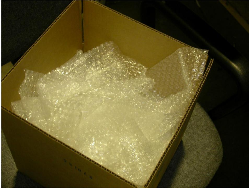
**Figure 6.14 One of the boxes with cups and bubble wrap that was burned in the flaming box with cups test fire in Test Series 3.**
