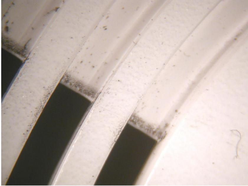
**Figure 17.33** This is a macroscopic view of the horn openings from Figures 17.31 and 17.32. This alarm sounded during exposure to a flaming polyurethane source. There is evidence of enhanced soot deposition on the short edges of all of the alarm horn openings.
