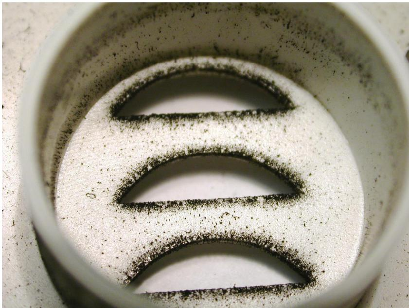
**Figure 23.4** This is a macroscopic view of the interior face of the alarm horn opening from Figures 23.1-23.3. The enhanced soot deposition is more developed on the interior face than the exterior face.
