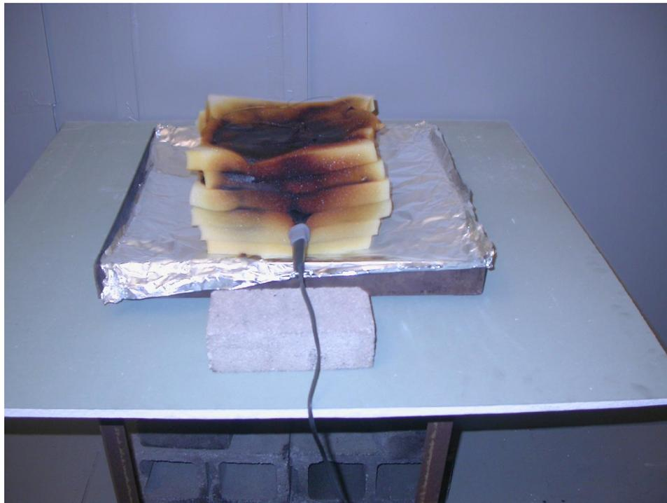
**Figure 7.2 Smoldering polyurethane source from Experiment 1.2 post-test. This reformatted source caused all 5 of the enabled alarms to sound.**
