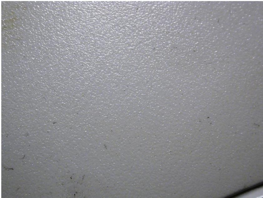
**Figure 17.20** This figure shows the level of ambient soot deposited on the cover of the alarm pictured in Figures 17.14-17.19 (photo at the same magnification as Figure 17.19). The density of soot deposited farther from the opening is lower than the density of soot in the pattern of enhanced soot deposition from the previous figure.
