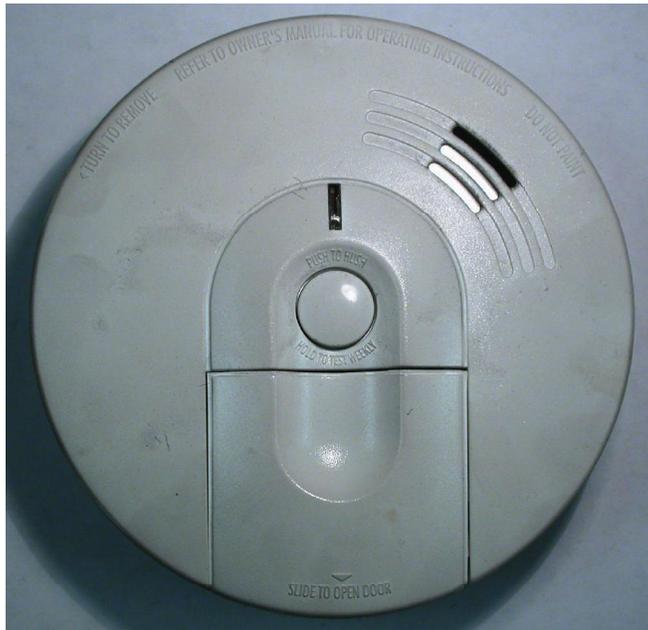
**Figure 17.18** This is the exterior of the cover of an FACI alarm that sounded during exposure to a flaming polyurethane fire.
