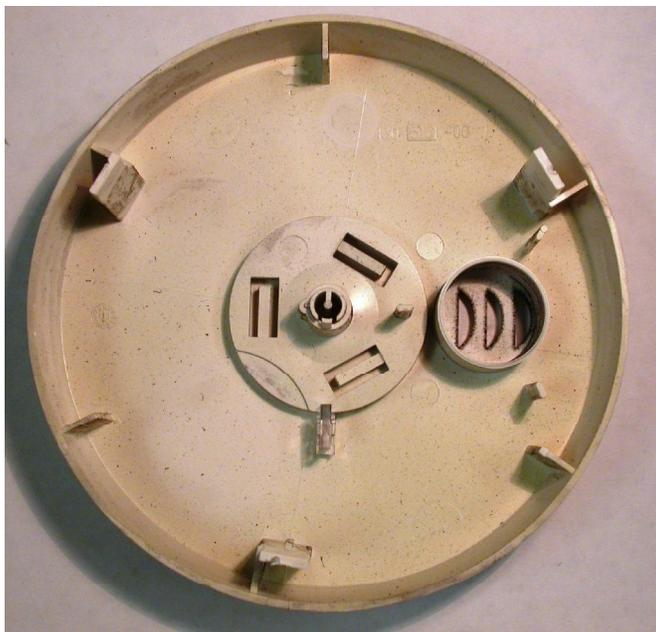
**Figure 17.5** This figure contains a view of the interior of the alarm cover from the alarm pictured in Figures 17.1-17.6. This alarm has been exposed to smoldering and flaming polyurethane sources, visible by the staining and carbonaceous soot depositions. The enhanced soot deposition on the interior faces of the horn openings is barely visible in this figure.
