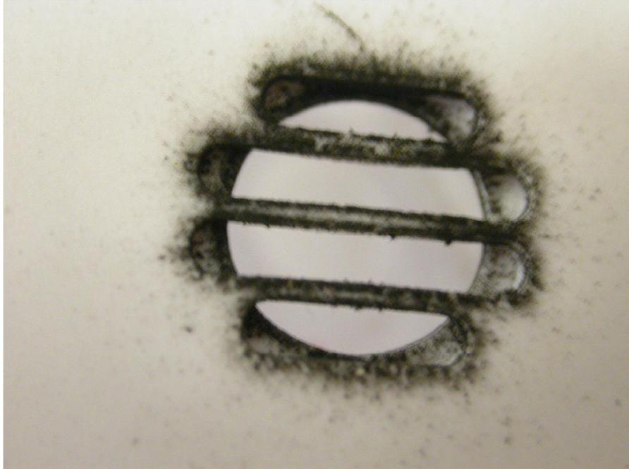
**Figure 7.6** An example of an enhanced soot deposition pattern with radial characteristics on the external face of an FSBI horn opening. This occurred on an alarm that sounded during exposure to a flaming polyurethane source.
