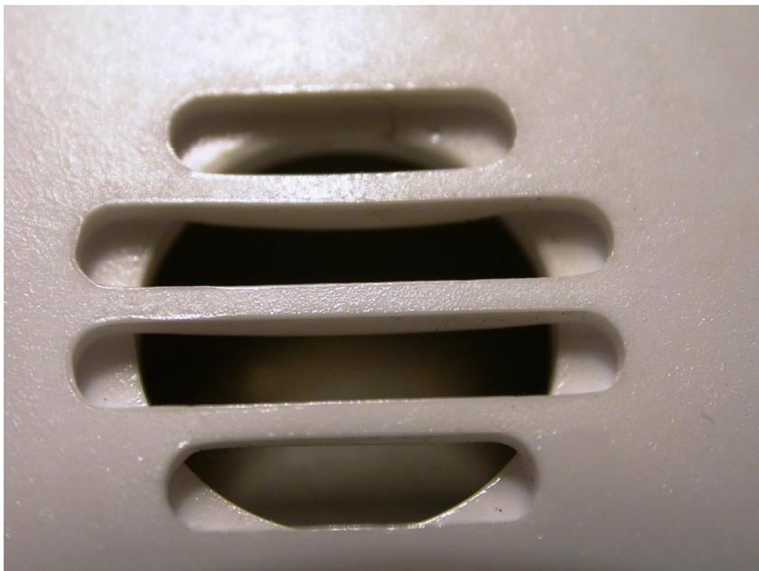
**Figure 22.20** This figure shows a macroscopic view of the horn openings from Figure 22.19. This alarm did not sound and does not show any evidence of enhanced depositions.
