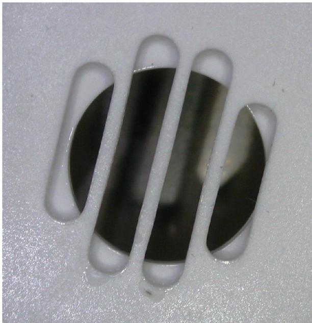
**Figure 19.8** This figure is a macroscopic view of the alarm horn openings of the alarm pictured in Figure 19.8. This alarm sounded during multiple nuisance exposures but does not show evidence of enhanced soot deposition.
