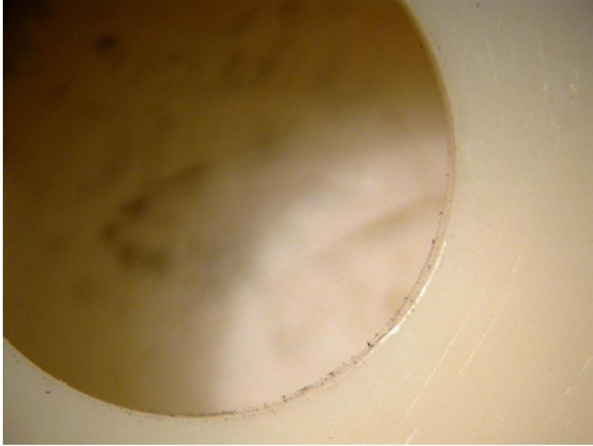
**Figure 17.17** This is a microscopic view of the horn from the alarm pictured in Figures 17.14-17.17. There is some soot deposited on the horn, but no evidence of enhanced soot deposition indicative of sounding.
