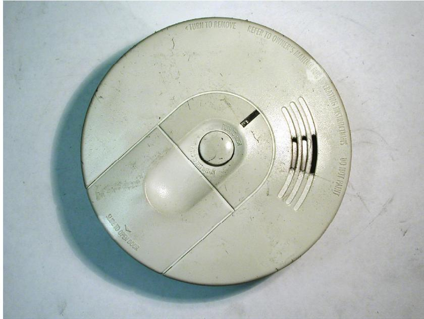
**Figure 23.7** This figure shows the external cover of an FACI alarm that sounded during exposure to the flaming couch section.
