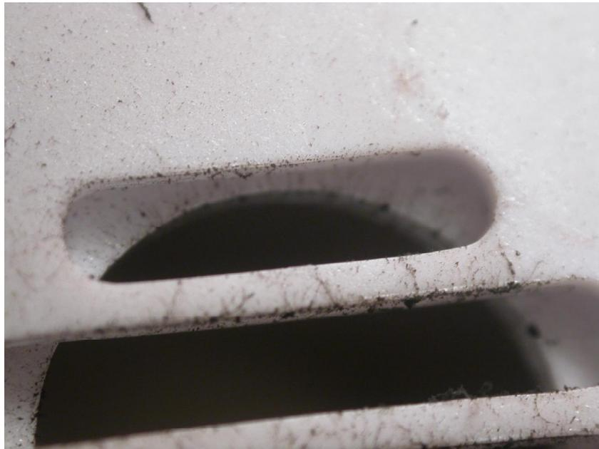
**Figure 21.26** This is a microscopic view of the alarm horn openings from Figure 21.26. This alarm did not sound shows soot deposition commensurate with exposure to a high soot yield fire, but not enhanced soot deposition indicative of sounding.
