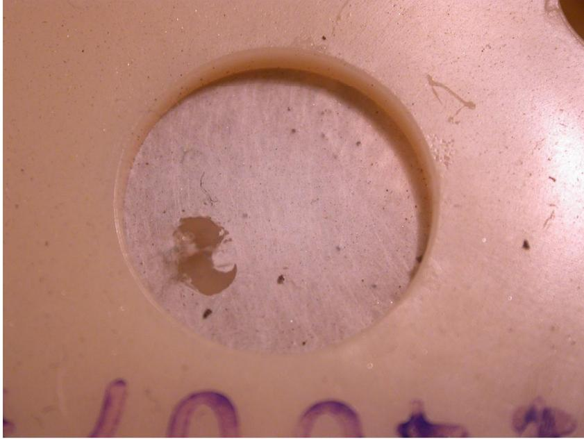
**Figure 22.21** This figure shows a macroscopic view of the horn opening of a used alarm. The alarm horn was covered by a cocoon that had a hole in it. This picture is prior to exposure to the smoldering to flaming cabinet assembly fire.
