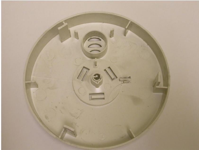
**Figure 13.9** This figure contains a view of the entire internal cover of the smoke alarm. There is some evidence of soot deposition on the cover, but no evidence supporting the direction of bulk flow of smoke through the alarm.
