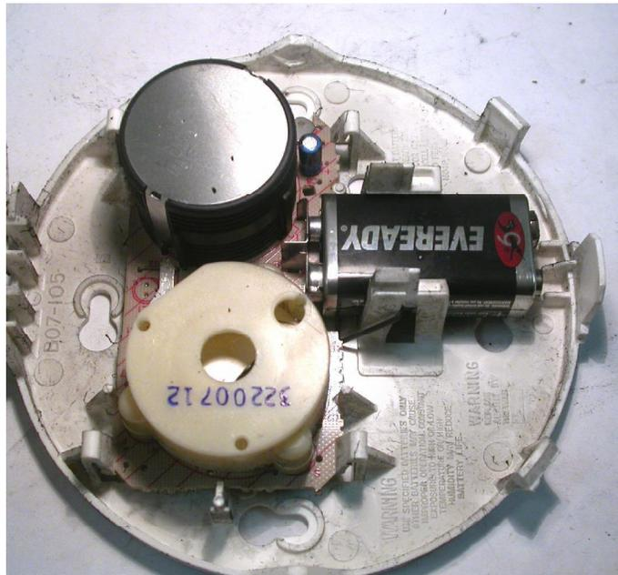
**Figure 21.20** This figures shows the interior of an alarm that did not sound during exposure to the flaming box with cups fire.
