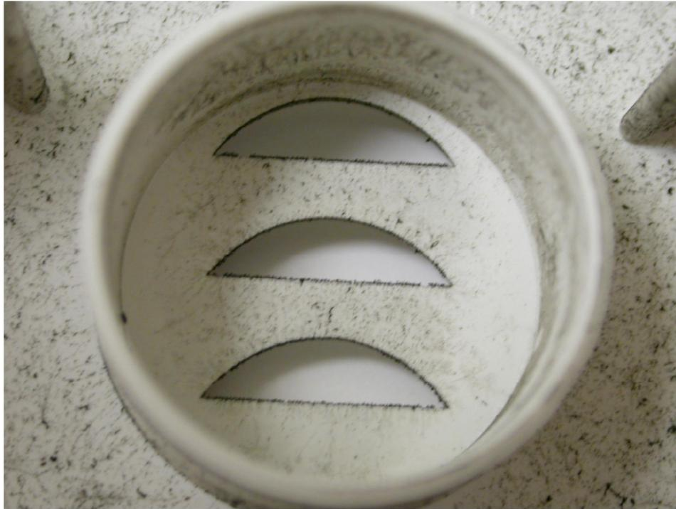
**Figure 7.15 Potentially misleading deposition on the internal face of an FBI style horn opening. This is representative of an alarm that did not sound during exposure to a flaming polyurethane source.**
