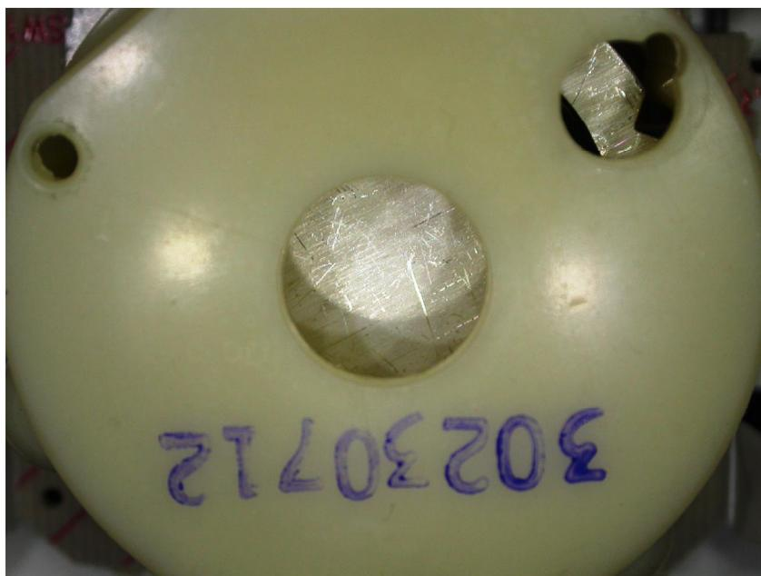
**Figure 20.6** This is a macroscopic view of the alarm horn openings from the alarm pictured in Figure 20.5. This alarm sounded but does not show any evidence of enhanced soot deposition.
