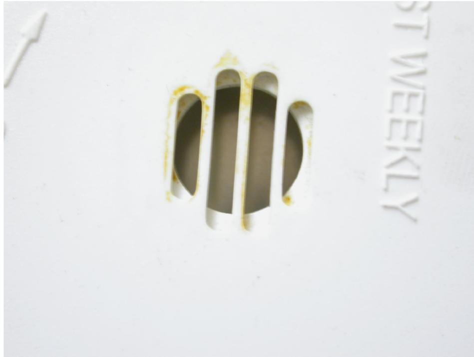
**Figure 7.9 An example of a "Tarry" pattern on the external face of an FSBI style horn opening. This is indicative of a smoke alarm that sounded during exposure to a smoldering polyurethane source.**
