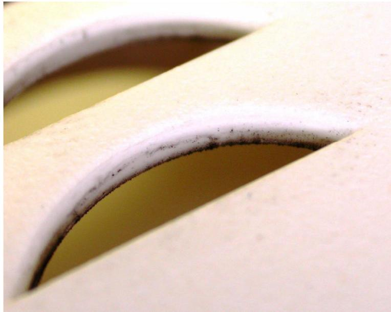
**Figure 13.6 This figure shows another view of a single vertical face of the alarm. The deposition is again denser than was seen on the alarm cover or external face, especially toward the corners of the moon shapes. The deposition density changes from higher to lower density moving from the internal to external face of the horn opening.**
