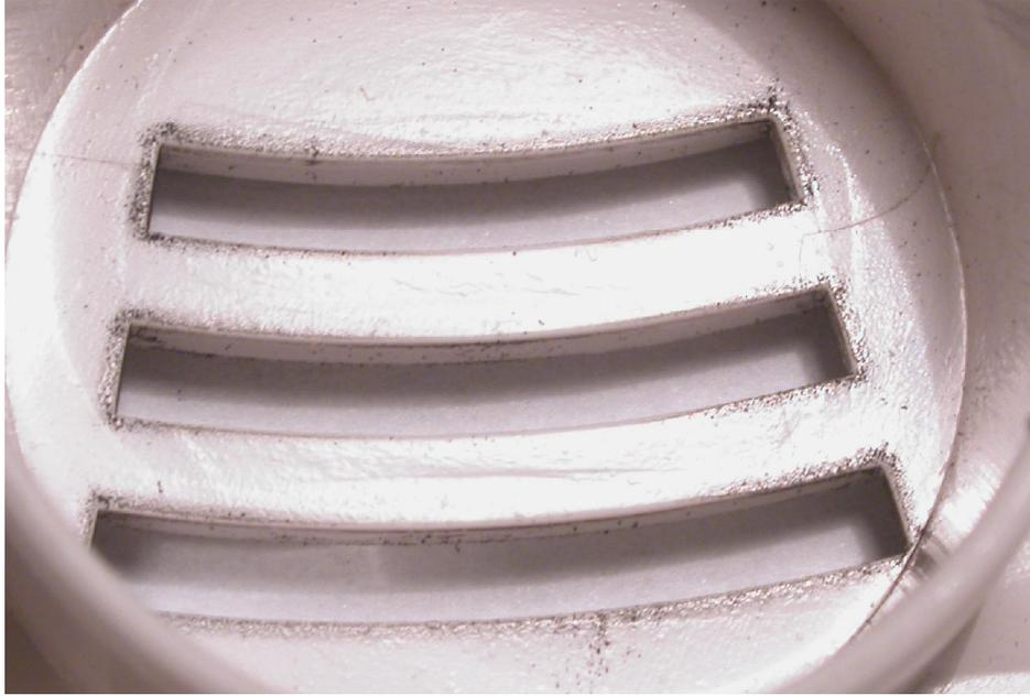
**Figure 17.35** This is a macroscopic view of the interior face of the alarm pictured in Figures 17.31-17.34. There are rings of enhanced soot deposition visible around the horn openings. The enhanced soot deposition is more distinct on the interior face than the exterior face, Figure 17.32.
