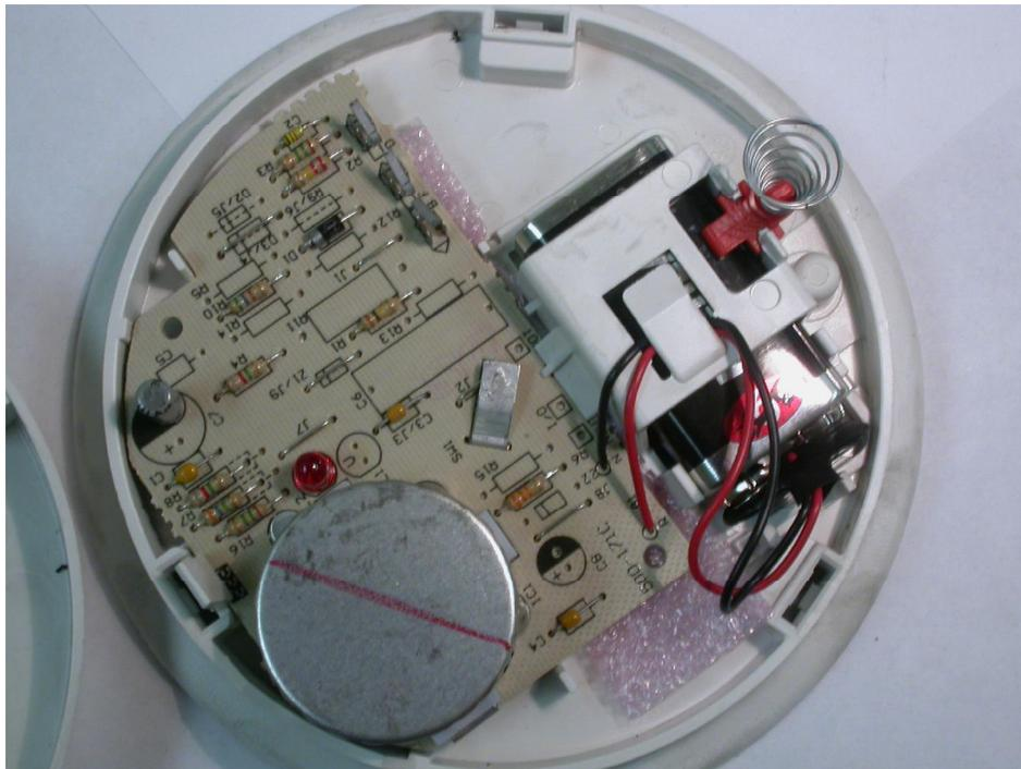
**Figure 13.8** This figure shows a macro view of the components of the smoke alarm after the cover has been removed. There is little evident soot deposition on the alarm components and no evidence of bulk flow of smoke through the alarm.
