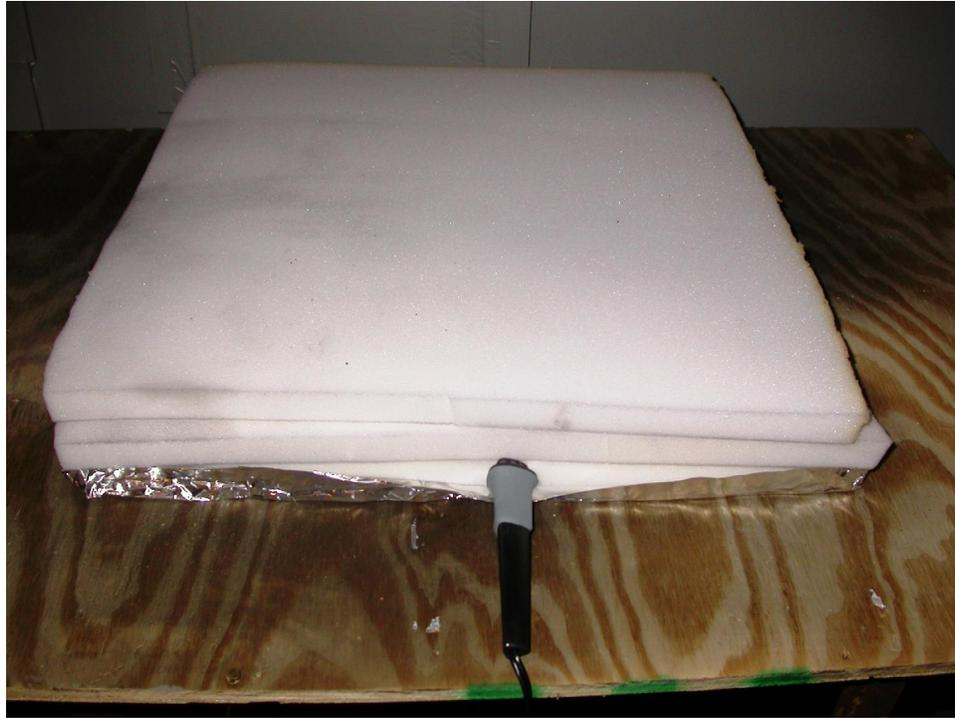
**Figure 6.3 Original smoldering polyurethane source prior to Experiment 1.1.**
