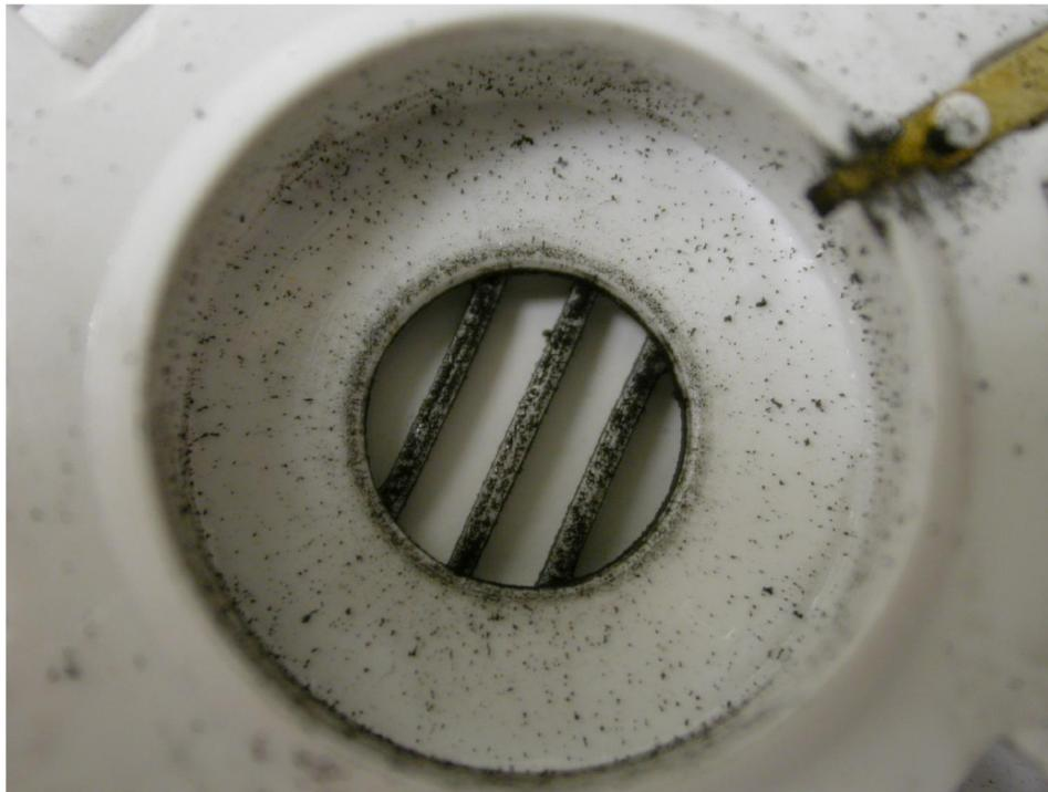
**Figure 7.5 An example of an enhanced soot deposition pattern with ring-like characteristics on the interior face of a FSBI smoke alarm horn opening. This enhanced soot deposition pattern occurred in an alarm that sounded during exposure to a flaming polyurethane source.**
