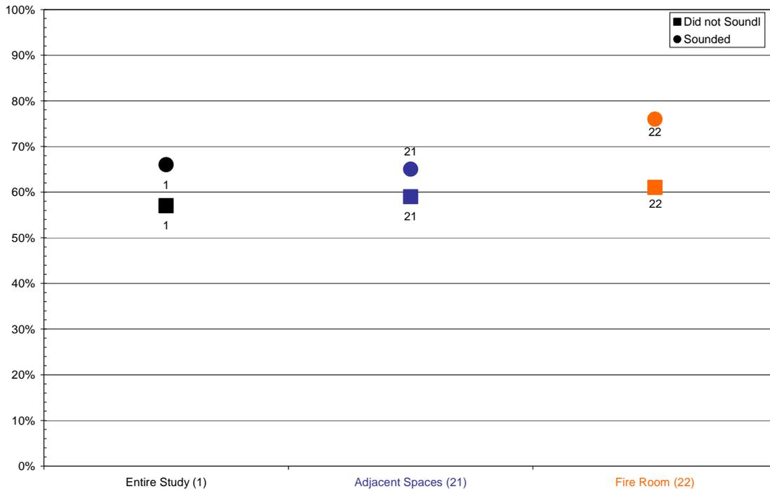
**Figure 8.9** The summary of percentage of alarms identified as having sounded and not having sounded during the blind study for the entire study and the populations separated by distance from source. This figure contains the percentages based on the number of alarms that sounded, 83, 55, and 25 respectively, and the number of alarms that remained silent, 68, 39, and 23 respectively, in each population.
