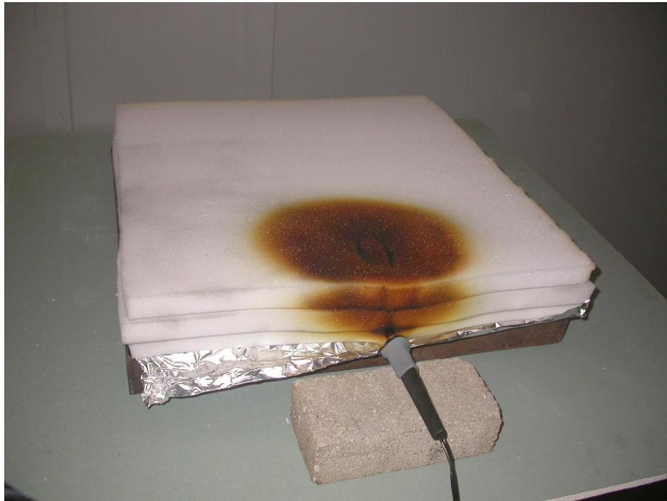
**Figure 7.1 This figure shows a smoldering polyurethane source from Experiment 1.1 post-test. No alarms sounded when exposed to this source.**
