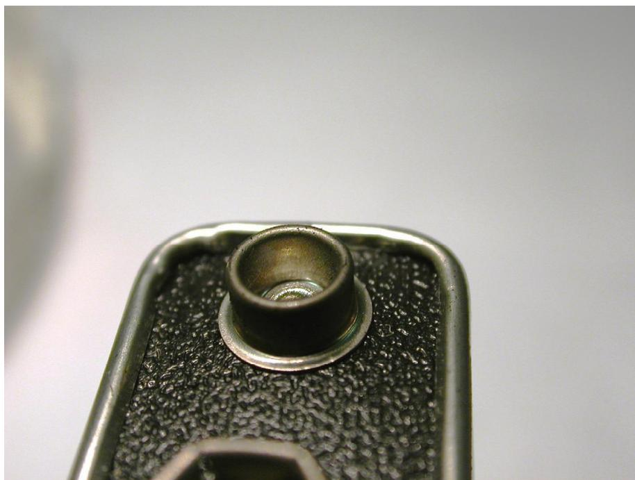
**Figure 14.4** Soot covering a battery terminal from a battery improperly installed in an FGFI alarm exposed in Experiment 4.2: Flaming Couch exposure. Soot could not have collected this way on the terminal of a properly installed battery, see Figure 14.2.
