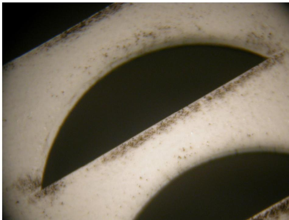
**Figure 7.10 This is enhanced soot deposition occurring in an FBI alarm sounding during exposure to flaming polyurethane. The corners of the enhanced deposition on this alarm is not uniform about the entire circumference, but was found to be comparable to Figure 18 in [Worrell, et al., 2003] and indicative of alarm sounding.**
