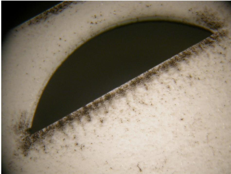
**Figure 7.8 This figure shows enhanced soot deposition that occurred on the external face of an FBI alarm horn when it sounded during exposure to a flaming polyurethane source. This pattern of enhanced soot deposition is not uniform around the entire horn opening, but displays the radial characteristics.**
