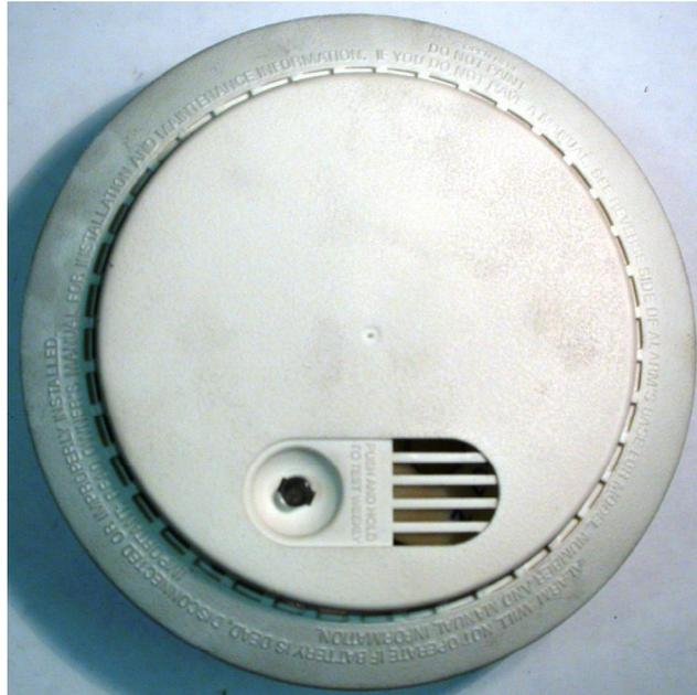
**Figure 17.10** This figure pictures the exterior cover of an FGBI alarm that sounded during exposure to a flaming polyurethane source.
