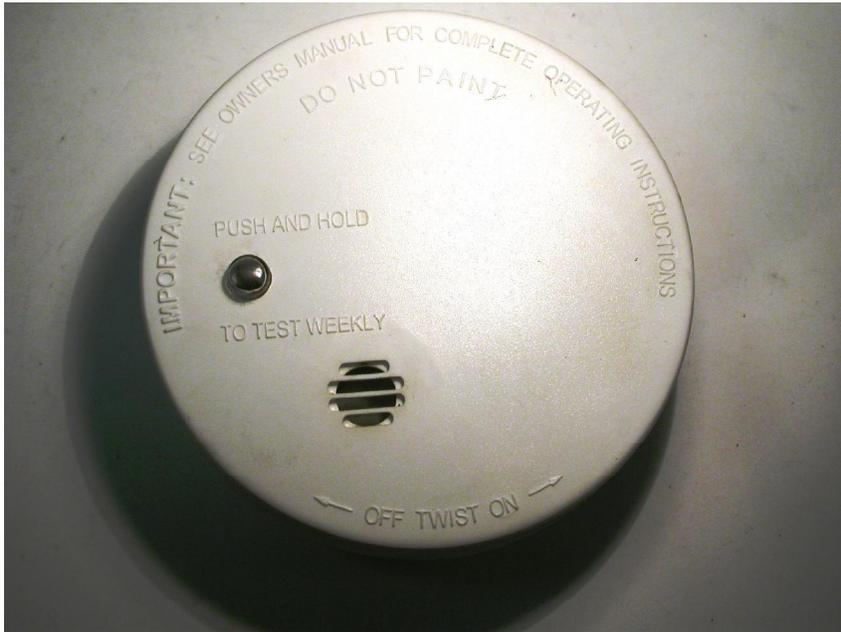
**Figure 22.16 This figure shows the external cover of an FSBI alarm that sounded during exposure to the smoldering to flaming cabinet assembly.**
