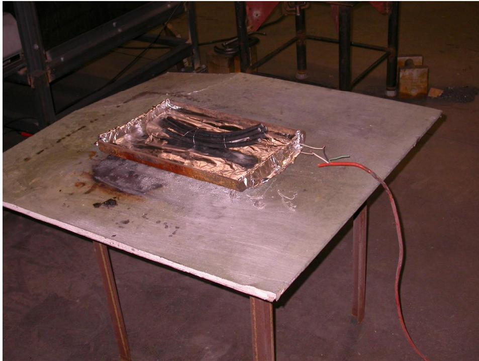
**Figure 6.12 A Cable bundle typical of that used for smoldering and flaming cable fires for Test Series 3.**
