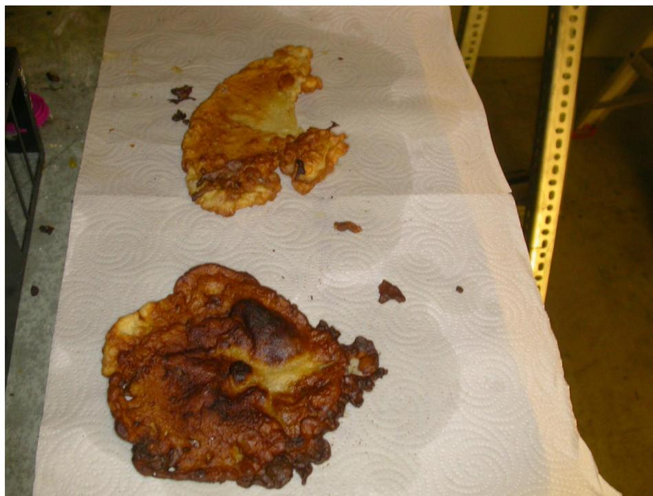
**Figure 6.10 Typical end product of batter fried during the deep-fried batter nuisance exposures of Test Series 2.**
