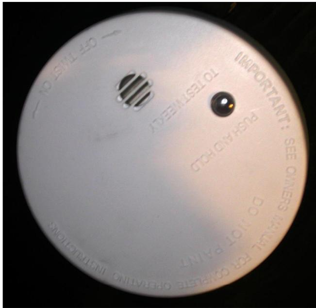
**Figure 20.7** This figure shows the cover of an FSBI alarm that sounded during exposure to a smoldering cable fire.
