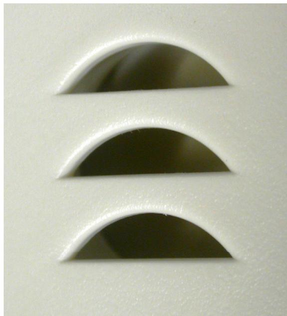
**Figure 19.2** This figure is a macroscopic view of the alarm horn openings of the alarm pictured in Figure 19.1. This alarm sounded during multiple nuisance exposures but does not show evidence of enhanced soot deposition.
