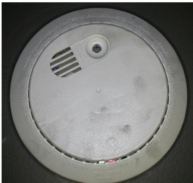
**Figure 19.5** This figure shows the exterior cover of an FGBI alarm that sounded during multiple nuisance exposures.
