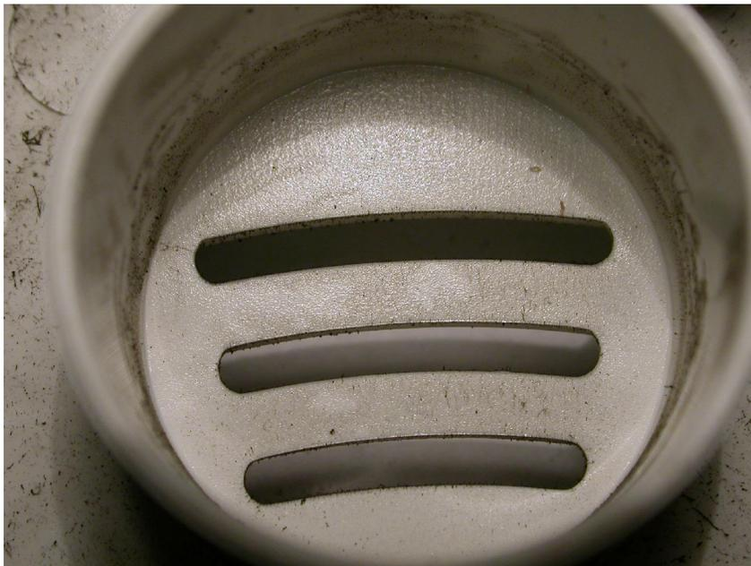
**Figure 23.12** This is a macroscopic view of the horn openings from Figures 23.9-23.10. This alarm did not sound during the exposure and does not show evidence of enhanced deposition. The soot deposited on the internal face of the alarm is similar in density inside and outside horn chamber on the same face.
