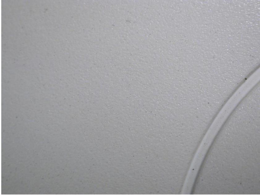
**Figure 17.23** This figure shows the level of ambient soot deposition on the external cover of the FACI alarm pictured in Figures 17.21 and 17.22.
