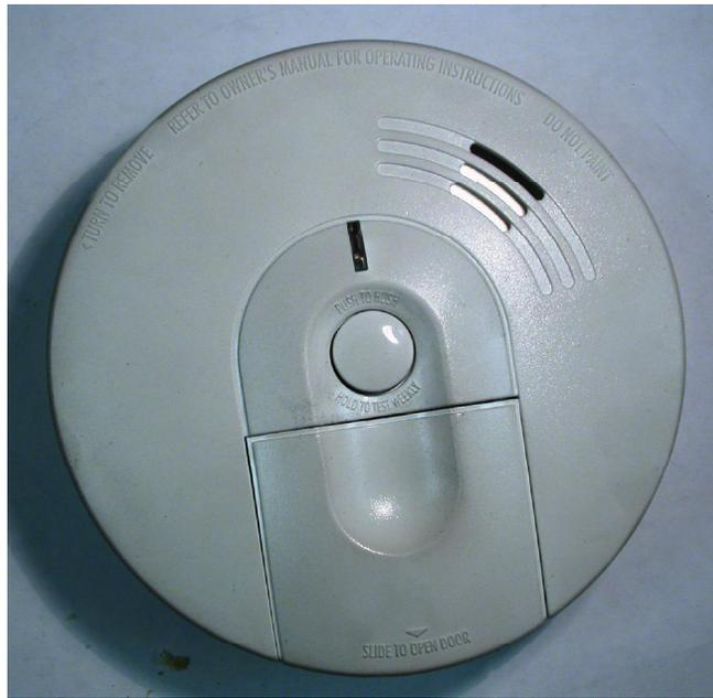
**Figure 17.21** This figure pictures the external cover of an FACI alarm that did not sound during exposure to a flaming polyurethane source.
