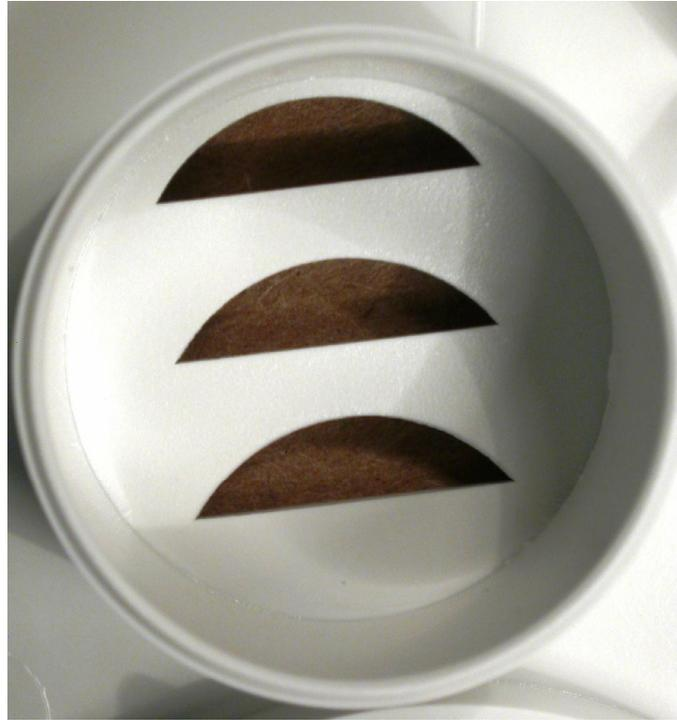
**Figure 0.15 Internal Face of a smoke alarm horn opening**
