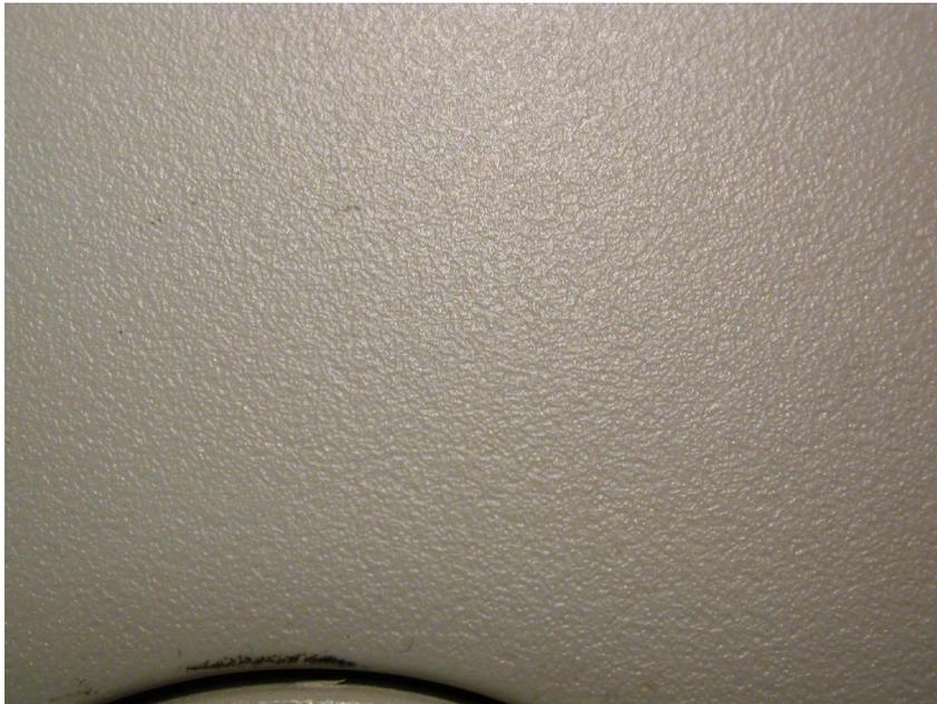
**Figure 18.4** This figure shows the ambient deposition on the exterior cover of the alarm in Figures 18.1-18.3.
