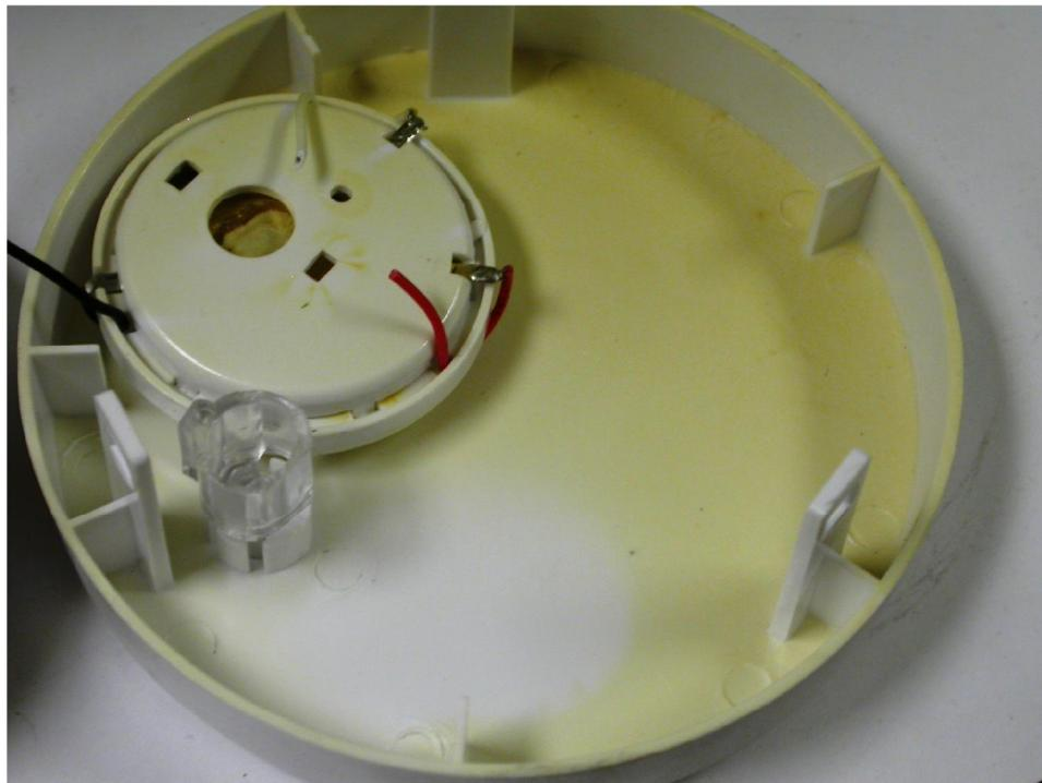
**Figure 14.1** The inside cover of an FSBI alarm exposed to a smoldering polyurethane source. The staining of the inside cover is indicative of exposure to a smoldering source, but reveals nothing about whether the alarm sounded or not.
