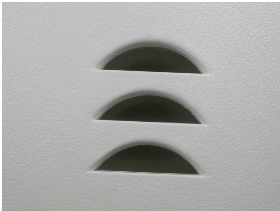
**Figure 0.7 Exterior of FBI Smoke Alarm Horn Opening.**
