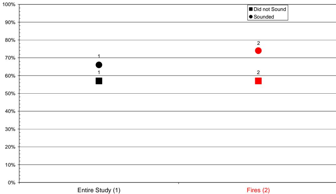
**Figure 8.5 Summary of the percent of the determinations made during the blind study to the entire study observations and the population composed of only the fire exposures. This figure contains the percentage results based on the number of alarms that sounded, 83 and 74 respectively, and that remained silent in each population, 68 and 68 respectively.**
