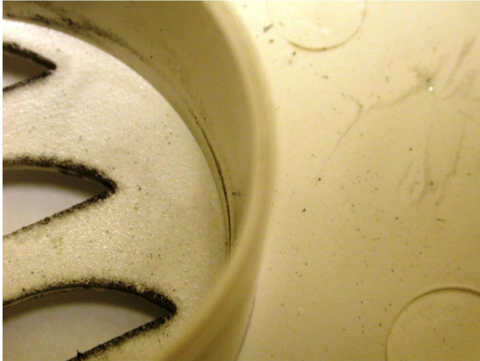
**Figure 13.12 This figure shows a view that is half inside and half outside the horn chamber. The enhanced deposition around the horn opening is visible on the left and the density of soot deposited inside the horn chamber is greater than or equal to that deposited outside the chamber. This observation verifies the identification of microscopic enhanced soot deposition on the internal face.**
