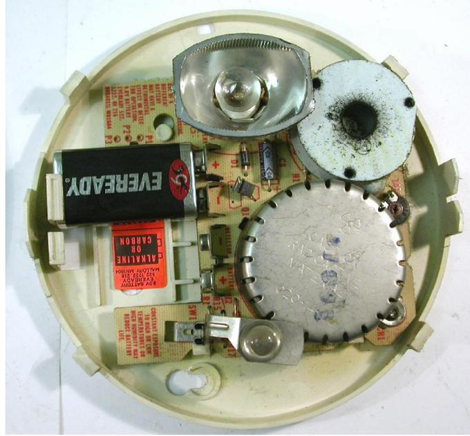
**Figure 23.25 This figure shows the interior of a used alarm exposed to the flaming couch section. This alarm sounded and shows enhanced soot deposition around the horn opening.**
