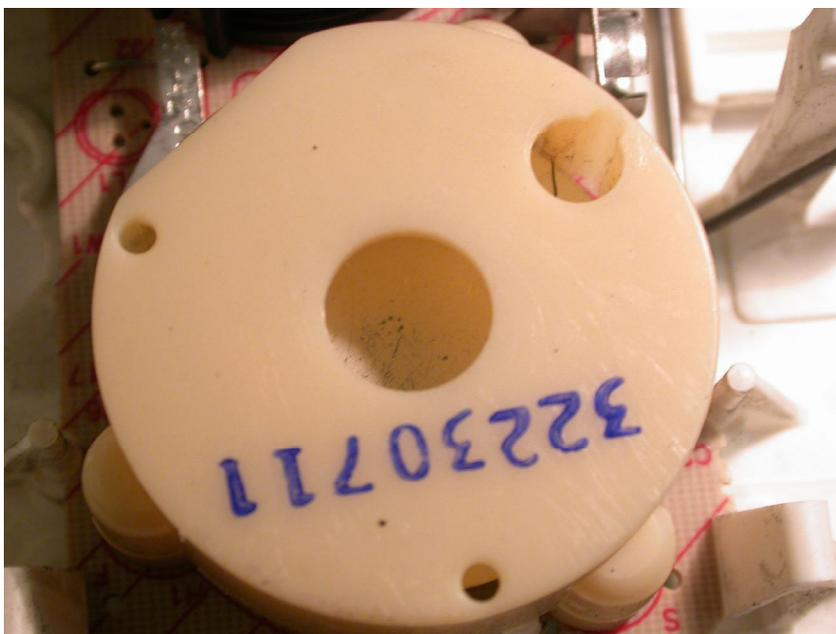
**Figure 16.7** This figure shows external face of an alarm that sounded during exposure to smoldering polyurethane source. There is no evidence of enhanced soot deposition indicative of sounding.
