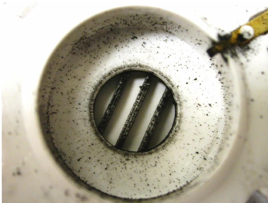
**Figure 7.28** An example of macroscopically observable enhanced soot deposition on the internal face of an FSBI alarm. This is representative of an alarm sounding during exposure to a flaming polyurethane source.
