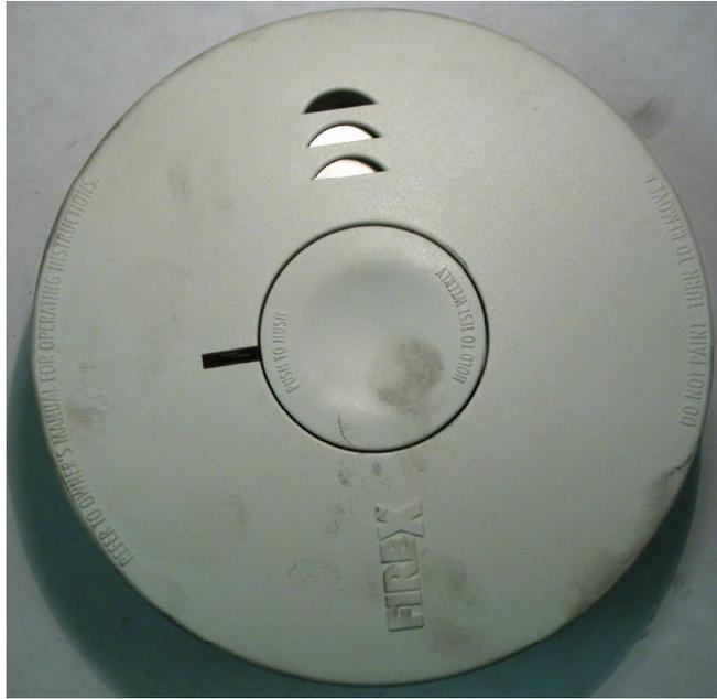
**Figure 18.1** This figure shows the outer cover of an FBI alarm that sounded during exposure to a flaming wood fire.
