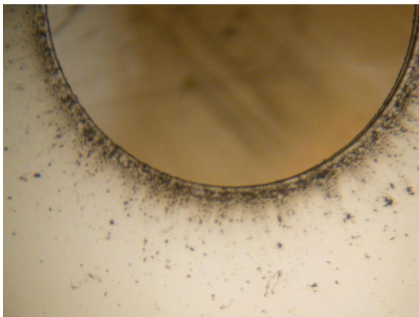
**Figure 17.12** This Figure contains a microscopic view of the external face of the alarm horn opening of the alarm pictured in Figures 17.10-17.11. There is a distinct pattern of enhanced soot deposition on this alarm that sounded during exposure to a flaming polyurethane source.
