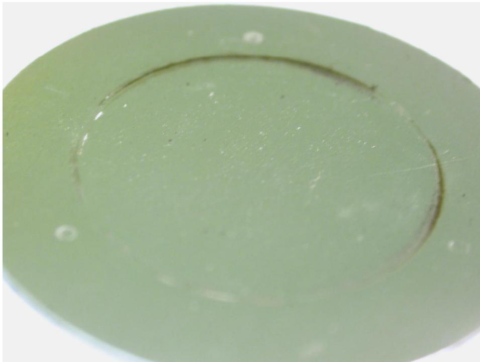
**Figure 14.7 Example of a ring marking on a smoke alarm horn disc exposed to a smoldering to flaming cabinet assembly fire.**
