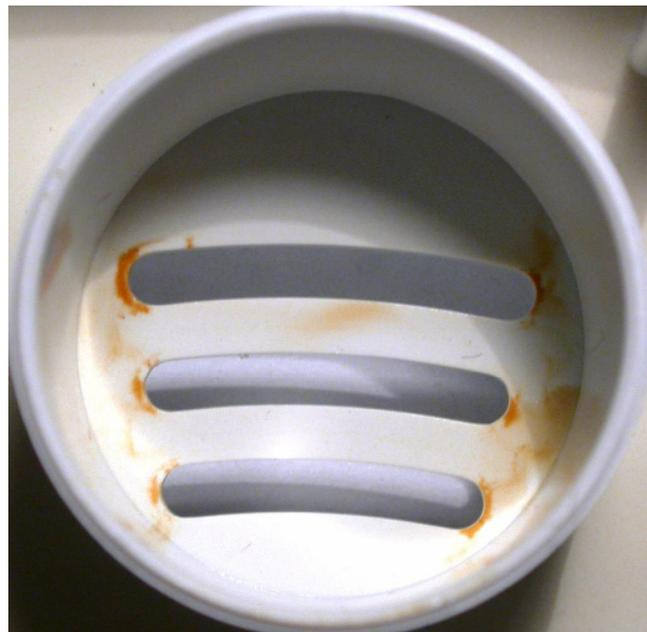
**Figure 16.14** This figure shows the internal face of the alarm pictured in Figure 16.13. This alarm sounded during exposure to a smoldering polyurethane source and has tarry enhanced soot deposition indicative of alarm sounding.
