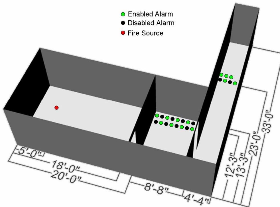
**Figure 4.5 Test Series 4 compartment layout**
