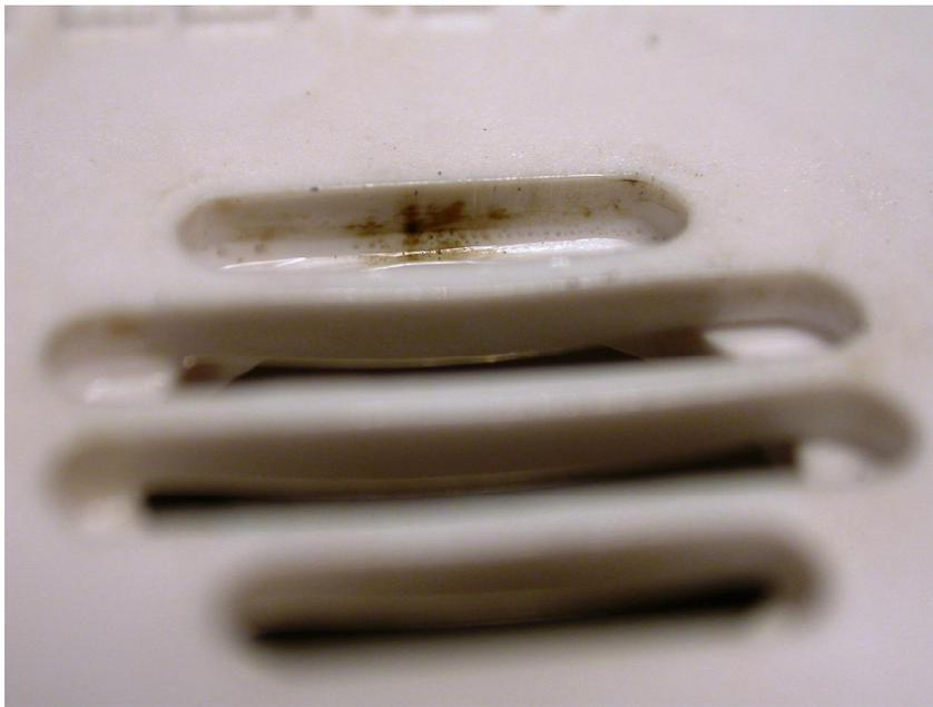
**Figure 22.18** This figure shows the vertical faces of the alarm from Figure 22.17. There are spots of enhanced depositions consistent with the fact that the alarm sounded.
