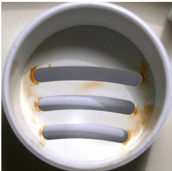
**Figure 7.20** This figure displays tarry enhanced deposition on the interior face of an FACI alarm exposed to a smoldering polyurethane fire. The orange enhanced deposition was only seen in alarms sounding. The yellow staining of the alarm cover outside the horn chamber was seen on all alarms exposed to smoldering polyurethane, regardless of sounding.
