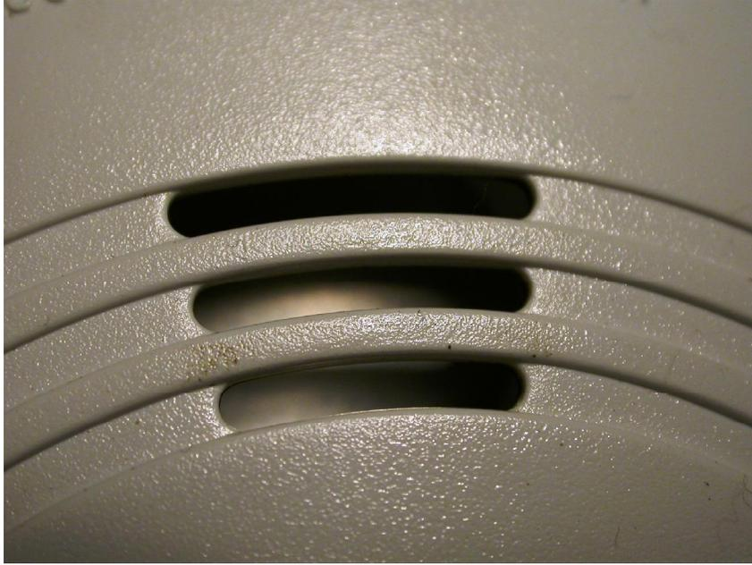
**Figure 22.9** This figure shows a macroscopic view of the horn openings from the alarm in Figure 22.8. This alarm sounded but shows only the slightest evidence of enhanced deposition.
