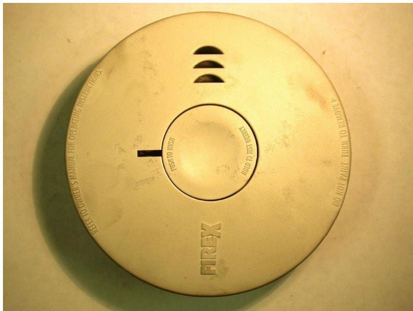
**Figure 17.7** This figure contains the external cover of an alarm that did not sound during exposure to a flaming polyurethane source.
