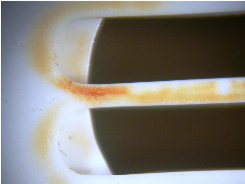
**Figure 16.3** This is a microscopic view of some of the alarm horn openings from the alarm in Figures 16.1-16.3. This alarm sounded during exposure to a smoldering polyurethane fire source. Tarry enhanced soot deposition is visible around the horn openings as orange/brown bands.
