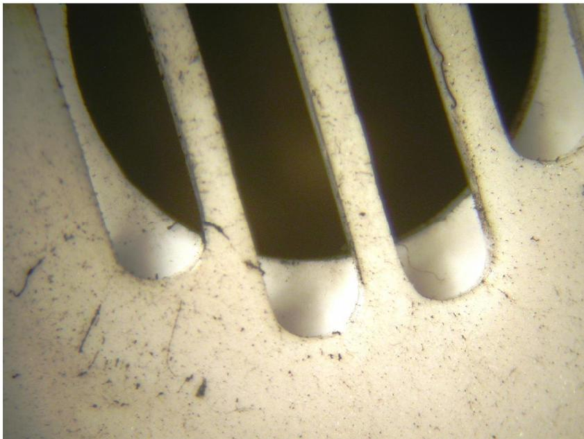
**Figure 23.24** This is a microscopic view of the horn openings of the alarm from Figure 23.23. The alarm did not sound and the soot deposition is commensurate with exposure to a high soot yield fire, but not enhanced deposition indicative of alarm.
