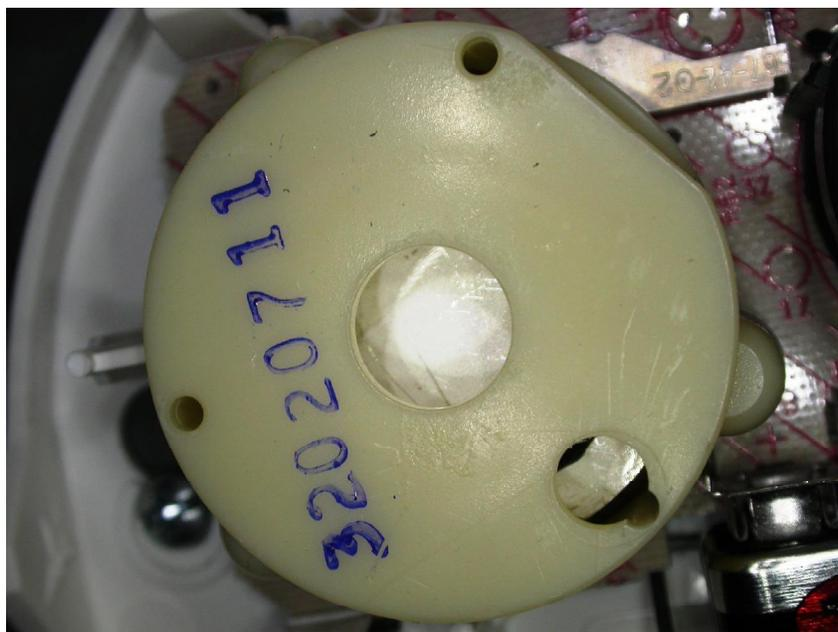
**Figure 19.6** This figure is a macroscopic view of the alarm horn openings of the alarm pictured in Figure 19.5. This alarm sounded during multiple nuisance exposures but does not show evidence of enhanced soot deposition.
