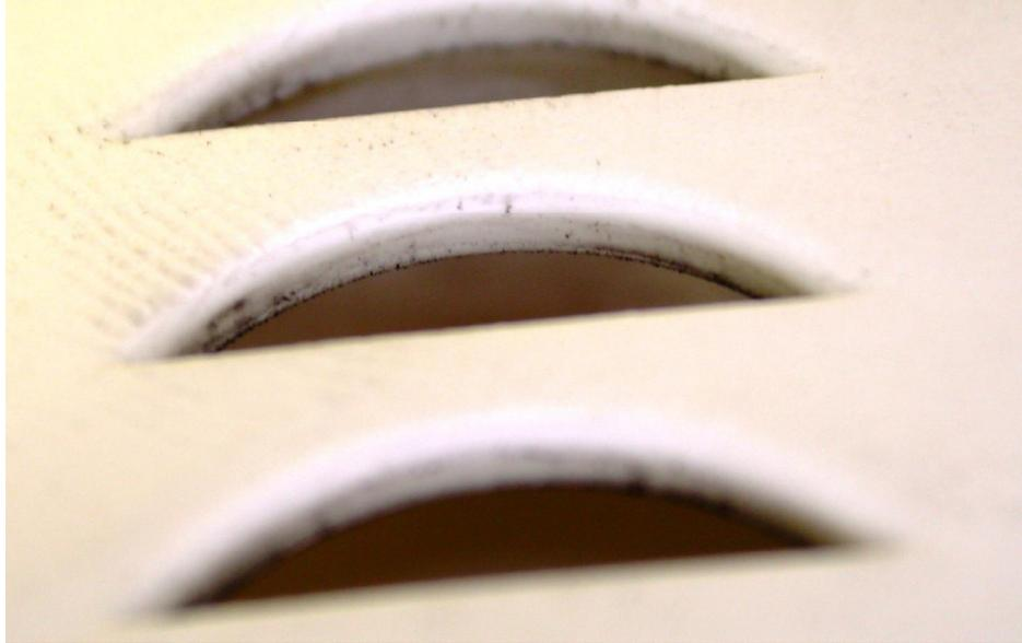
**Figure 13.7** A different view of the vertical faces of the smoke alarm horn openings. Deposition on the vertical face is darker than has been seen on the alarm cover or external face of the alarm horn openings. The deposition density moves from higher to lower density from the internal towards the external face. Combining the observations of Figures 13.2-13.7, it can be concluded that there is macroscopic, and therefore also microscopic enhanced soot deposition on the vertical face.
