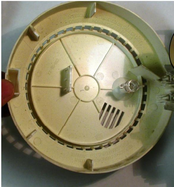
**Figure 16.6** This figure pictures the interior of the alarm cover of an FGBI alarm subjected to a smoldering polyurethane source. The alarm shows staining characteristic of an alarm subjected to a smoldering fire source.
