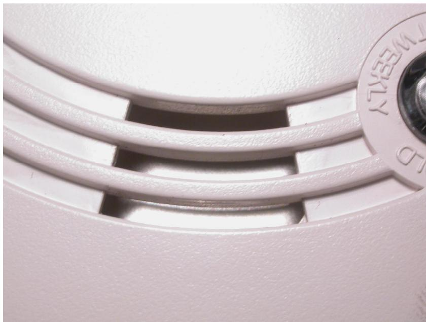
**Figure 17.32** This is a macroscopic view of the alarm horn from Figure 17.31. This alarm sounded during exposure to flaming polyurethane.
