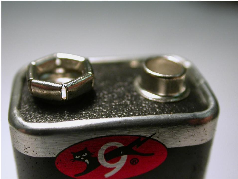
**Figure 14.5 Clean terminals on a properly installed battery from an FGBI alarm exposed to the flaming couch in Experiment 4.2. Compare the lack of deposition to soot deposited on the terminals of an improperly installed battery in Figure 14.4.**
