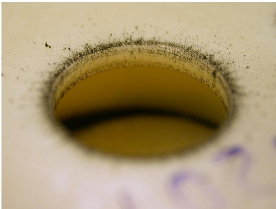
**Figure 7.30** Macroscopically observable enhanced soot deposition patterns on the vertical and external faces of an FGBI alarm horn opening that sounded during exposure to a flaming couch. Notice the bands of enhanced soot deposition on the vertical face of near each the internal and external faces of the horn opening.
