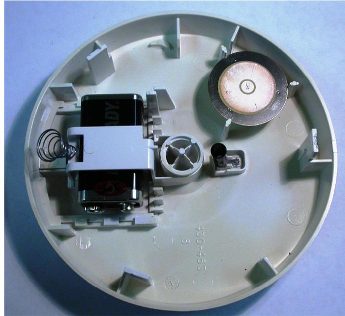
**Figure 16.13** This figure shows the interior of an alarm cover that sounded during exposure to a smoldering polyurethane fire source. There is staining characteristic of exposure to a smoldering polyurethane source.
