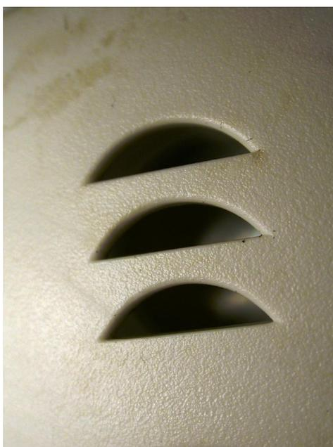
**Figure 22.2** This figure shows a macroscopic view of the horn openings from the alarm in Figure 22.1. This alarm sounded but shows only the slightest evidence of enhanced deposition at the corner of the upper right horn opening.
