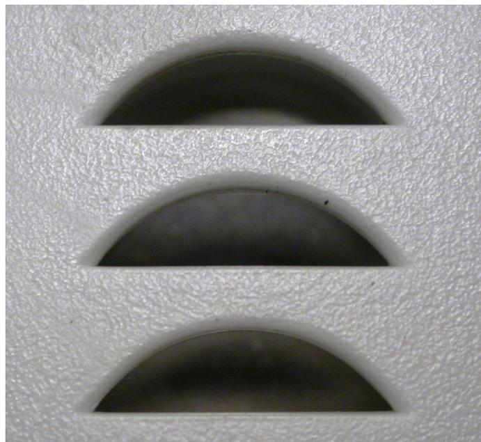
**Figure 18.6** This figure is a macroscopic view of the alarm horn openings of the alarm pictured in Figure 18.5. This alarm did not sound during the exposure.
