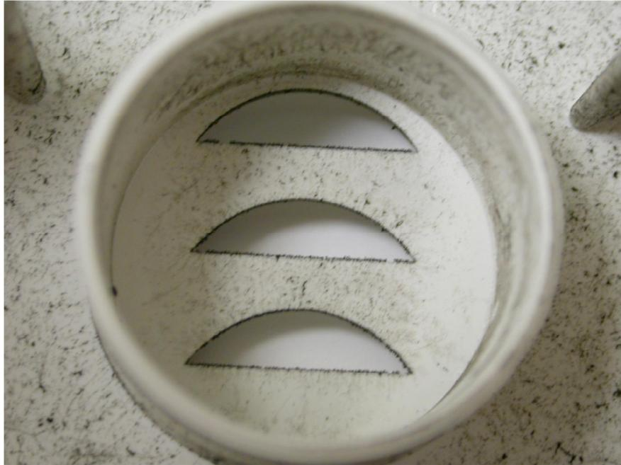
**Figure 7.24** This is the horn chamber of the alarm (shown in Figures 7.21-7.23) that did not sound. Notice the thin ring of soot around the horn openings, but the lower soot density in the horn chamber otherwise. Compare this to Figure 7.25.
