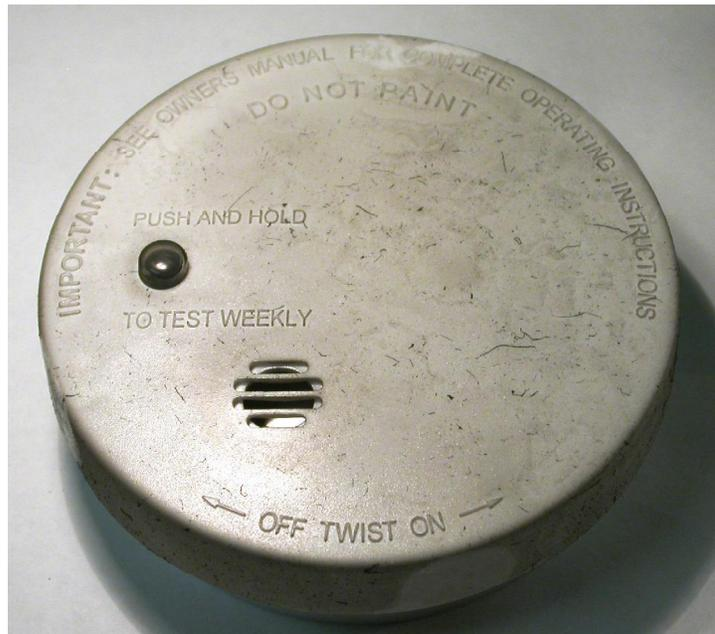
**Figure 23.22** This figure shows the cover of an FSBI alarm that did not sound during exposure to the flaming couch. The cover has soot deposited consistent with a high soot yield fire, but no signs of enhanced deposition.
