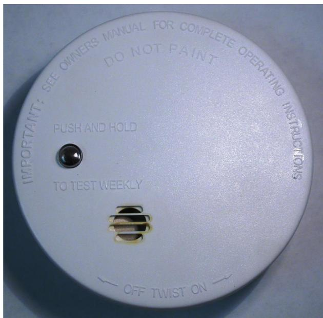
**Figure 16.1** This figure shows the exterior of the alarm cover of an alarm that sounded during exposure to a smoldering polyurethane source. Enhanced soot deposition patterns are visible in this figure around the alarm horn openings.
