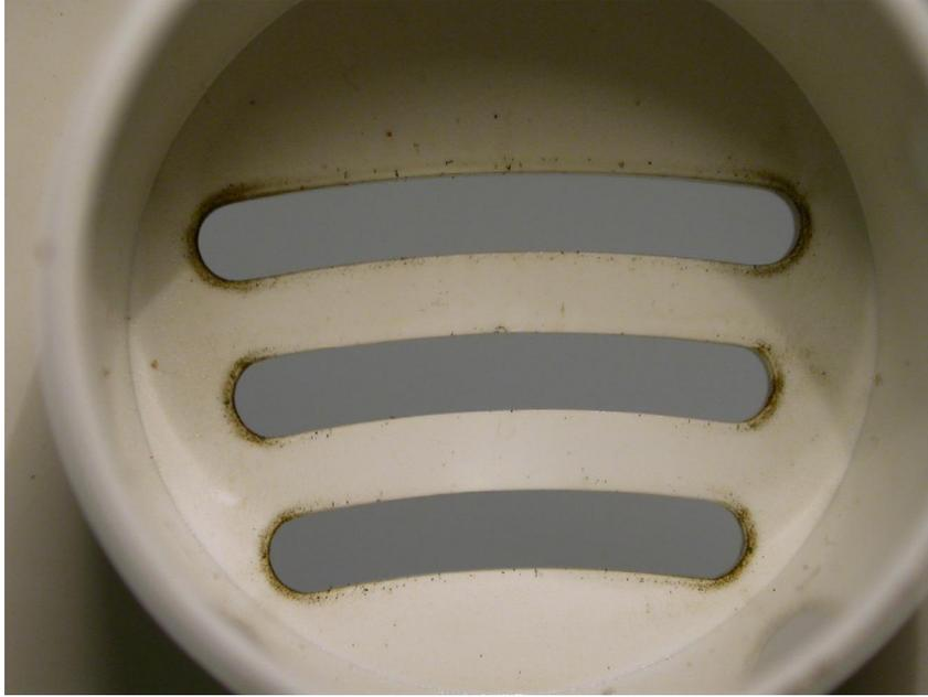
**Figure 22.11** This is a macroscopic view of the internal faces of the alarm horn openings from Figures 22.8-22.10. There is evidence of enhanced deposition around all three of the horn openings that was not apparent around the external faces.
