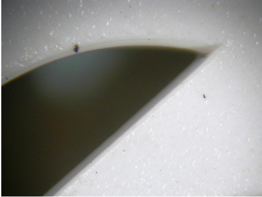
**Figure 18.7 This is a microscopic view of a horn opening pictured in Figure 18.6. This alarm did not sound and does not show evidence of enhanced soot deposition.**
