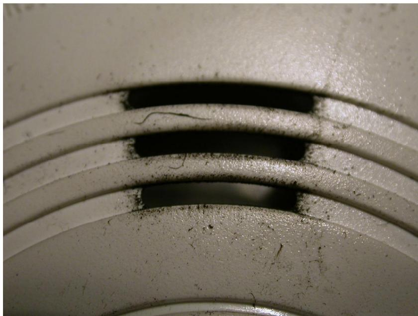
**Figure 23.8** This is a macroscopic view of the horn openings from the alarm in Figure 23.7. Enhanced deposition is apparent around portions of all of the horn openings.
