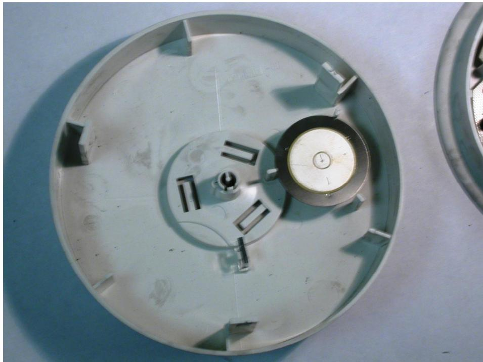
**Figure 0.20 Internal cover of a smoke alarm.**
