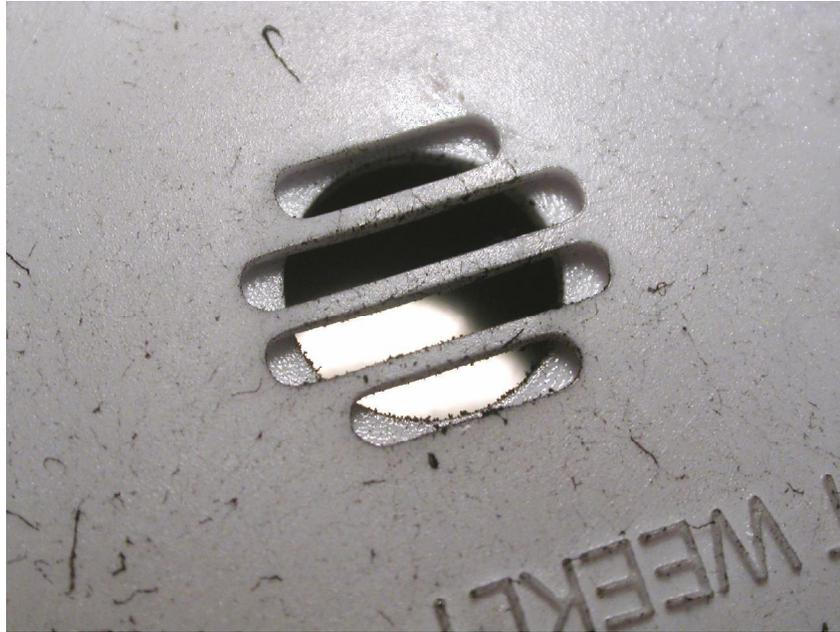
**Figure 21.25** This is a macroscopic view of the alarm horn openings from an FSBI alarm that did not sound during exposure to a flaming box filled with cups. There is soot deposited around the horn openings of the same size and density as that deposited away from the horn openings.
