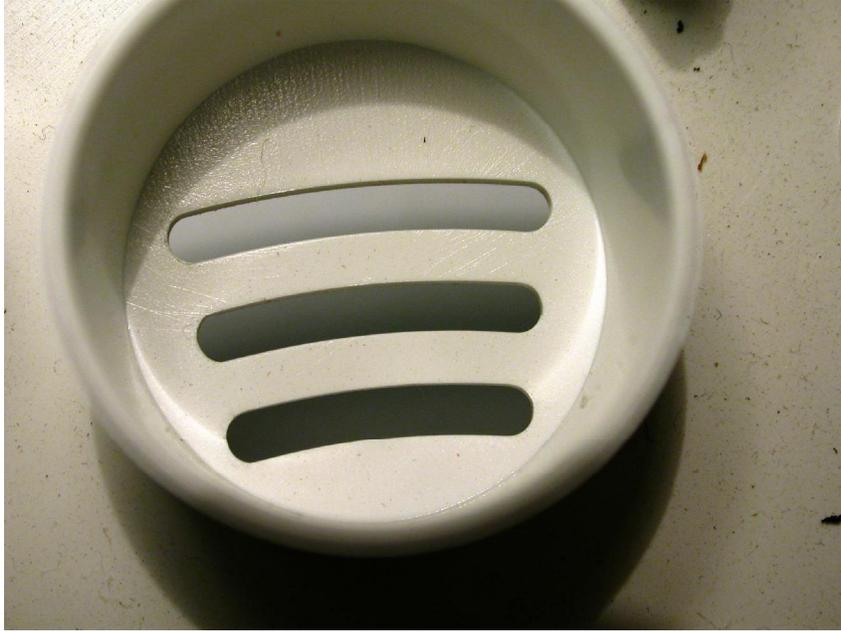
**Figure 22.15 This is a macroscopic view of the internal faces of the alarm horn openings from Figures 22.12-22.14. There is no evidence of enhanced deposition consistent with the fact that the alarm did not sound.**
