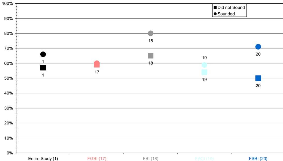
**Figure 8.8** This figure contains a summary of the percentage of alarms identified by the technique, during the blind study for the entire study and the populations of horn configuration. This figure contains the percentage results based on the number of alarms that sounded, 83, 20, 20, 17, and 21 respectively, and the number of alarms that remained silent in each population, 68, 17, 20, 13, and 18 respectively.
