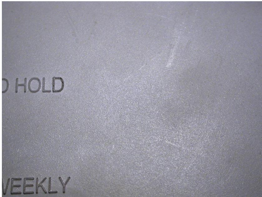
**Figure 17.29** This figure shows the ambient soot deposited on the external cover of the alarm pictured in Figures 17.27-17.28.
