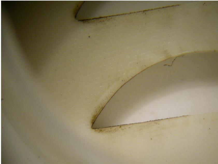
**Figure 22.4 This is a microscopic view of one of the alarm horn openings from Figure 22.3. There is evidence of enhanced deposition consistent with the tarry deposition indicative of alarm sounding.**
