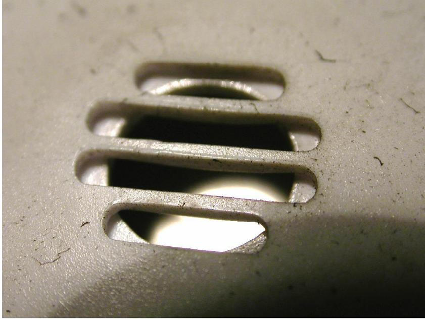
**Figure 23.23** This is a macroscopic view of the horn openings of the alarm from Figure 23.22. This alarm did not sound and does not have enhanced deposition.
