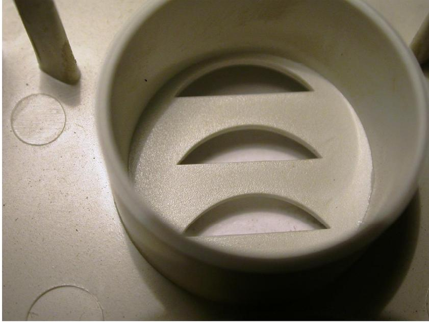
**Figure 22.7** This figure shows a macroscopic view of the internal face of the alarm horn openings from Figures 22.5 and 22.6. There is no evidence of enhanced deposition consistent with the fact that the alarm did not sound.
