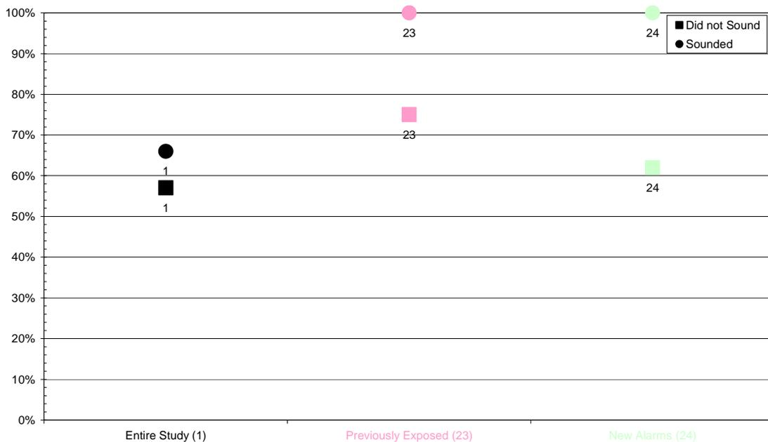
**Figure 8.10 Summary of results of the blind study for the entire study and the populations separated by exposure history. This figure contains the percentage results based on the number of alarms that sounded, 83, 7 and 8 respectively, and the number of alarms that remained silent, 68, 8, and 8 respectively, in each population.**
