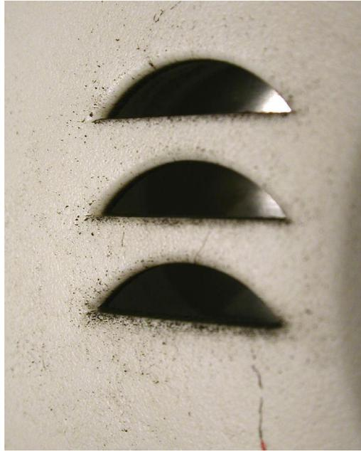
**Figure 23.1 Macroscopic view of the external face of the alarm horn openings of an alarm that sounded during exposure to a flaming couch. Enhanced soot deposition is apparent on the flat edges of the moon-shapes.**
