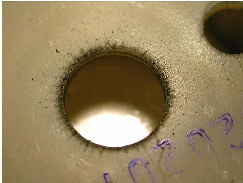
**Figure 23.14** This figure is a macroscopic view of the horn opening of the alarm pictured in Figure 23.13. The horn opening has enhanced soot depositions encircling the opening as evidence of the alarm sounding.
