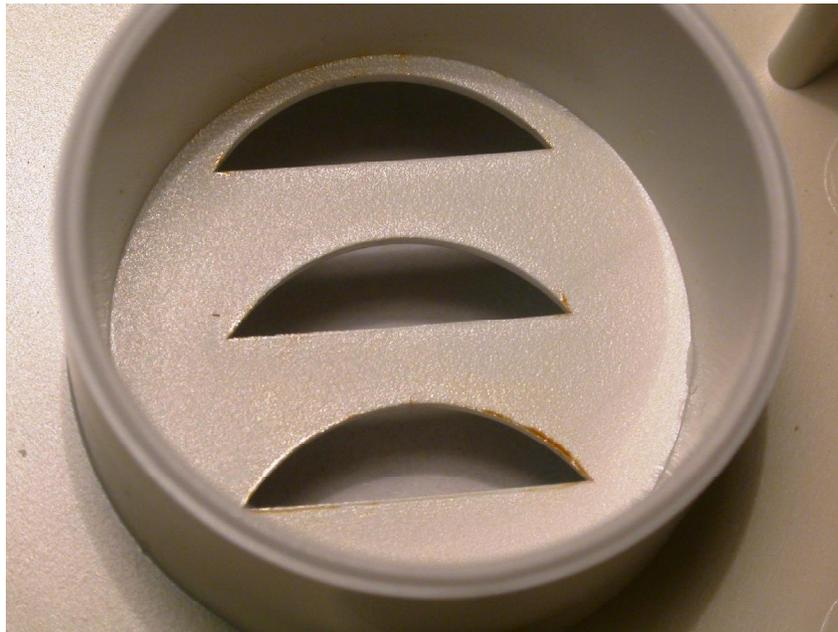
**Figure 16.10** This figure shows a macroscopic view of the internal face of smoke alarm horn openings of an alarm that sounded during exposure to a smoldering polyurethane source. There is evidence of tarry enhanced soot deposition indicative of alarm sounding around the edges of the horn openings.
