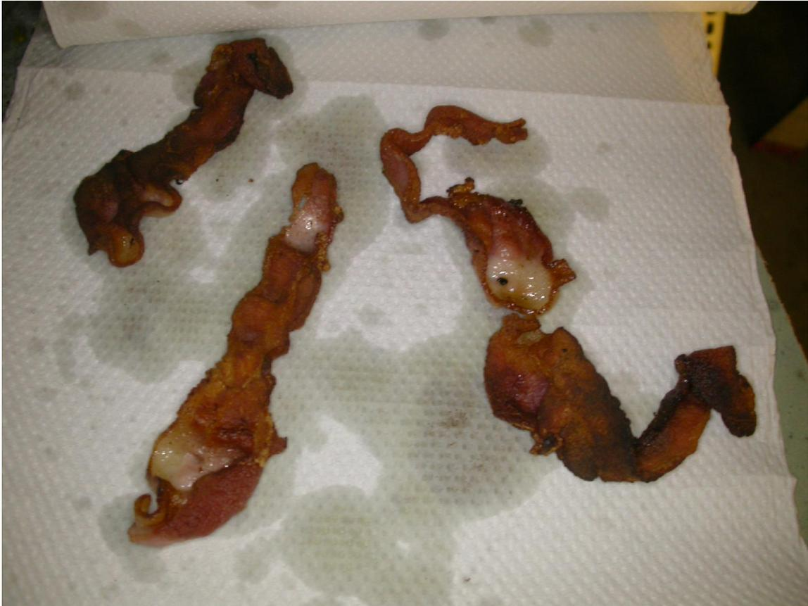
**Figure 6.7 Typical end product of the frying bacon nuisance exposure tests in Test Series 2.**
