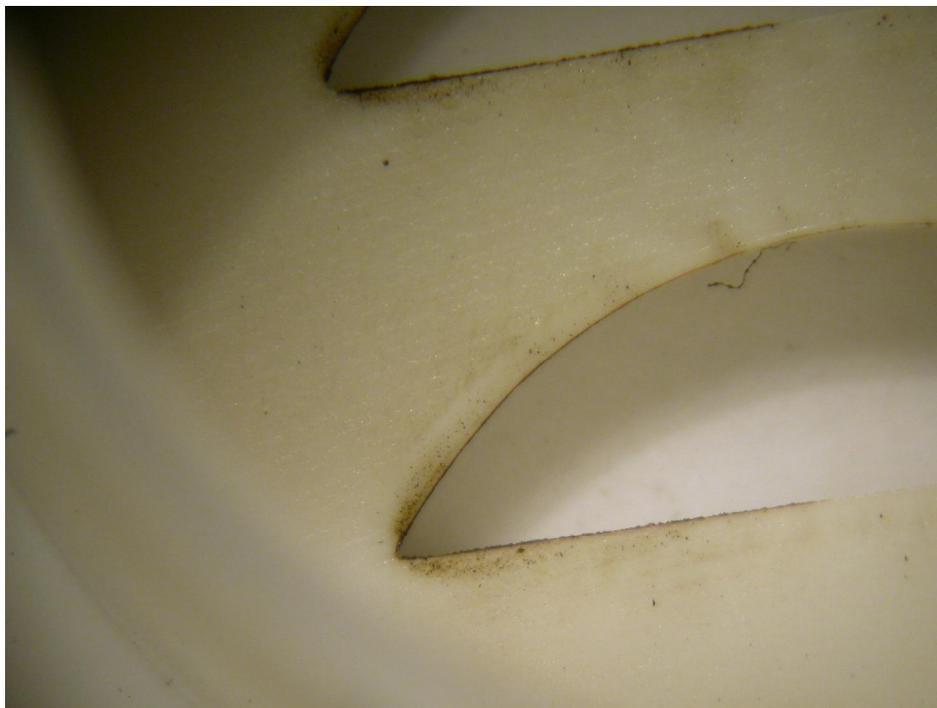
**Figure 7.29** An example of microscopically observable enhanced deposition on the internal face of an FBI horn opening that sounded from a smoldering/flaming cabinet assembly fire.
