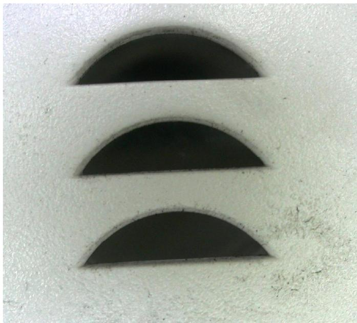
**Figure 17.8** This figure contains a macroscopic view of the external face of the alarm horn openings of the same alarm as in Figure 17.7. There is some visible deposition around the alarm horn openings but it is not of any greater density than the deposition on the cover of the alarm further from openings.
