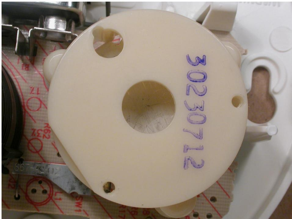
**Figure 0.10 Exterior of FGBI Smoke Alarm Horn Opening.**
