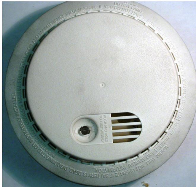
**Figure 17.14** This figure shows the exterior alarm cover of an FGBI alarm that did not sound during exposure to a flaming polyurethane fire.
