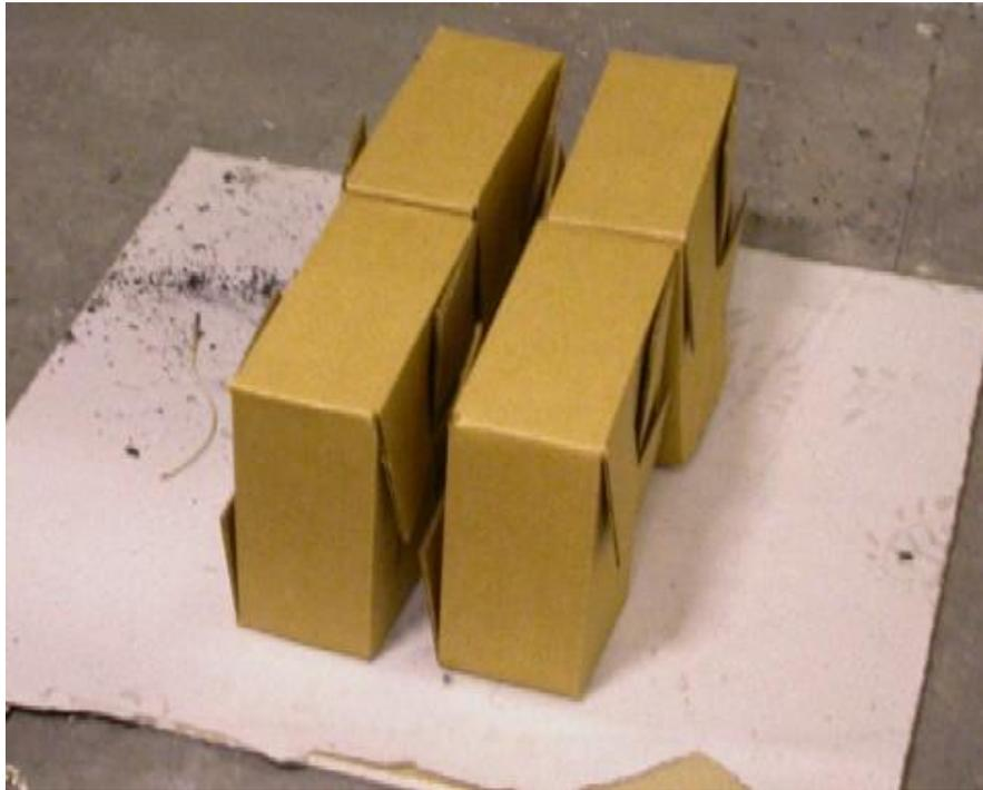
**Figure 6.13 Arrangement of boxes for the boxes filled with paper experiment in Test Series 3. The boxes were ignited with a butane lighter in the central flue space.**
