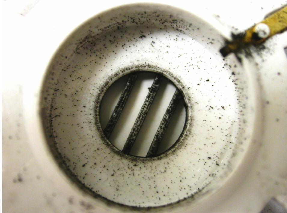
**Figure 0.13 Interior of FSBI Smoke Alarm Horn Opening.**
