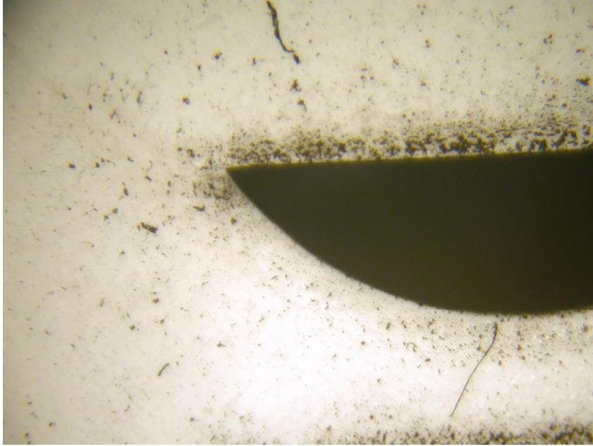
**Figure 23.3** This is a microscopic view of the corner of the alarm horn opening from Figure 23.2. The enhanced soot deposition is distinctly apparent in this view.
