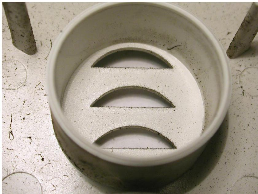
**Figure 23.6 This is a macroscopic view of the interior face of the horn openings of the alarm from Figure 23.5. This alarm did not sound and there is no enhanced soot deposition indicative of sounding. Although there is some soot deposition on the edges the soot deposition density inside the horn chamber is less dense than that deposited outside the horn chamber.**
