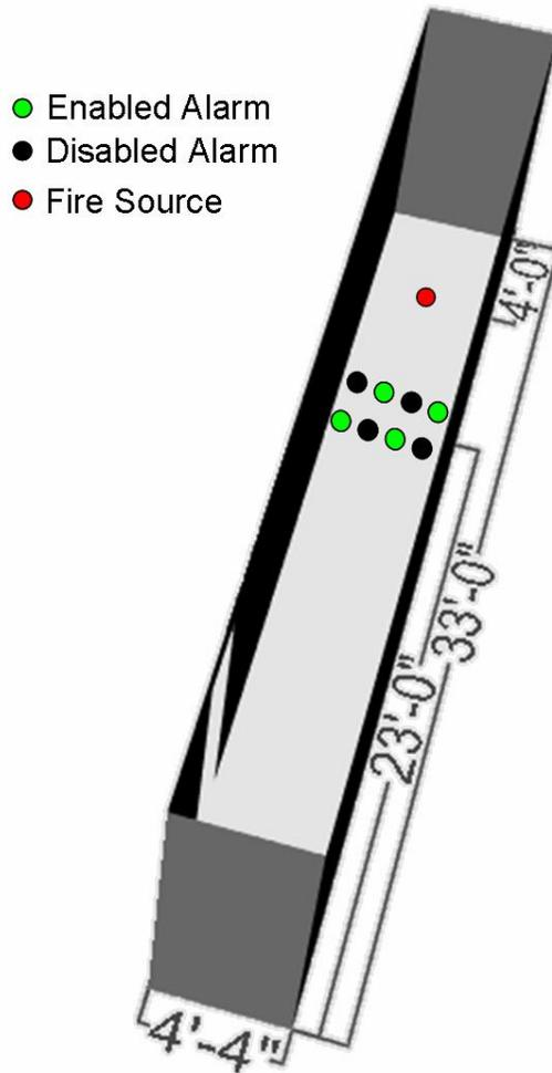
**Figure 4.4 Test Series 3 compartment layout.**
