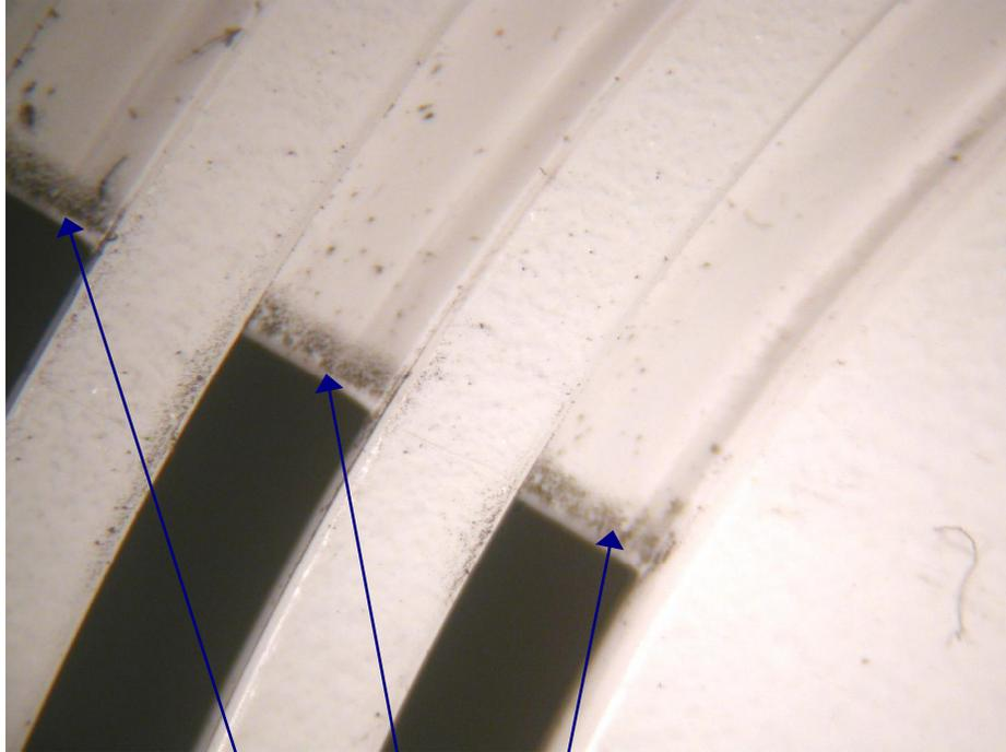
**Figure 7.12 Enhanced soot deposition on the external face of a PHOTO horn opening occurring in an alarm sounding during exposure to a flaming polyurethane fire. The enhanced deposition is concentrated on the side edges of the horn opening.**
