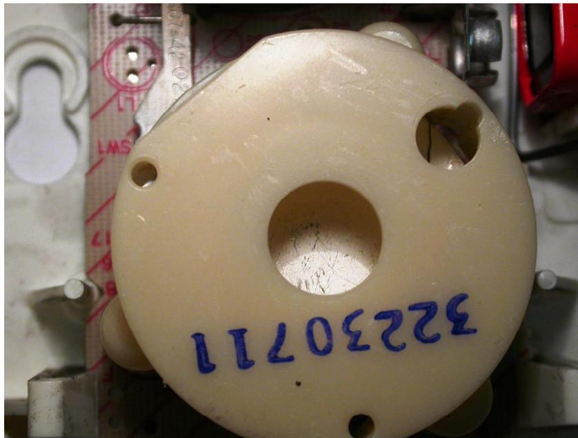
**Figure 17.16** This is a macroscopic view of the horn of the alarm pictured in figures 17.14-17.15. This alarm did not sound during exposure to a flaming polyurethane source and shows no signs of enhanced soot deposition.
