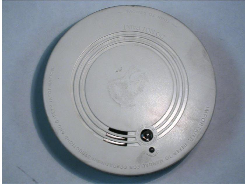
**Figure 17.31** This is the exterior cover of a Photo alarm that sounded during exposure to a flaming polyurethane fire.
