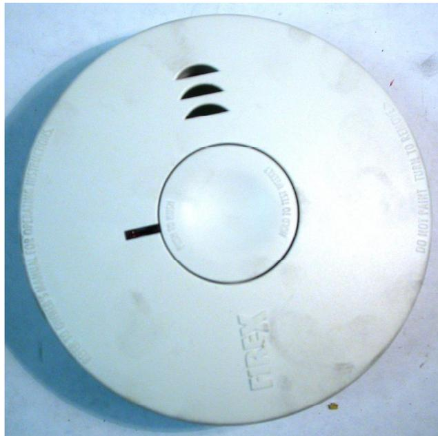
**Figure 18.5** This figure shows the exterior cover of an FBI alarm that did not sound during exposure to a flaming wood fire.
