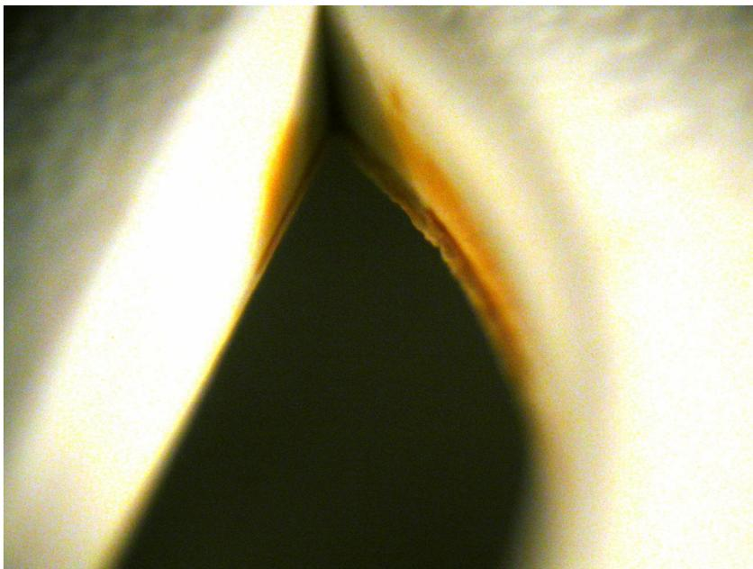
**Figure 16.11** This figure shows a microscopic view of the vertical face of one of the alarm horn openings of the alarm pictured in Figures 16.9-16.10. This alarm sounded during the exposure and tarry enhanced soot deposition is visible as the yellow orange depositions in the corner of the opening.
