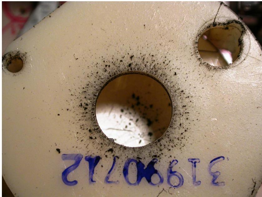
**Figure 21.17** This is a macroscopic view of the horn opening of the alarm pictured in Figures 21.15 and 21.16. Evidence of enhanced soot deposition indicates that the alarm sounded during the exposure.
