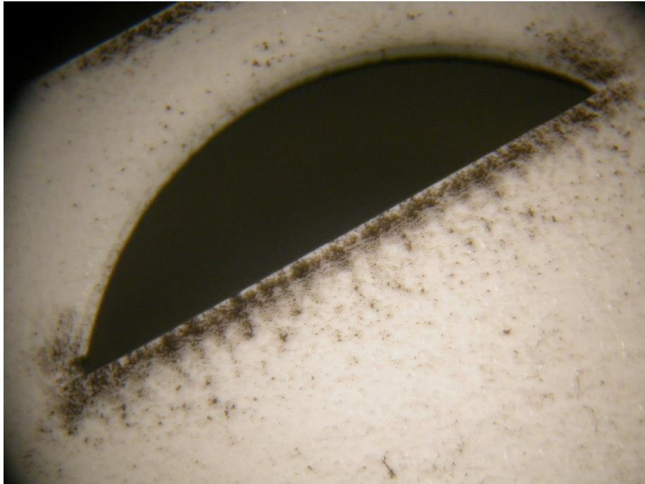
**Figure 7.11 An example of enhanced soot deposition pattern on the external face of an FBI horn opening in an alarm that sounding during exposure to a flaming polyurethane test fire. The enhanced deposition is especially concentrated on the corners and flat portions of the moon-shaped openings and not around the entire opening.**
