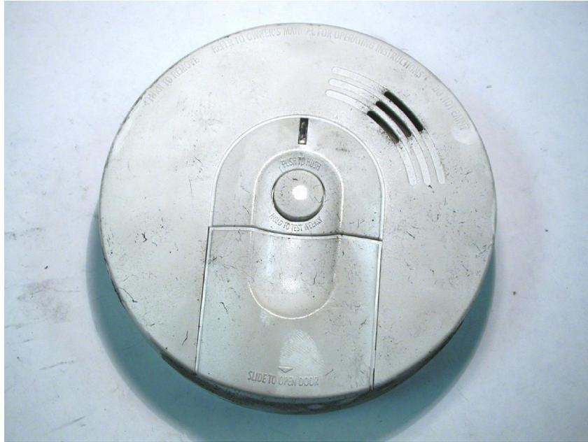
**Figure 21.9** This figure shows the exterior of the alarm cover of an FACP alarm that sounded during exposure to a flaming box with cups fire.
