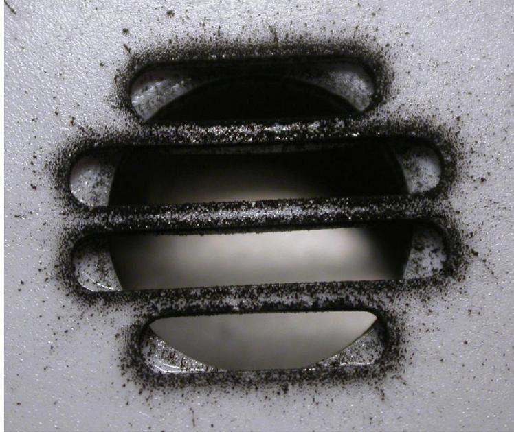
**Figure 17.25** This is a macroscopic view of the alarm horn opening seen from afar in Figure 17.24. The FSBI alarm sounded during exposure to a flaming polyurethane fire and displays evidence of enhanced soot deposition.
