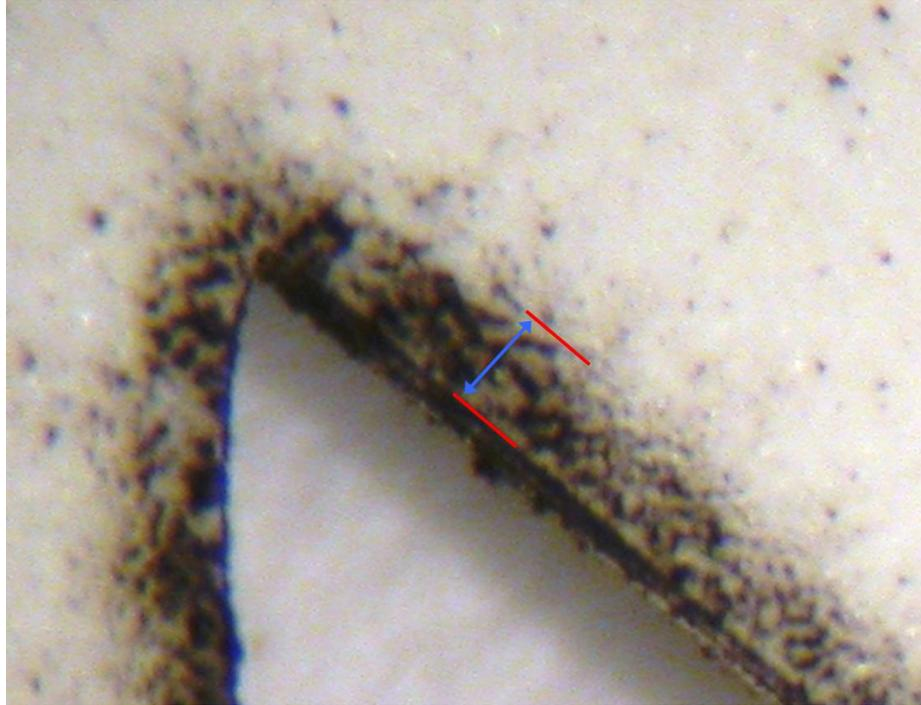
**Figure 7.14 An example of the measurement of the radial width of an enhanced soot deposition on the internal face resulting from a flaming polyurethane exposure. The radial width is conservatively measured to the extent of soot agglomerates obviously larger than the ambient agglomerate size. The radial width, measured perpendicular to the horn opening edge, or radially, between the two red lines is 0.433 mm.**
