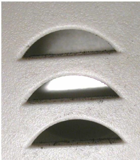
**Figure 21.7 This is a macroscopic view of the horn openings from the alarm pictured in Figure 21.6. This alarm did not sound during the exposure but there is ambient soot deposition on the vertical face of the alarm.**
