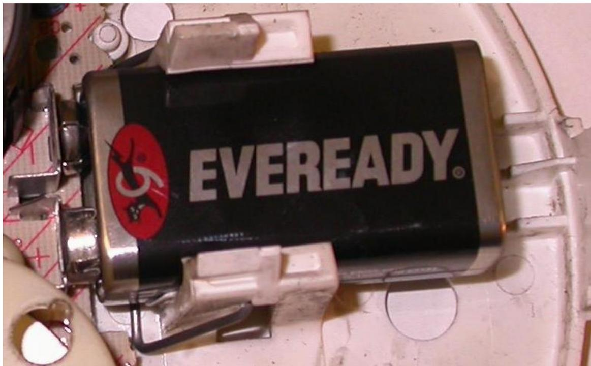
**Figure 14.2 An FGBI alarm with a properly installed battery. The arms that hold the battery in place form a tight seal to the battery and during some higher soot yield exposures yield the patterns seen in Figure 14.3. The alarm battery terminals also fit tightly around the battery terminals allowing for evaluation of soot or lack thereof on both terminal sets.**
