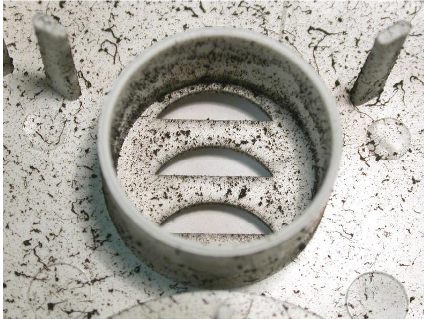
**Figure 21.5** This figure shows the interior face of the alarm horn opening pictured in Figures 21.1-21.4. There is evidence of enhanced soot deposition around the alarm horn openings, as the alarm sounded. Also of note is the soot deposited within the horn chamber is of equal or greater density than that outside the horn chamber.
