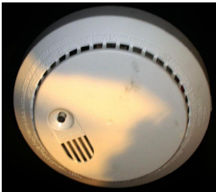
**Figure 20.5** This figure shows the cover of an FGBI alarm that sounded during exposure to a smoldering cable fire.
