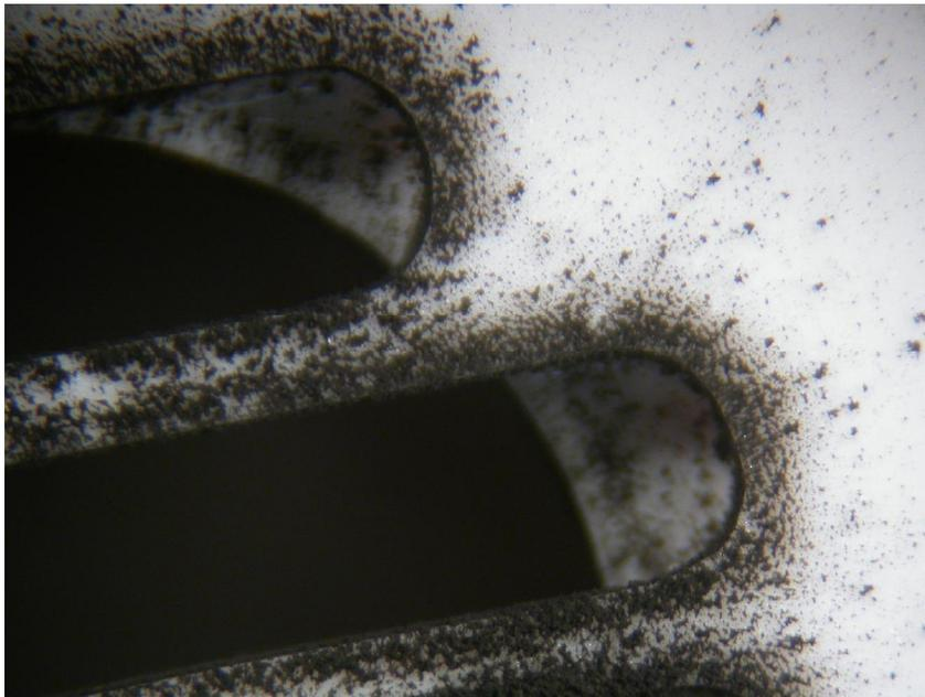
**Figure 17.26** This is a microscopic view of the pattern of enhanced soot deposition seen in Figure 17.25. This alarm sounded during exposure to a flaming polyurethane source.
