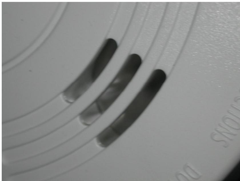
**Figure 20.4** This is a macroscopic view of the alarm horn openings from the alarm pictured in Figure 20.3. This alarm sounded but does not show any evidence of enhanced soot deposition.
