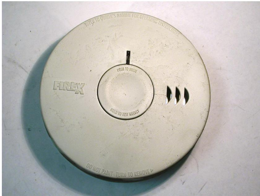
**Figure 23.5 This is the external cover of an FBI alarm that did not sound during exposure to the flaming couch.**
