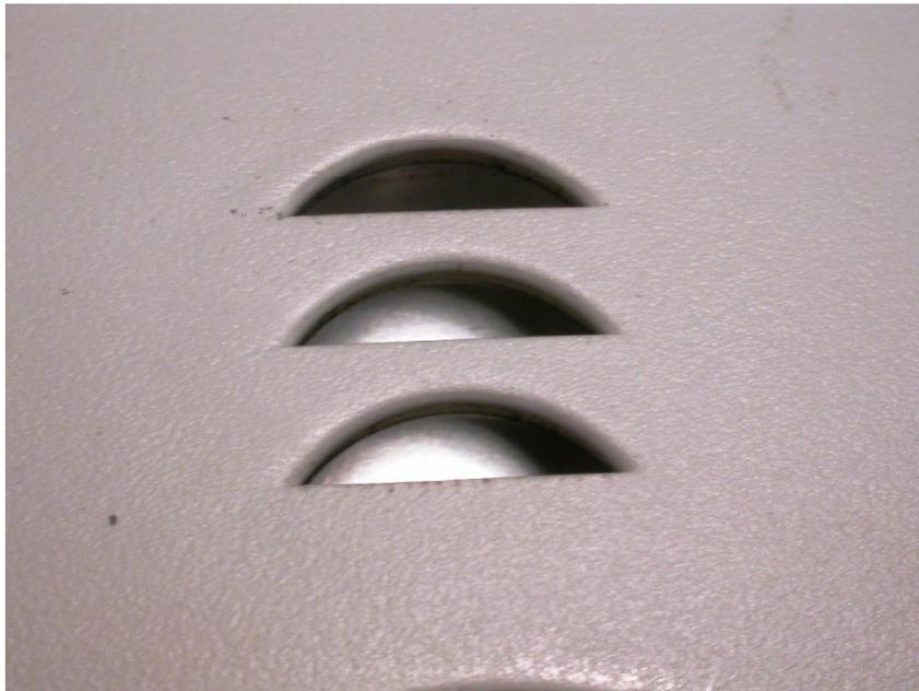
**Figure 13.2** This figure shows the next step in documenting the alarm state. It contains a macroscopic view of the alarm horn openings. There is very little soot apparent at this magnification. There appear to be slight indications of possible enhanced soot deposition on the flat edge of the lowest opening. There is not enough soot to make a conclusive determination of sounding.
