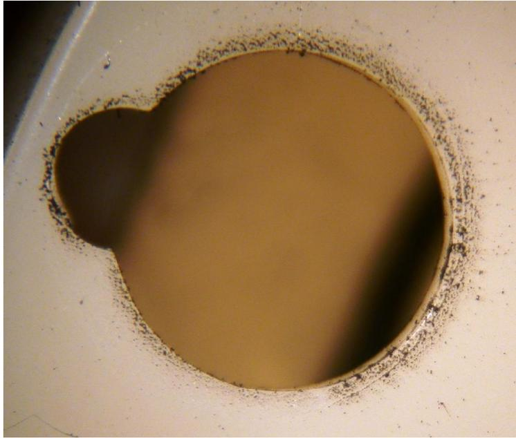
**Figure 17.13** This is a macroscopic view of the secondary hole on the horn of the same FGBI alarm pictured in Figures 17.10-17.13. There are obvious patterns of enhanced soot deposition indicating that this alarm sounded during exposure to the flaming polyurethane source.
