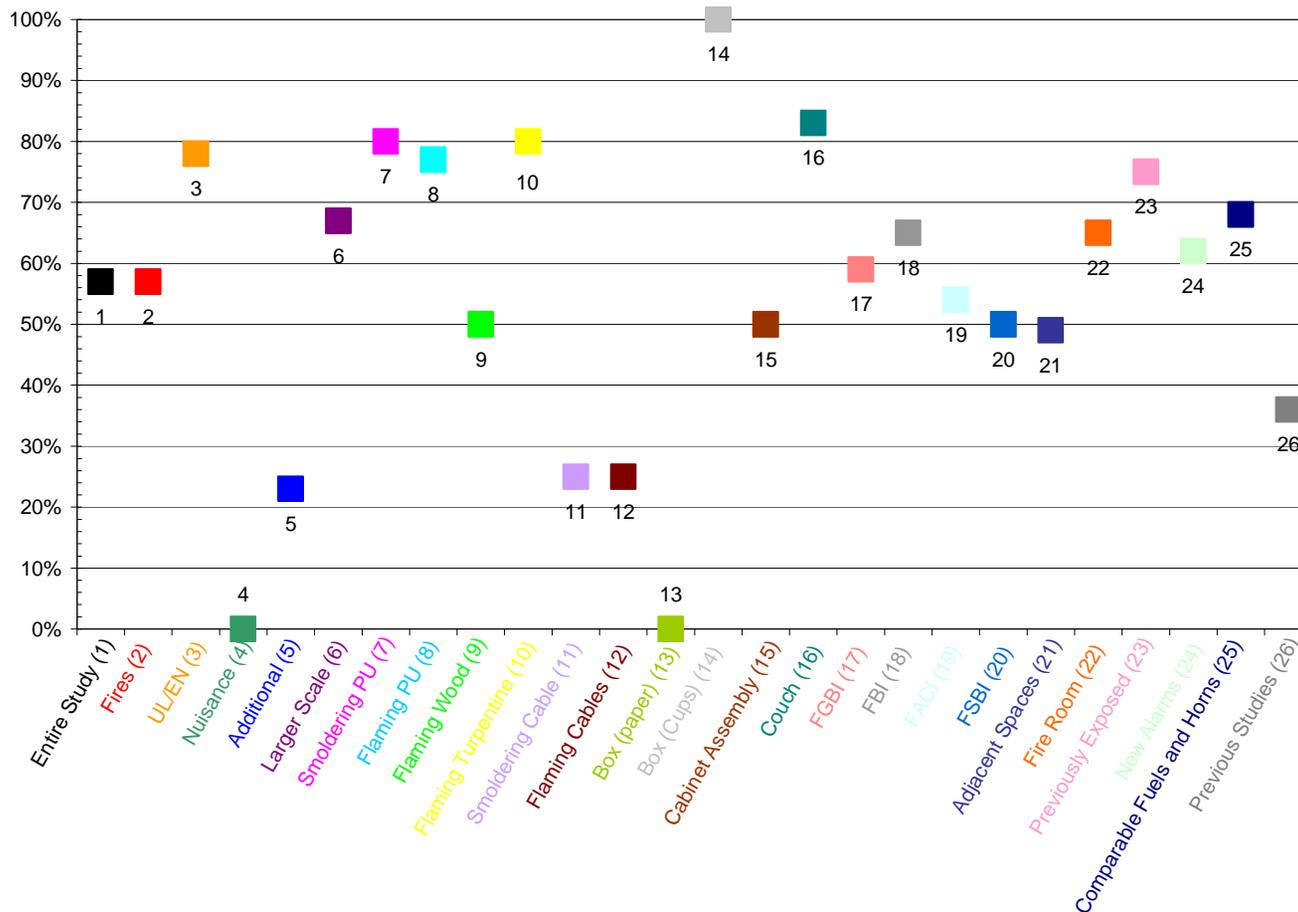
**Figure 8.4 This figure summarizes the results of the application of the negative identification heuristic to the blind study observations by population. This figure contains the percentage of alarms identified as not having sounded per the number of alarms that actually had not sounded in the specified population. There were no false determinations of not having sounded for any of the populations in this study.**
