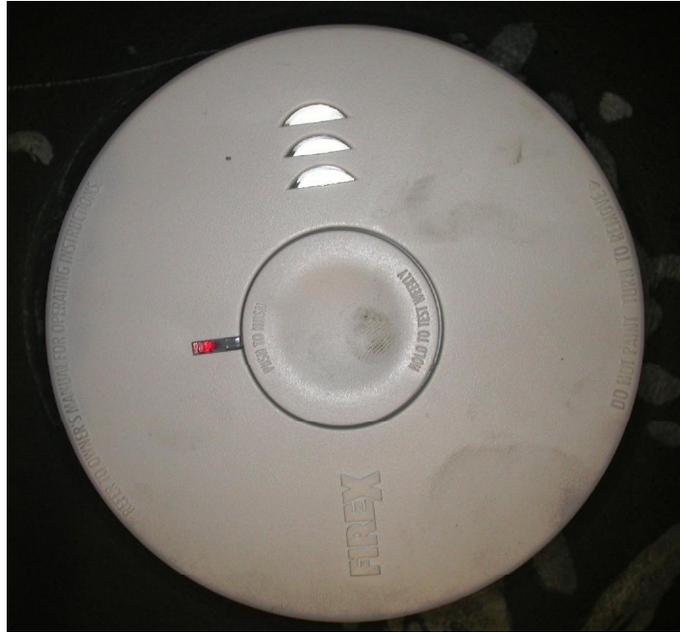
**Figure 20.1** This figure shows the cover of an FBI alarm that sounded during exposure to a smoldering cable fire.
