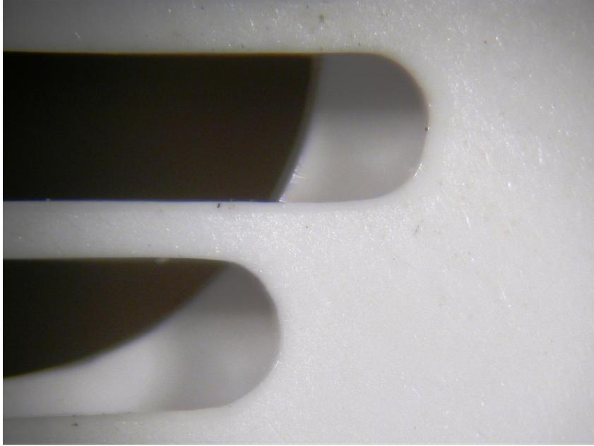
**Figure 18.15 This is a microscopic view of the alarm horn opening of the alarm pictured in Figure 18.14. This alarm sounded during exposure to a flaming wood fire but does not show evidence of enhanced soot deposition.**
