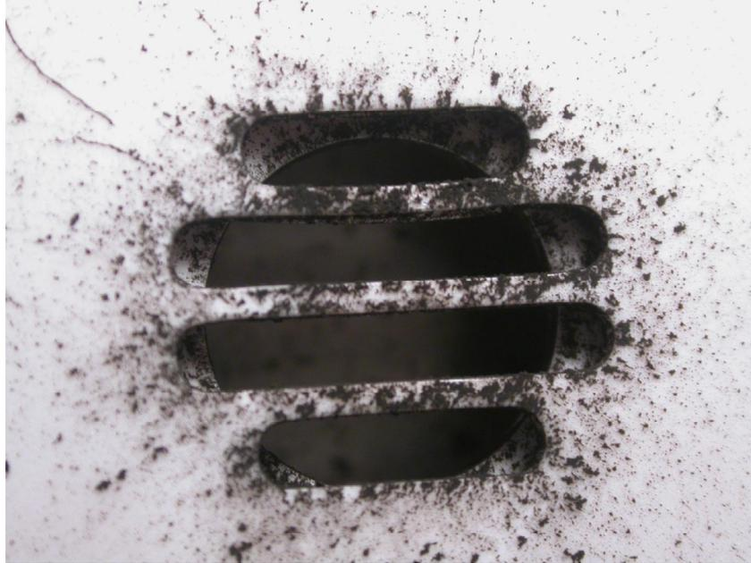
**Figure 21.23** This figure shows a macroscopic view of an alarm horn opening of an FSBI alarm that sounded during exposure to a flaming box filled with cups. There is evidence of enhanced soot deposition with higher density and larger soot agglomerates around the openings.
