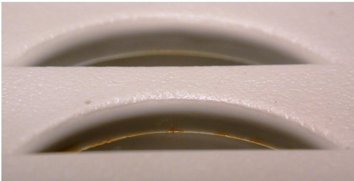
**Figure 16.12** This is a macroscopic view of 2 of the vertical faces of the alarm horn openings of the alarm pictured in Figures 16.9-16.12. Enhanced tarry soot deposition visible on both vertical faces but most obvious on the closer vertical face.
