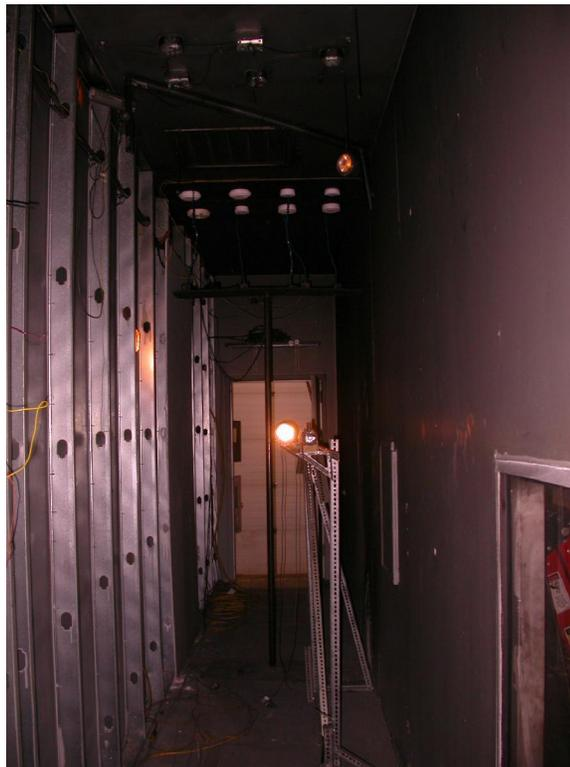
**Figure 6.11** The bank of smoke alarms typical of the arrangement of alarms in the hallway for Test Series 3. The bank consisted of eight new alarms, one pair of enabled and disabled alarms each of new FBI, FGBI, FSBI, and FACI alarms.
