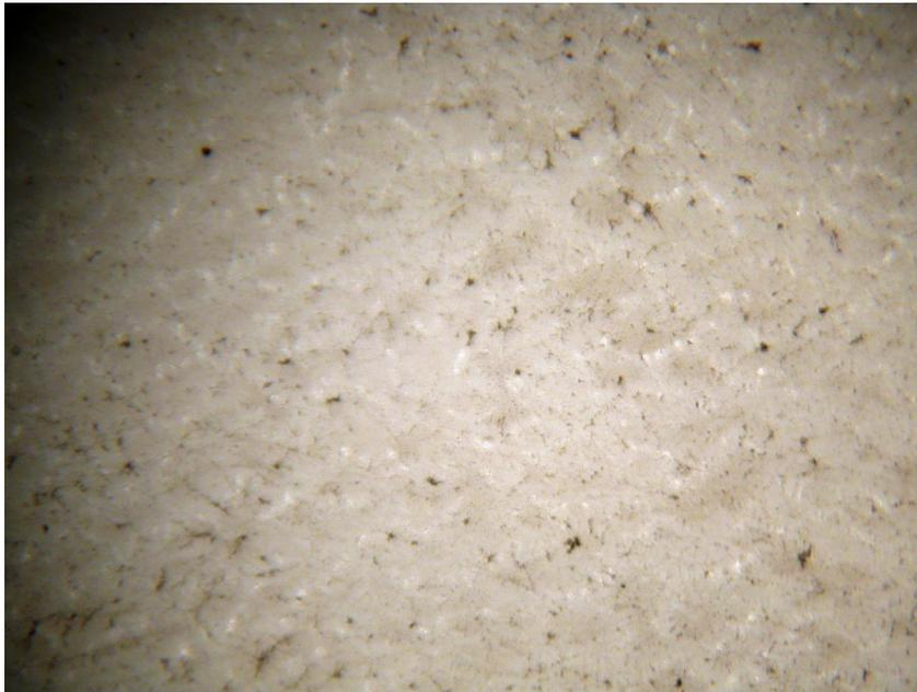
**Figure 21.4 This figure shows the ambient soot deposition on the exterior of the alarm cover taken at the same magnification as Figure 21.3. The deposition density and agglomerate size are much lower than those in the pattern of enhanced soot deposition.**
