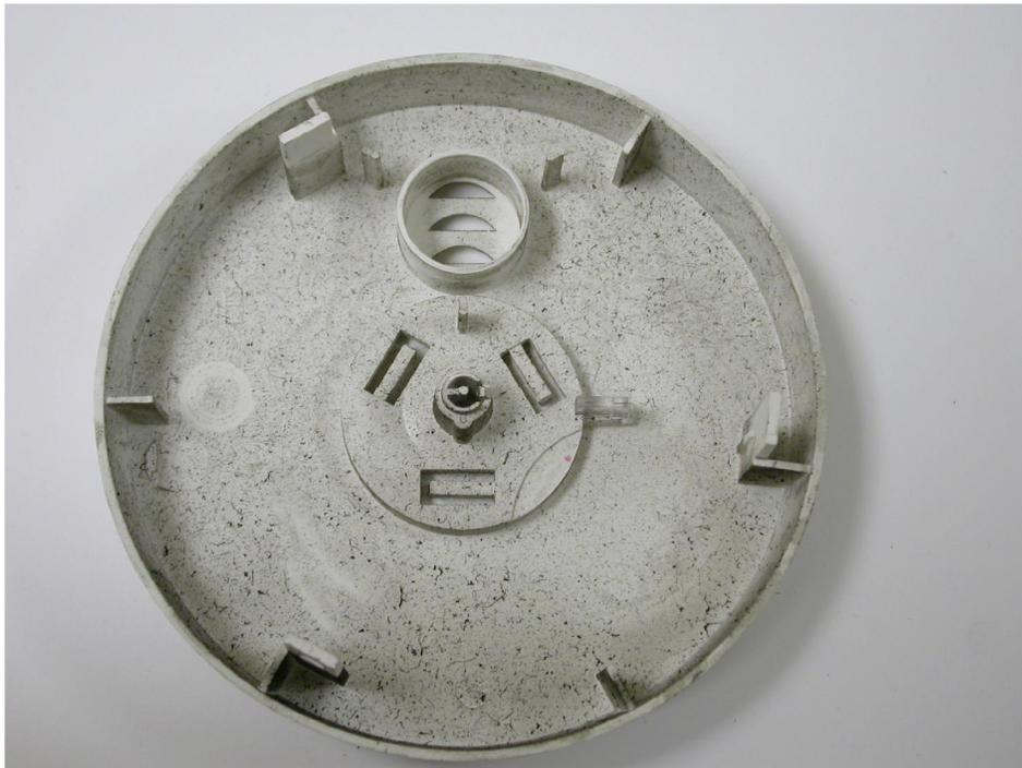
**Figure 7.23** This is the internal cover of the alarm in Figures 7.19 and 7.22 that did not sound. Notice the difference in soot deposition density inside and outside the smoke alarm horn chamber.
