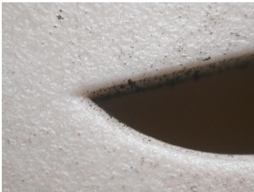
**Figure 21.8 This is a microscopic view of one of the alarm horn openings from Figure 21.7. This alarm did not sound and there is soot deposited around the horn opening, but no evidence of enhanced soot deposition.**
