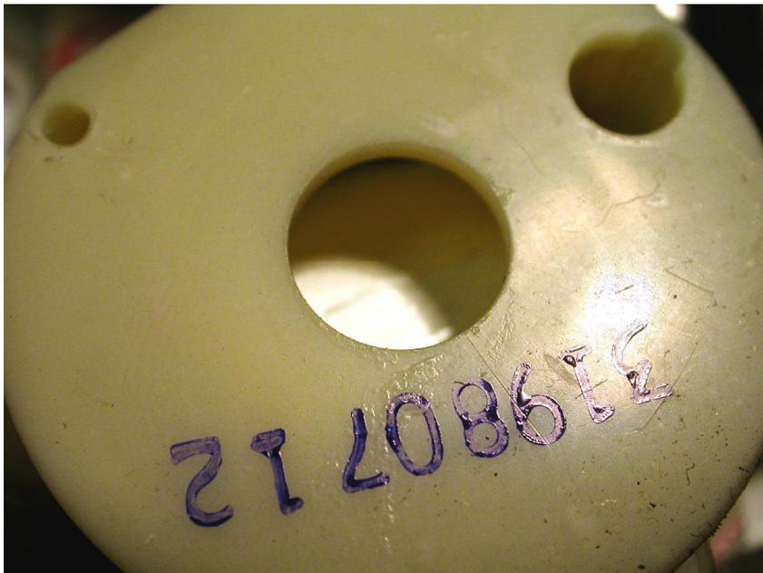
**Figure 23.18** This is a macroscopic view of the alarm horn opening of the alarm in Figure 23.17. There is no enhanced deposition visible on this horn, consistent with it not sounding.
