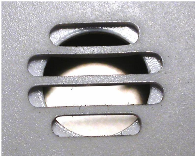
**Figure 17.28** This is a macroscopic view of the external face of the alarm horn opening from the alarm pictured in Figure 17.27. This alarm does not display evidence of enhanced soot deposition, as it did not alarm.
