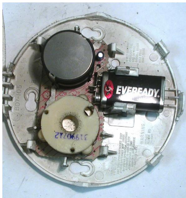
**Figure 21.16** This figure shows the interior of the alarm pictured in Figure 20.15. Enhanced soot deposition around the horn opening is visible in this view.
