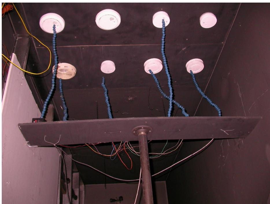
**Figure 6.18** The bank of alarms in the hallway for Test Series 4. The bank consists of 2 pairs of new alarms enabled and disabled, two used alarms enabled, and two enabled photo alarms.
