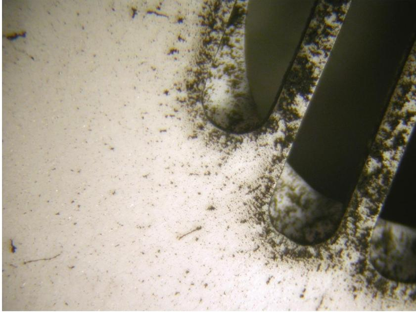
**Figure 23.21** This is a microscopic view of the horn openings from Figure 23.20. The enhanced soot deposition, indicative of alarm sounding, is evident from the higher density and larger agglomerates proximate to the horn openings.
