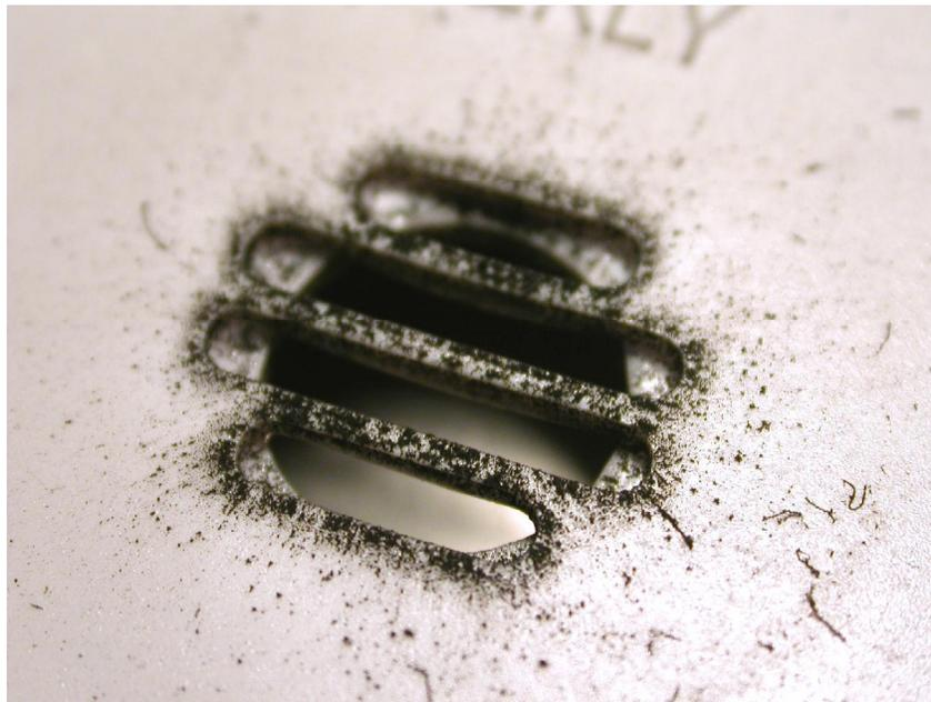
**Figure 23.20** This is a macroscopic view of the horn openings of the alarm in Figure 23.19. The alarm sounded during the fire exposure which is indicated through the enhanced soot deposition around the horn openings.
