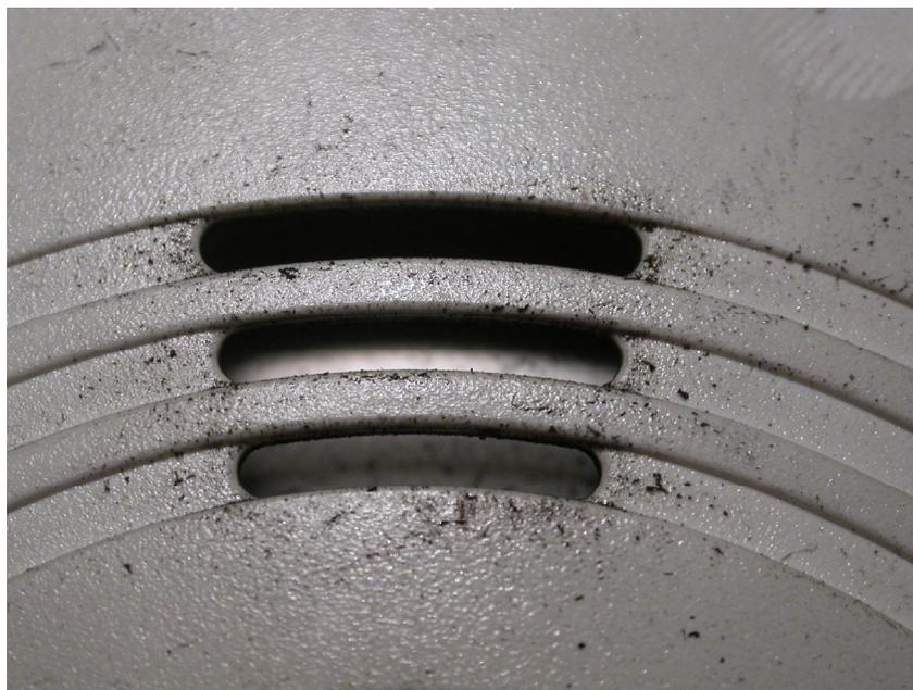
**Figure 21.10** This is a macroscopic view of the horn openings from the alarm pictured in Figure 21.9. This alarm sounded during the exposure and shows some evidence of enhance soot deposition.
