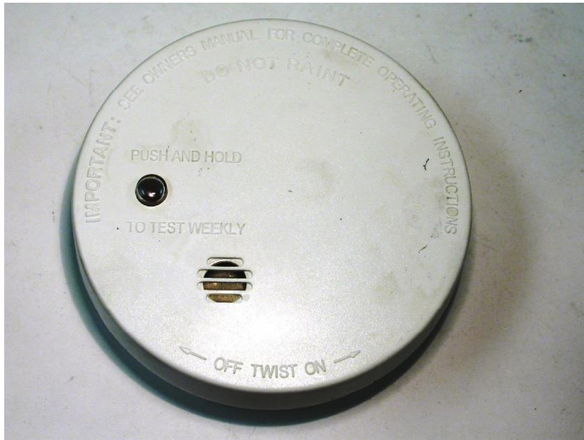
**Figure 22.19** This figure shows the external cover of an FSBI alarm that did not sound during exposure to the smoldering to flaming cabinet assembly.
