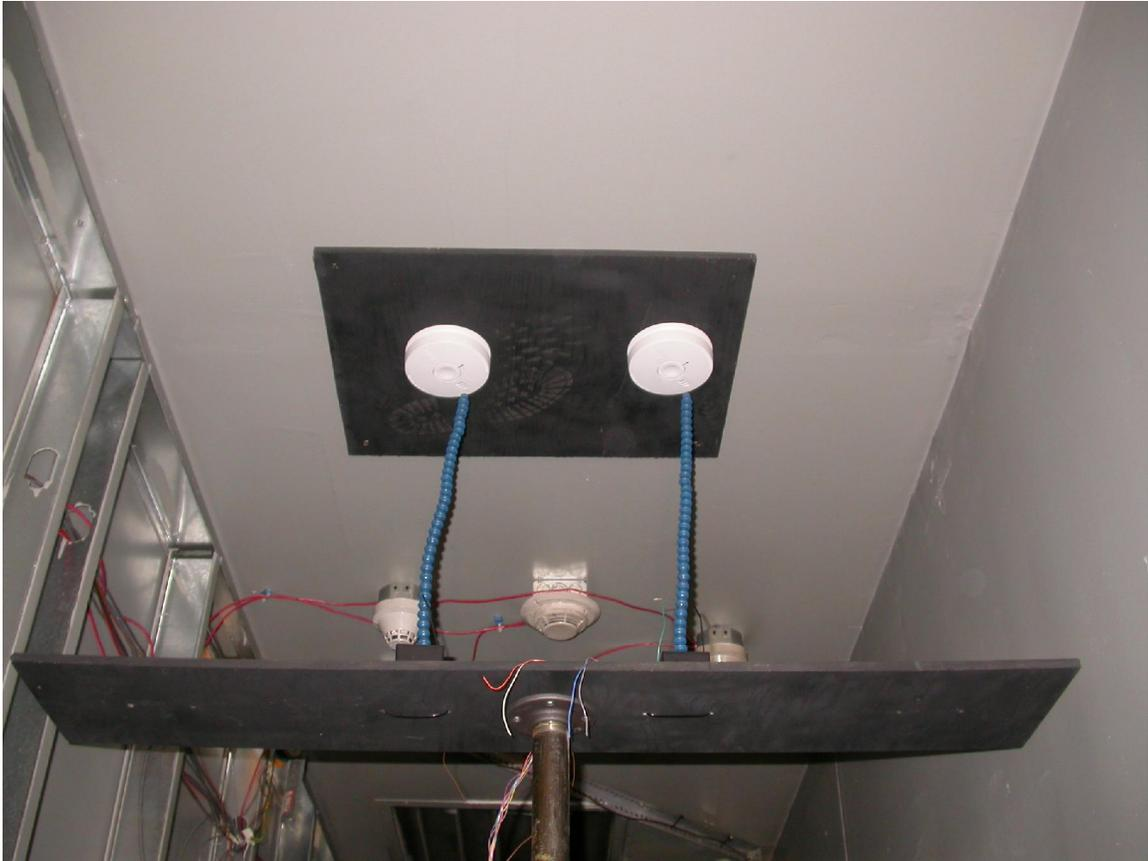
**Figure 6.2 The bank of alarms mounted in the hallway for Test Series 1. The bank consisted of one pair of new FBI alarms, one enabled and one disabled.**
