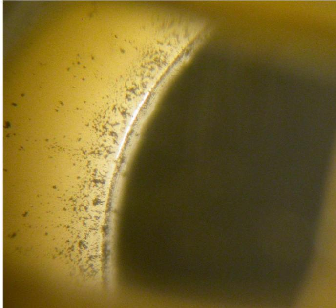
**Figure 23.16** This is a microscopic view of the internal face of the alarm horn opening from the alarm in Figures 23.13-23.15. The enhanced soot deposition visible is evidence of the alarm sounding.
