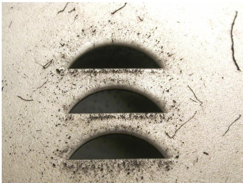
**Figure 21.2** This is a macroscopic view of the horn openings of the alarm in Figure 21.1. Enhanced soot deposition is apparent around each of the openings as evidence that the alarm sounded.
