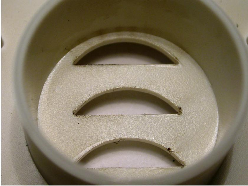
**Figure 22.3 This is a macroscopic view of the internal face of the horn openings of the alarm pictured in Figures 22.1 and 22.2. There is evidence of enhanced deposition along the flat edges and corners of the horn openings.**
