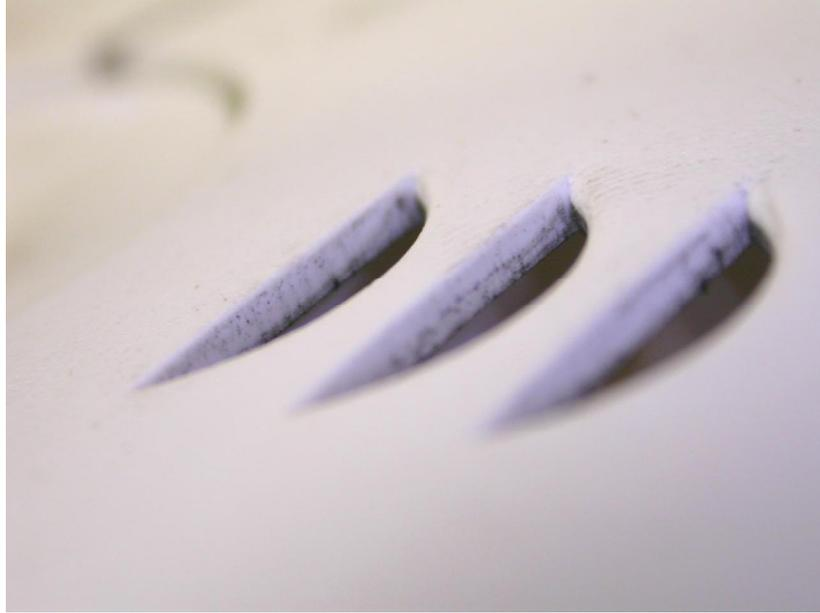
**Figure 13.5 This figure along with Figures 13.6 and 13.7 show views of the vertical face of the alarm horn opening. All three photos show darker deposition on the vertical face than was apparent on the external face of the alarm horn opening. The density decreases from the internal towards the external face on the vertical face. The depositions are the whole vertical face and not just on the corner between the vertical and internal faces.**
