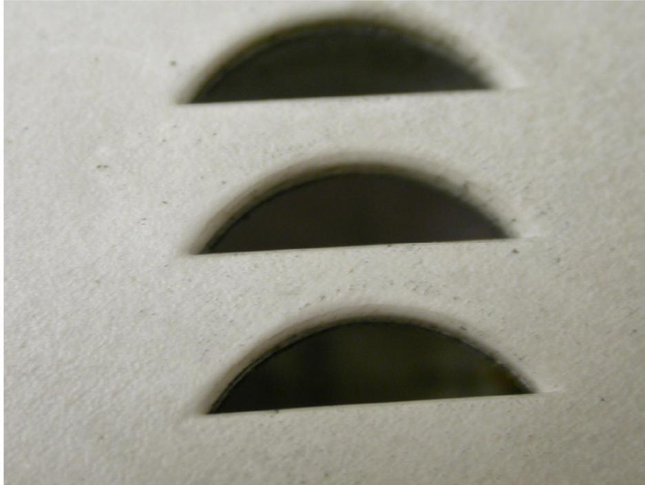
**Figure 7.22** This is the external face of the bottom alarm in Figure 7.21. There is some visible soot deposited but no evidence of enhanced deposition.
