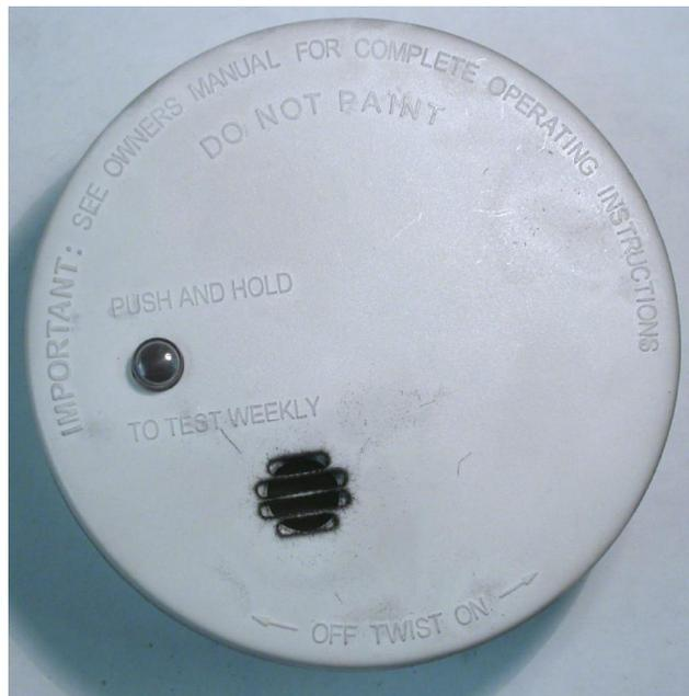
**Figure 17.24** This figure shows the external cover of an FSBI alarm that sounded during exposure to a flaming polyurethane fire. Enhanced soot deposition is evident even from this view.
