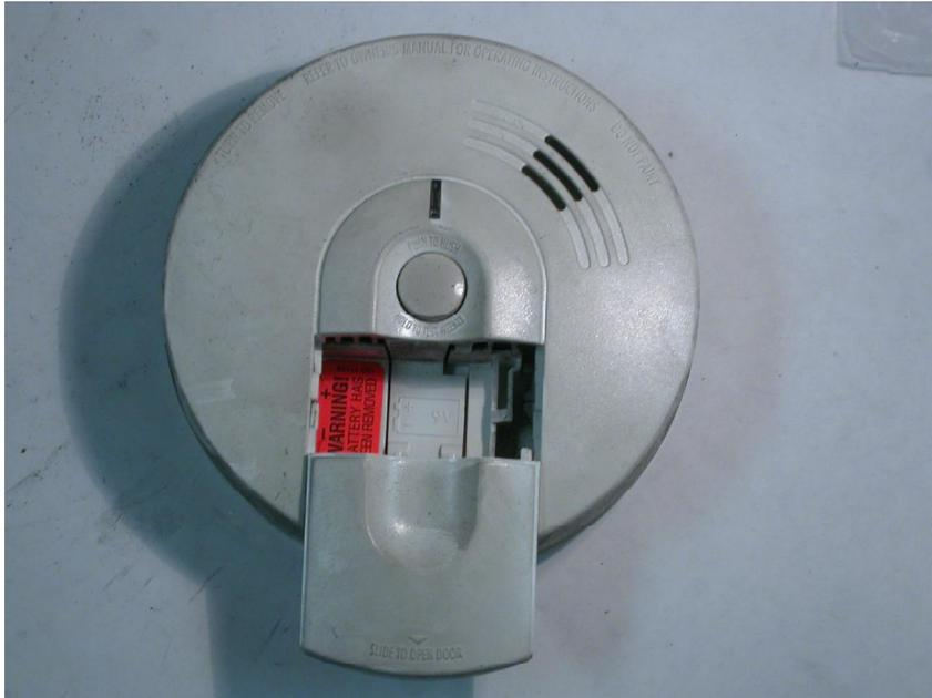
**Figure 21.12** This figure shows the exterior of the alarm cover of an alarm that did not sound during exposure to a flaming box with cups fire.
