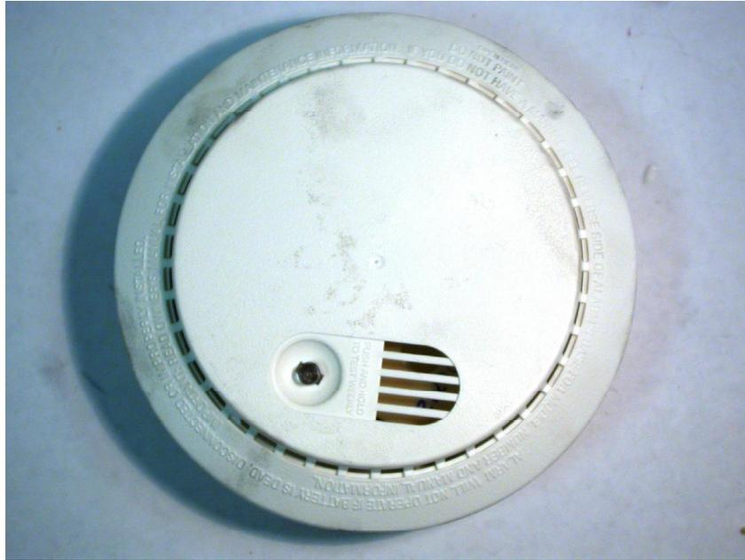
**Figure 18.11** This figure shows the exterior cover of an FGBI alarm that sounded during exposure to a flaming wood fire.
