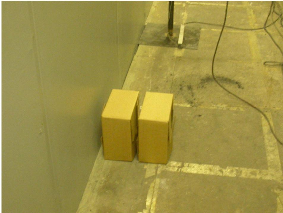
**Figure 6.15 The arrangement of the boxes with cups used in Test Series 3. The boxes were ignited in the central flue space with a butane lighter.**
