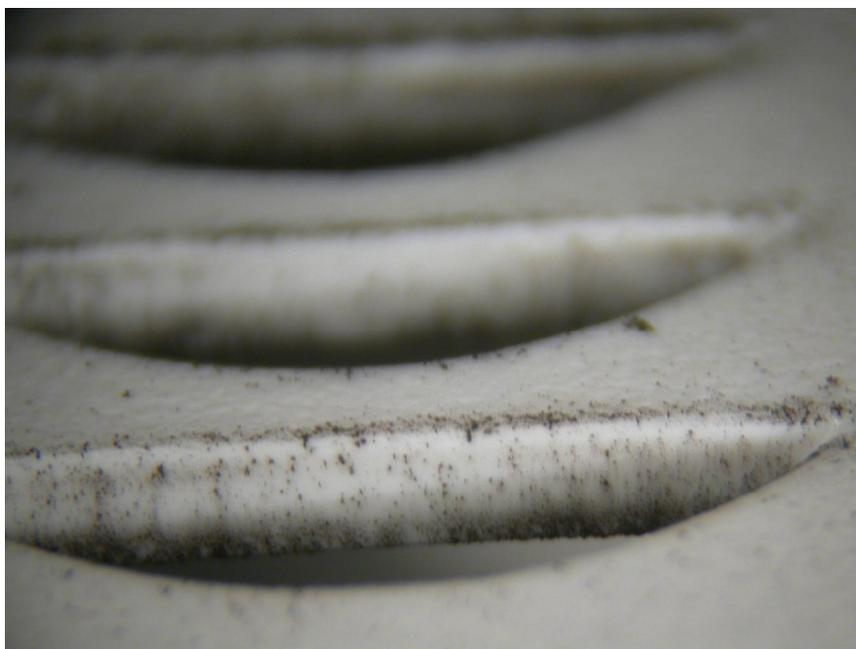
**Figure 7.31** This figure shows enhanced soot deposition on a vertical face of an FBI alarm that sounded during exposure to a flaming polyurethane fire. The deposition starts at higher density close to the internal face and decrease toward the external face. Compare this to Figure 7.32.
