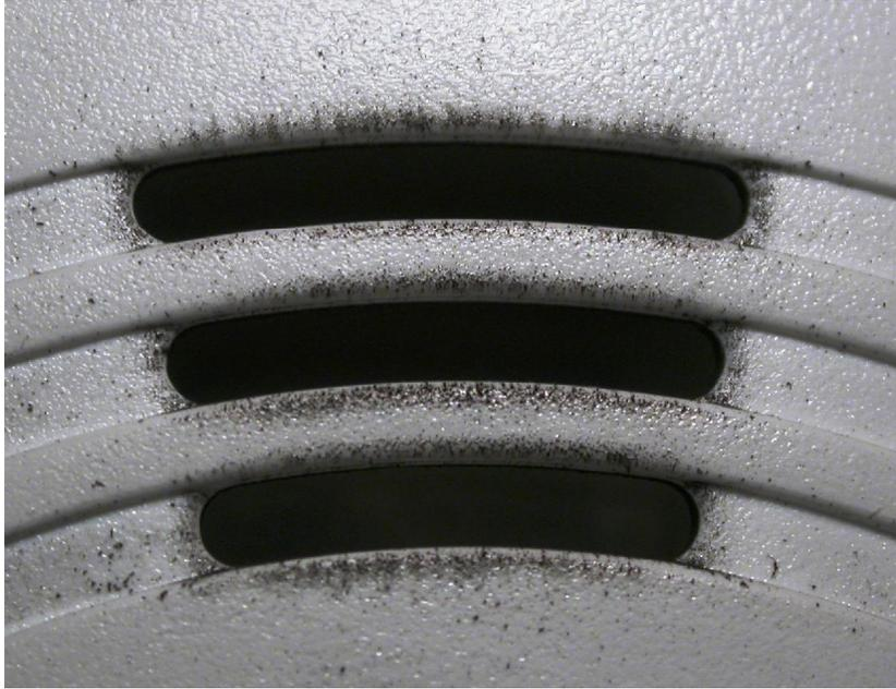
**Figure 17.19** This is a macroscopic view of the external face of the horn openings of the alarm pictured in Figure 17.18. This alarm did sound during exposure to a flaming polyurethane source and shows evidence of enhanced soot deposition.
