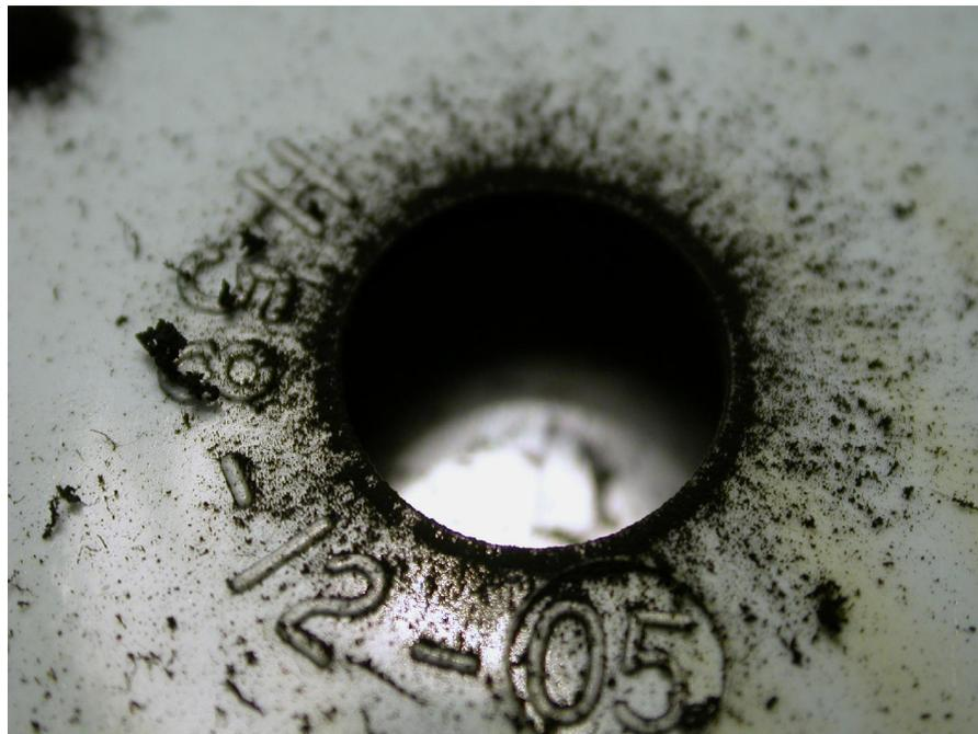
**Figure 7.7** An example of enhanced soot deposition with radial characteristics on the external face of an FGBI smoke alarm horn opening. This pattern is indicative of an alarm which sounded during exposure to the flaming couch fire of Experiment 4.2.
