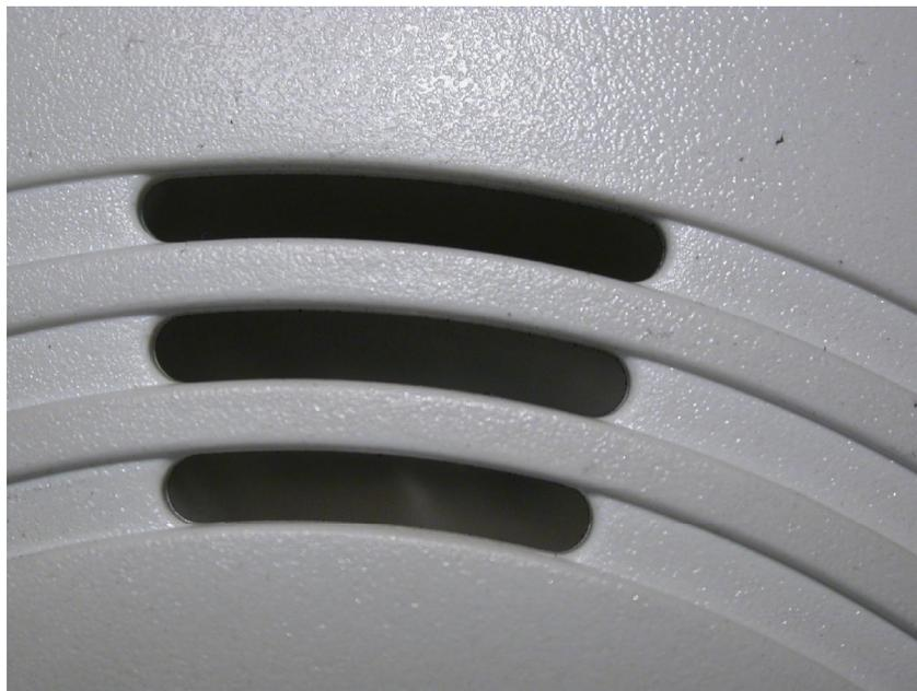
**Figure 17.22** This figure shows a macroscopic view of the external face of the alarm horn opening of the FACI alarm pictured in Figure 17.21. There is no indication of enhanced soot deposition, as this alarm did not sound during exposure to the flaming polyurethane fire.
