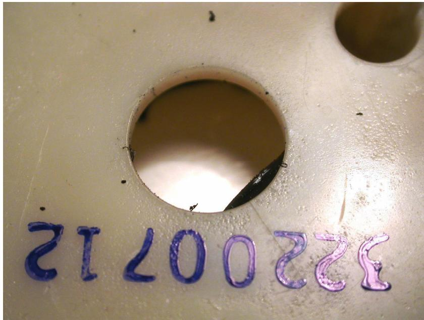
**Figure 21.21** This figure is a macroscopic view of the horn opening of the alarm from Figure 21.20. This alarm did not sound and does not show evidence of enhanced soot deposition.
