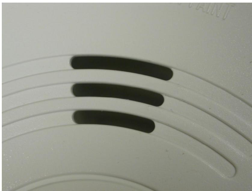
**Figure 19.4** This figure is a macroscopic view of the alarm horn openings of the alarm pictured in Figure 19.3. This alarm sounded during multiple nuisance exposures but does not show evidence of enhanced soot deposition.
