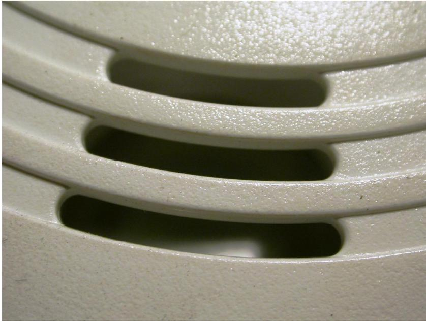
**Figure 22.13** This figure shows a macroscopic view of the horn openings from Figure 22.12. This alarm did not sound and does not show any evidence of enhanced depositions.
