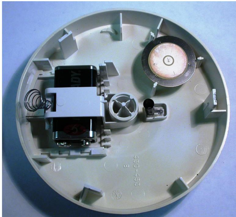
**Figure 7.19** This figure shows the interior cover of an alarm exposed to a smoldering polyurethane fire. There is a light yellow staining over the interior of the alarm cover that is seen in both alarms that sounded and alarms that did not sound.
