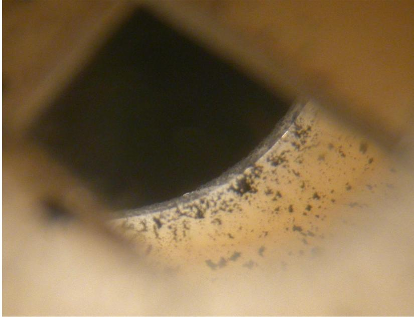
**Figure 21.19** this is a microscopic view of the internal face of the alarm horn opening from the alarm in Figures 21.15-21.18. There is evidence of enhanced soot deposition as there was on the external face of the horn opening.
