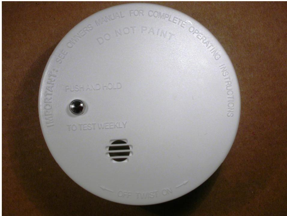
**Figure 0.11 FSBI style alarm typical of those used in this study.**
