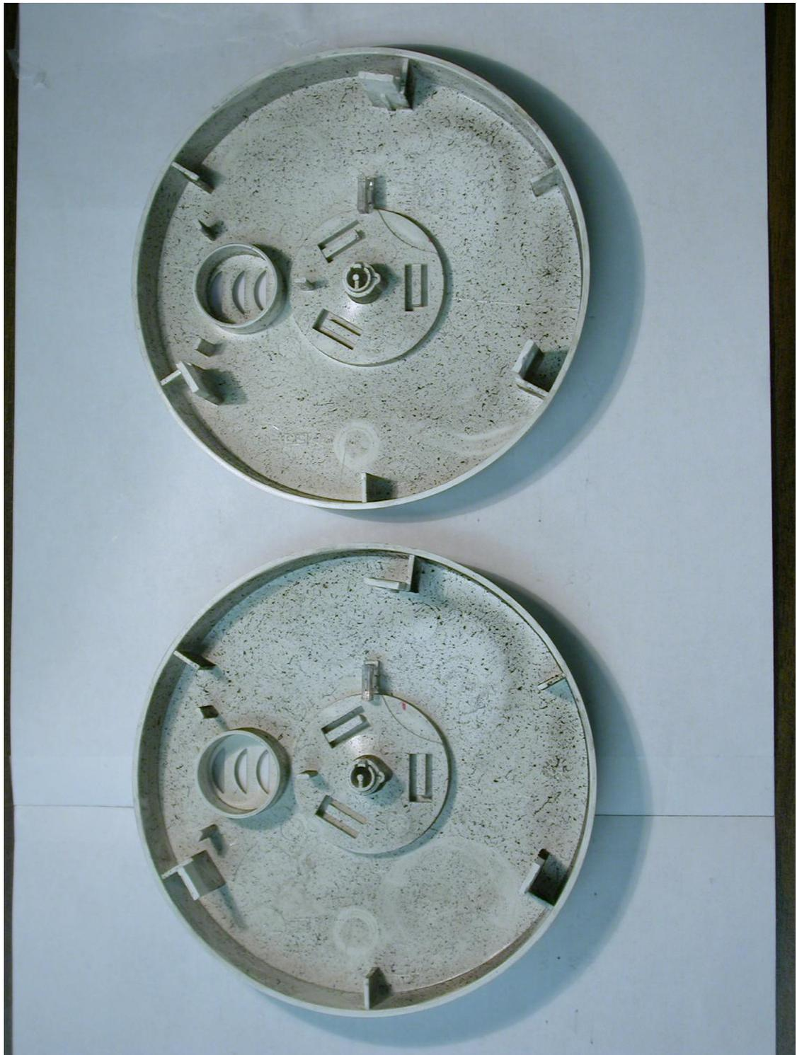
**Figure 7.21** The alarms above were mounted side-by-side. The alarm on top sounded the bottom alarm did not. In the top alarm the soot deposition inside and outside the horn chamber is comparable. In the bottom alarm the soot density outside the horn chamber is denser than the soot deposition inside the horn chamber.
