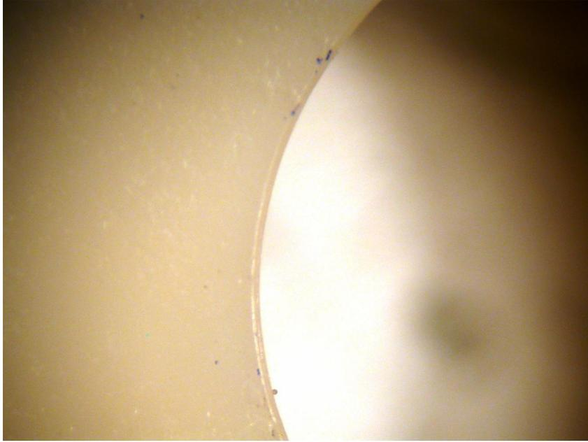
**Figure 18.13** This is a microscopic view of the alarm horn opening of the alarm pictured in Figure 18.12. This alarm sounded during exposure to a flaming wood fire but does not show evidence of enhanced soot deposition.
