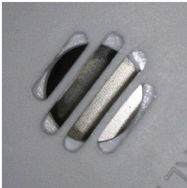
**Figure 20.8** This is a macroscopic view of the alarm horn openings from the alarm pictured in Figure 20.7. This alarm sounded but does not show any evidence of enhanced soot deposition.
