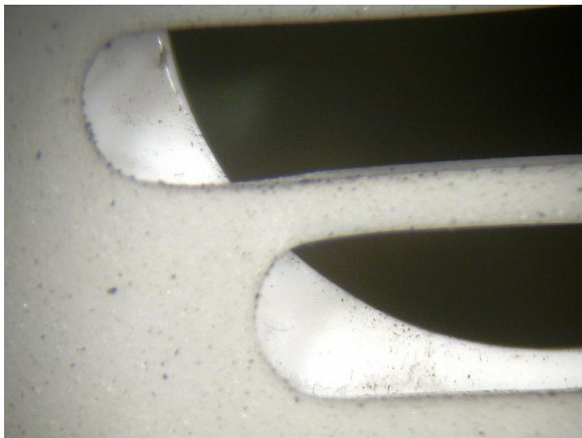
**Figure 17.30** This is a microscopic view of the alarm horn opening of the alarm from Figures 17.27-17.30. This alarm did not sound during exposure to flaming polyurethane. There is evidence of soot deposited on the horn openings but not evidence of enhanced soot deposition as pictured in Figure 17.26.
