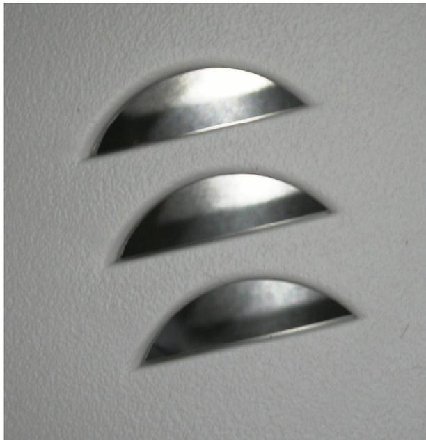
**Figure 20.2** This is a macroscopic view of the alarm horn openings from the alarm pictured in Figure 20.1. This alarm sounded but does not show any evidence of enhanced soot deposition.
