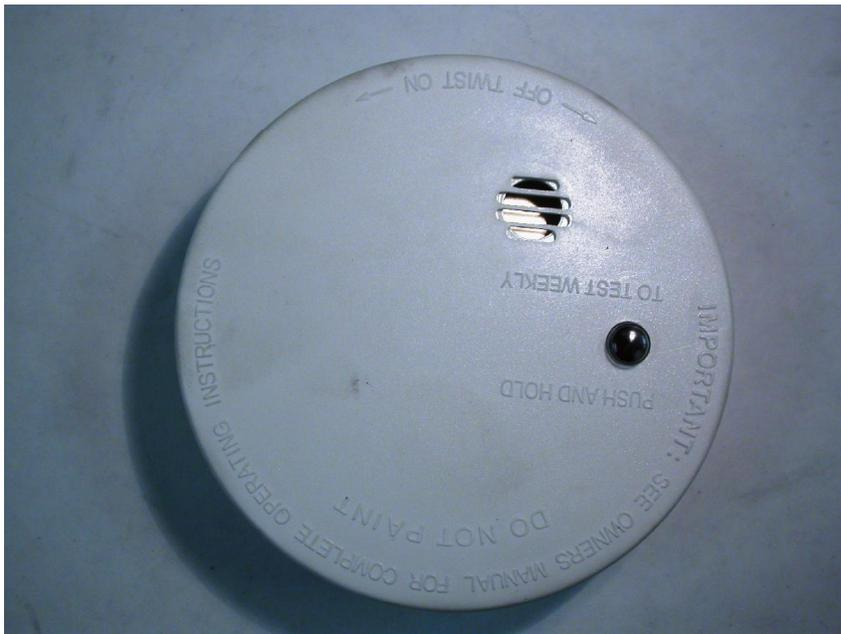
**Figure 18.14** This figure shows the exterior cover of FSBI alarm that sounded during exposure to a flaming wood fire.
