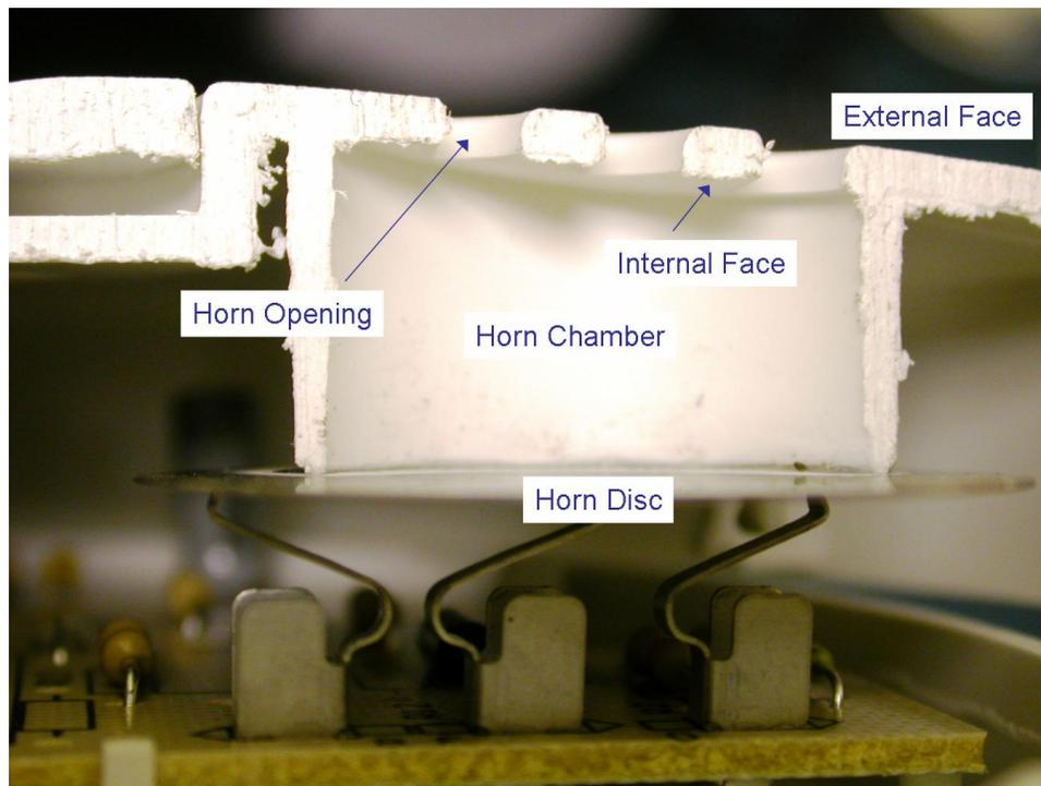
**Figure 0.14 Cross-section of an FBI horn chamber.**
