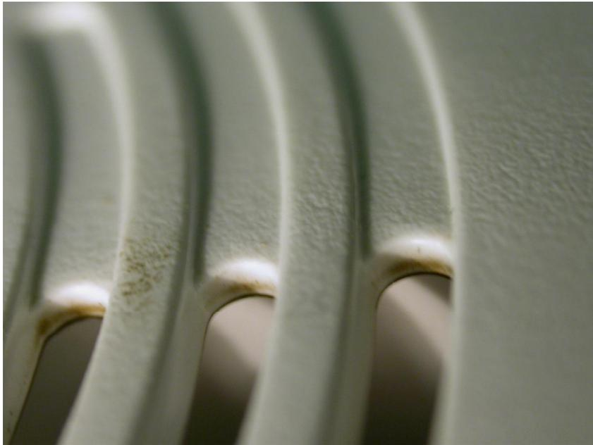
**Figure 22.10** This figure shows a macroscopic view of the vertical faces of the horn openings of the alarm pictured in Figures 22.8 and 22.9. There is evidence of enhanced depositions on all three of the vertical faces pictured.
