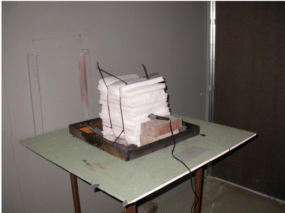
**Figure 6.4 Reformatted polyurethane source before Experiment 1.2.**
