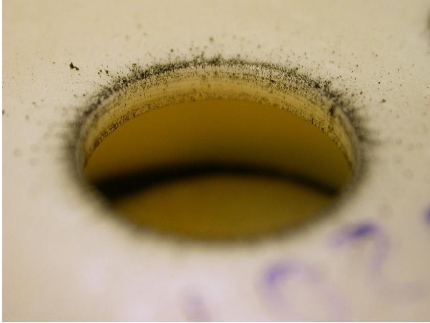
**Figure 23.15** This figure is a macroscopic view of the vertical face of the alarm horn opening from Figure 23.14. There are two bands of enhanced soot deposited proximate to the internal and external faces of the alarm horn openings, further evidence of alarm sounding.
