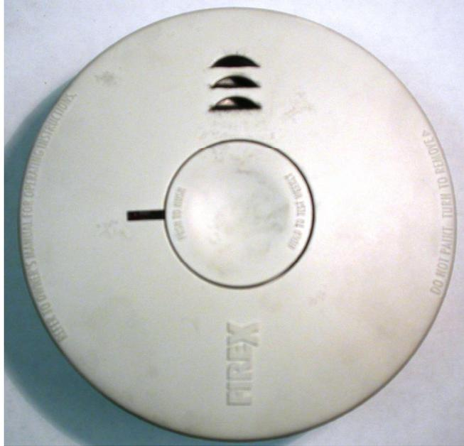
**Figure 17.1** This figure shows the exterior of the alarm cover of an alarm that sounded during exposure to a flaming polyurethane fire source. Enhanced soot deposition patterns with radial characteristics are barely visible in this figure around the alarm horn openings.
