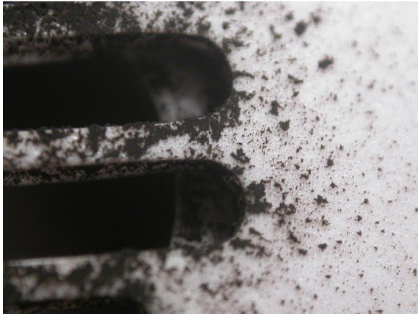
**Figure 21.24** This is a microscopic view of the alarm horn openings from Figure 21.23. This shows the high density of soot deposition and larger agglomerates closer to the horn openings.
