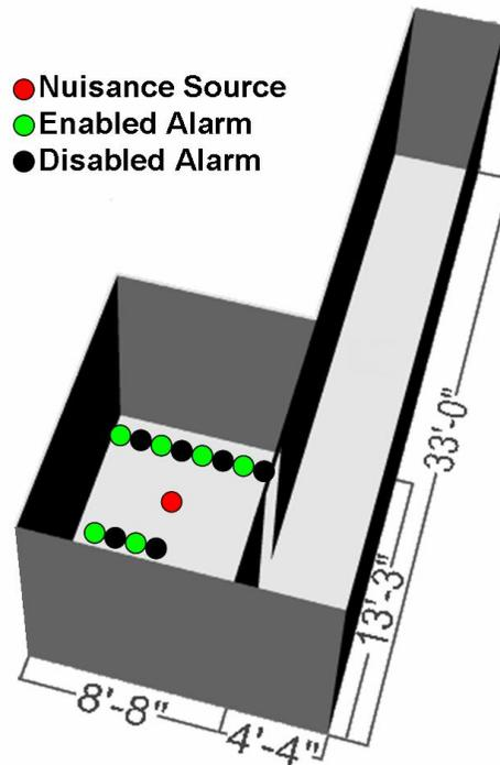
**Figure 4.3 Test Series 2 compartment configuration.**
