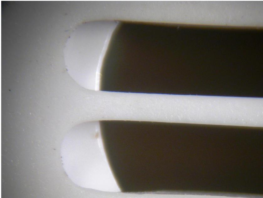
**Figure 16.5** This is a microscopic view of the horn openings from the alarm pictured in Figure 16.4. This alarm did not sound during exposure to a smoldering polyurethane fire source and does not show evidence of enhanced soot deposition.
