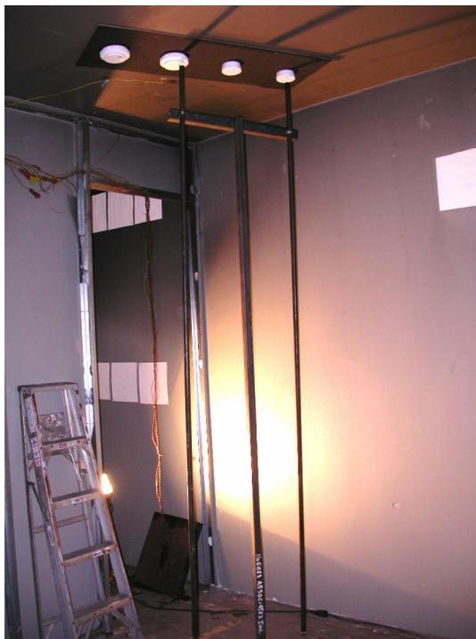
**Figure 6.16 Alarms mounted in the fire room for Test Series 4. The plastic Loc-Line hose was replaced for these alarms with 1 ¼” metal pipe due to the high temperatures expected at the detectors. The bank consists of two pairs of new alarms enabled and disabled.**
