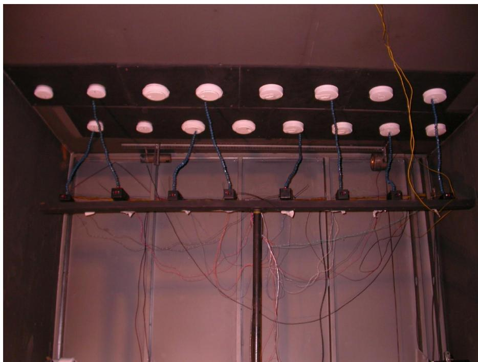
**Figure 6.17** The alarm bank mounted in Room A for Test series 4. The bank consists of one row of new alarm pairs enabled and disabled and one row of alarms previously exposed in Test Series 2 enabled and disabled.
