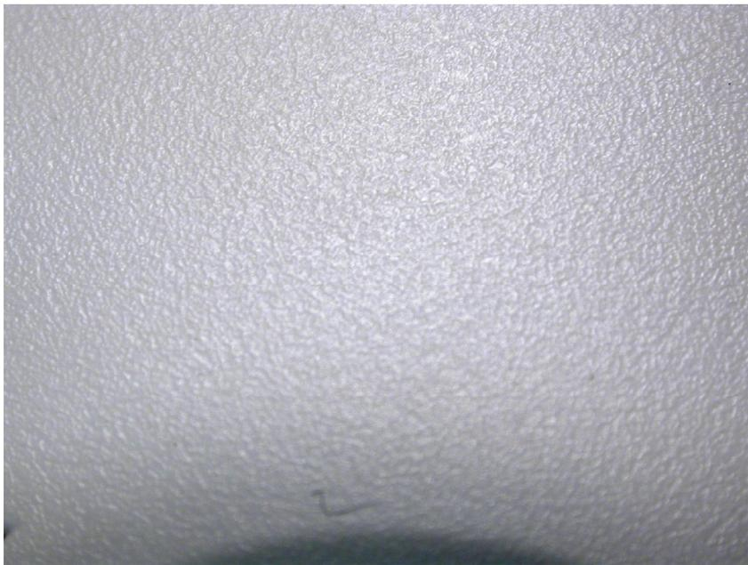
**Figure 18.8 This figure shows the ambient soot deposited on the exterior cover of the alarm that did not sound during exposure to a flaming wood fire.**
