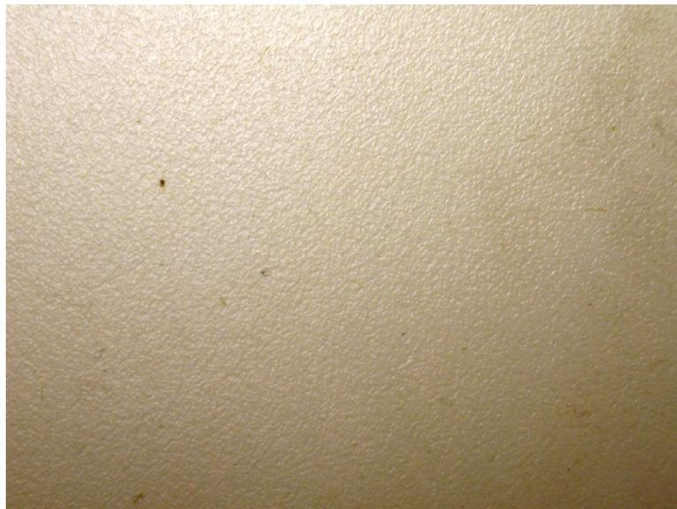
**Figure 13.4** This figure contains the ambient soot deposition on the external cover of the smoke alarm. This photo was taken at the same magnification as Figure 13.3 to allow the comparison of soot deposition density proximate and farther from the horn openings (approximately 2 cm). There is little appreciable soot deposited on the alarm cover compared to the horn opening supporting the identification of enhanced soot deposition indicative of sounding.
