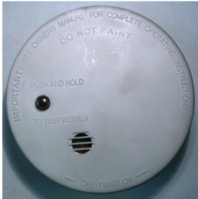
**Figure 17.27** This figure shows the external cover of an FSBI alarm that did not sound during exposure to flaming polyurethane.
