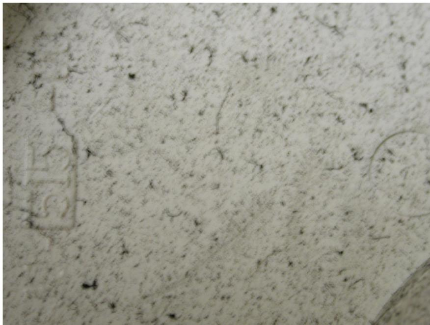
**Figure 7.25** This is the ambient soot deposition on the body of the alarm in Figure 7.24. This photo is taken at the same magnification as the previous figure. Notice the higher density and similar agglomerate size of soot in this figure to the last figure. The difference in deposition density is an indication the alarm did not sound.
