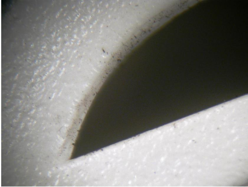
**Figure 17.9** This figure contains a microscopic view of the external face of the alarm horn opening from the same alarm pictured in Figures 17.7 and 17.8. There is some minimal deposition around the horn opening, but it is similar in density to the ambient deposition on the alarm cover.
