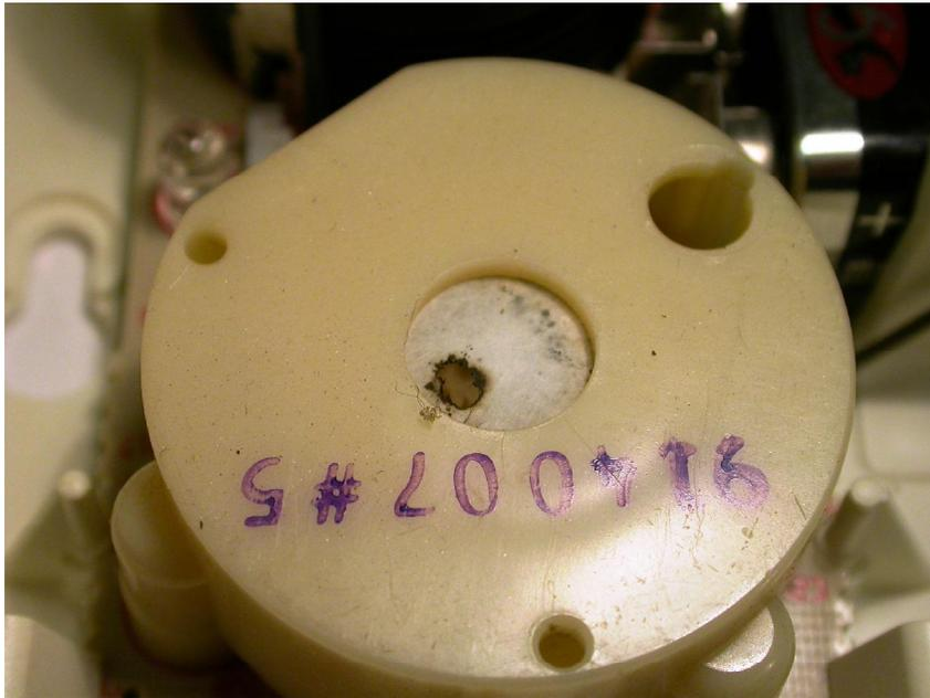
**Figure 22.22** This figure shows the alarm from Figure 22.21 post-test. This alarm sounded during the exposure and shows evidence of enhanced depositions around the improvised horn opening in the cocoon.
