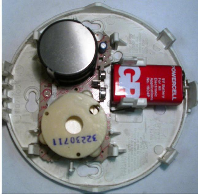
**Figure 17.15** This figure shows the interior of the alarm in Figure 17.14, an alarm that did not sound during exposure to a flaming polyurethane fire.
