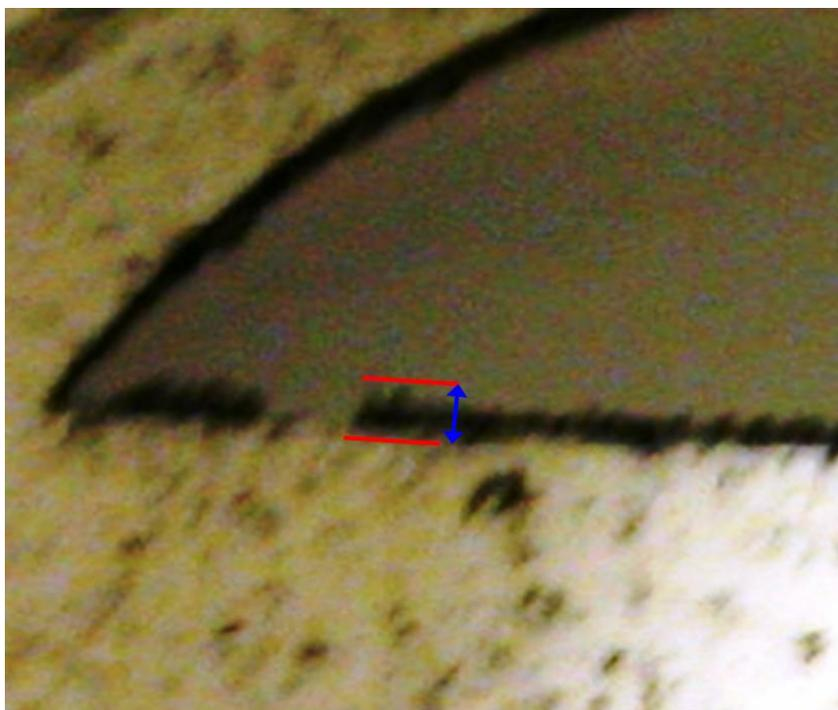
**Figure 7.18 This is an example of the measurement of the width of a misleading deposition. The dimension was measured from the one edge of the agglomerate ring to the other, red line to red line in this figure. The radial width measured in this figure in 0.22 mm.**
