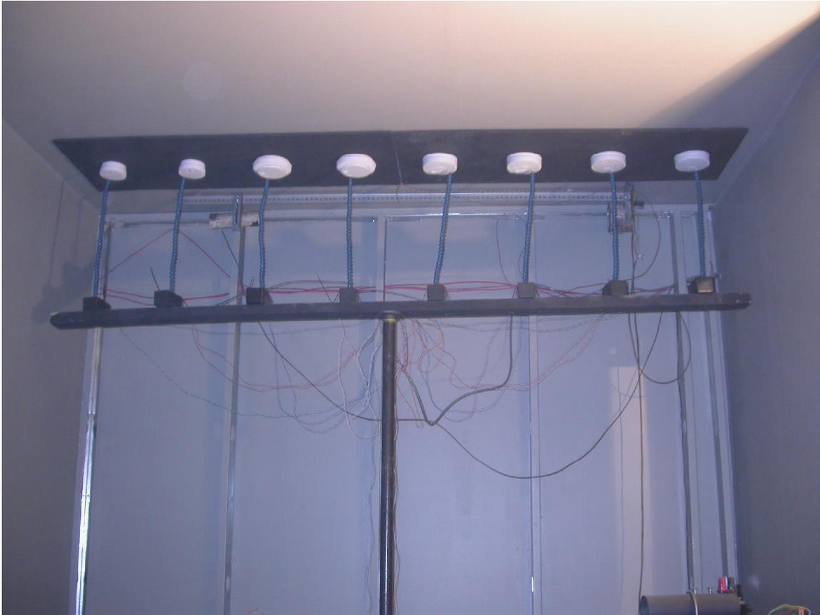
**Figure 6.1 The alarm bank mounted in Room A Test Series 1. The bank consisted of four pairs of new alarms, enabled and disabled. One pair each of FBI, FGBI, FSBI, and FACI alarms.**
