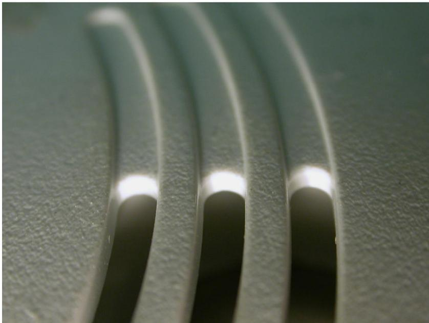
**Figure 22.14** This figure is a macroscopic view of the horn openings from Figure 22.13. The alarm did not sound during the exposure and shows no evidence of enhanced deposition on the vertical faces.
