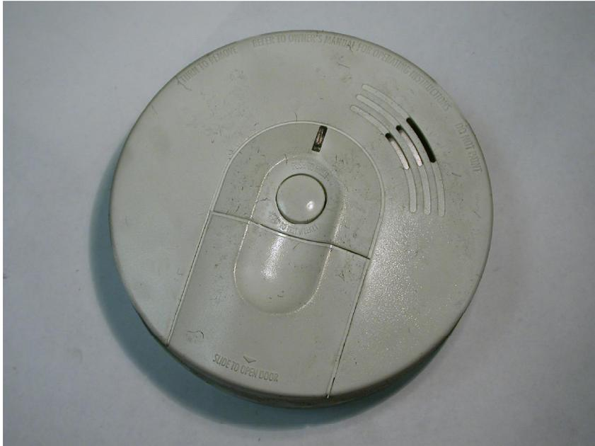
**Figure 23.10** This is the external cover of an FACI alarm that did not sound during exposure to the flaming couch fire.
