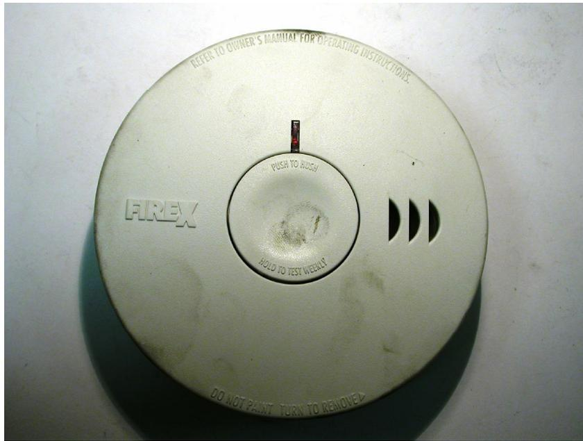
**Figure 22.5** This figure shows the alarm cover of an FBI alarm that did not sound during exposure to the smoldering to flaming cabinet assembly.
