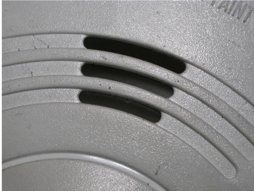
**Figure 21.13** this is a macroscopic view of the horn openings from the alarm pictured in Figure 21.12. This alarm did not sound and does not show evidence of enhanced soot deposition.
