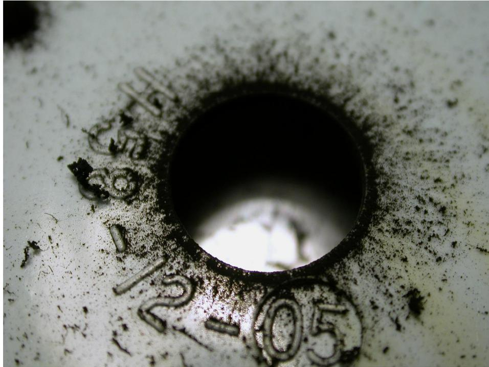
**Figure 7.13 Enhanced soot deposition on the exterior of a used alarm that sounded 45 feet away from the flaming couch fire. The density of the deposition gradually decreases from almost 100% of the area covered directly adjacent to the horn opening to deposition comparable to the ambient soot deposition on the horn. This change along with the radial direction of the soot agglomerates are what is meant by radial characteristics of enhanced deposition.**
