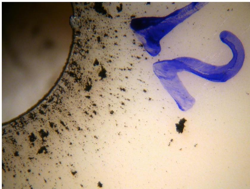
**Figure 21.18** This is a microscopic view of the horn opening of the alarm from Figures 21.15-21.17. This alarm displays enhanced soot deposition indicative of sounding with larger agglomerates and higher density soot near the opening.
