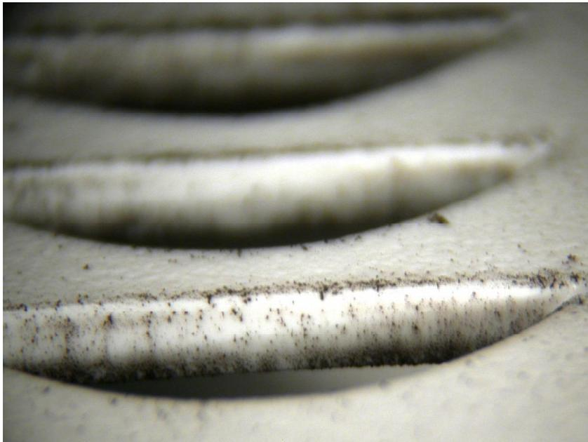
**Figure 17.4** This figure contains a macroscopic view of the vertical faces of the alarm [pictured in Figures 17.1-17.3]. This alarm sounded during exposure to a flaming polyurethane fire source. Enhanced soot deposition is visible on all three vertical faces. The deposition density moves from higher to lower density from the internal to external faces of the horn opening.
