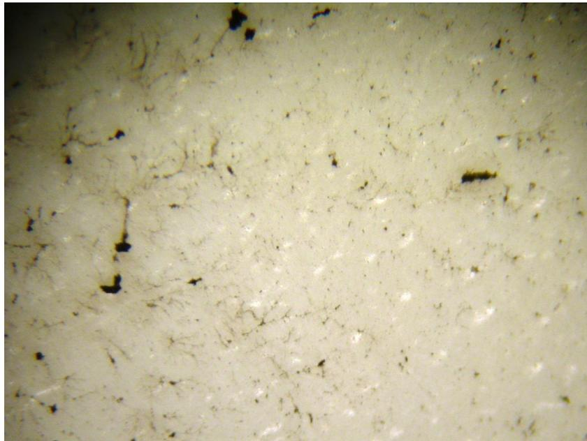
**Figure 23.2 This figure shows the ambient soot deposited on the cover of the alarm from Figure 23.1. This soot is less dense than that in enhanced depositions.**
