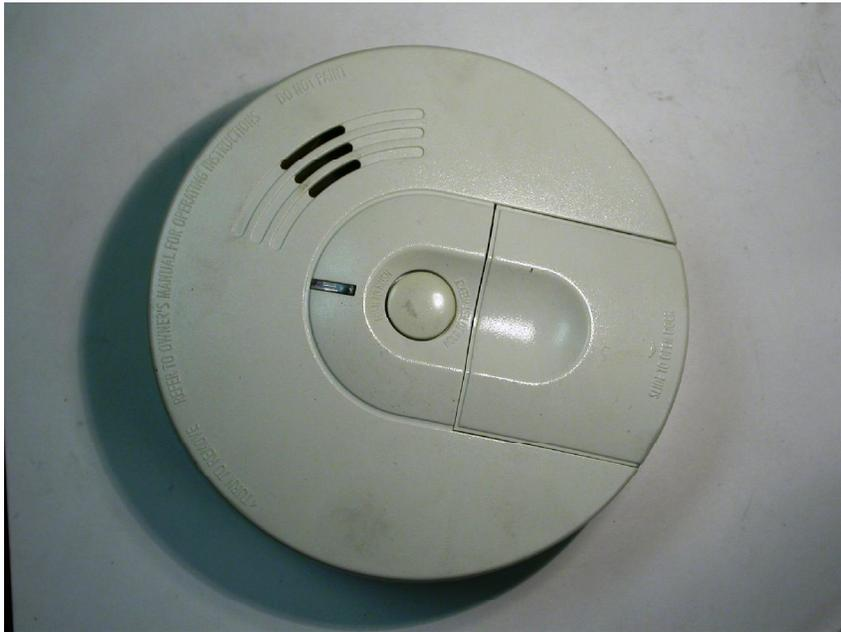
**Figure 22.8** This figure shows the external cover of an FACI alarm sounded during exposure to the smoldering to flaming cabinet assembly.
