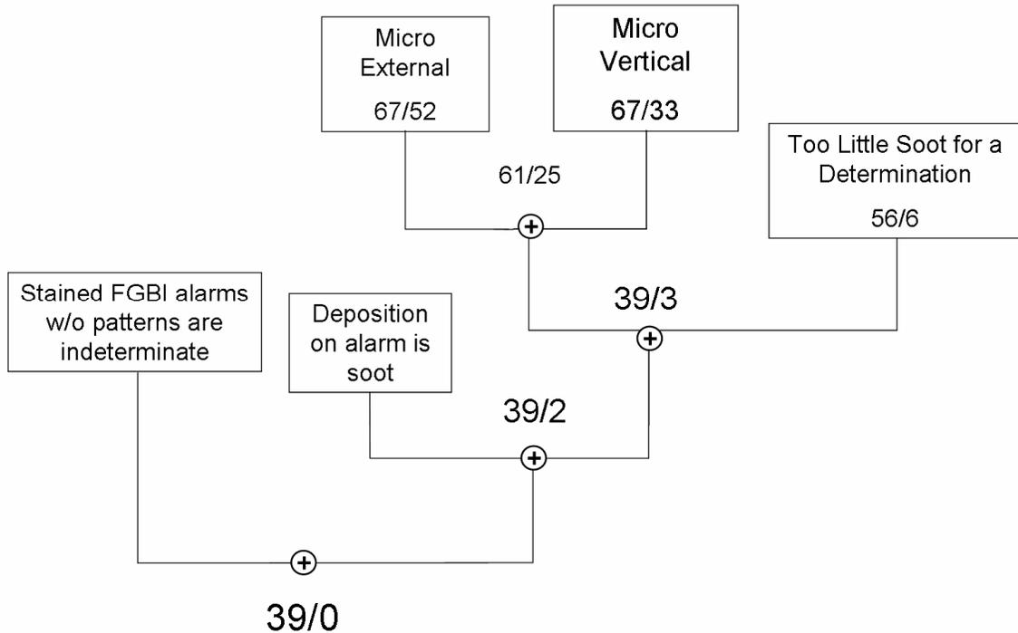
**Figure 8.2 The negative alarm sounding heuristic. The pluses represent Boolean AND combinations and the dots represent Boolean OR combinations. Combining the absence of patterns and the rules to the observations from the blind study results in 39 alarms correctly identified as not having sounded and 0 incorrectly identified.**
