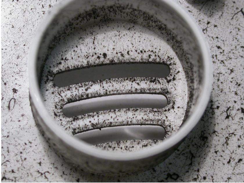
**Figure 21.11** This is a macroscopic view of the interior face of the alarm pictured in Figures 21.9-21.10. This alarm sounded and shows evidence of enhanced soot deposition. Also of note, the deposition density inside the horn chamber is of equal or greater density than that outside the horn chamber.
