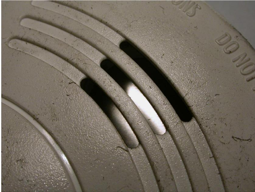
**Figure 23.11** This is a macroscopic view of the horn openings from the alarm in Figure 23.10. This alarm did not sound and does not show any enhanced soot deposition.
