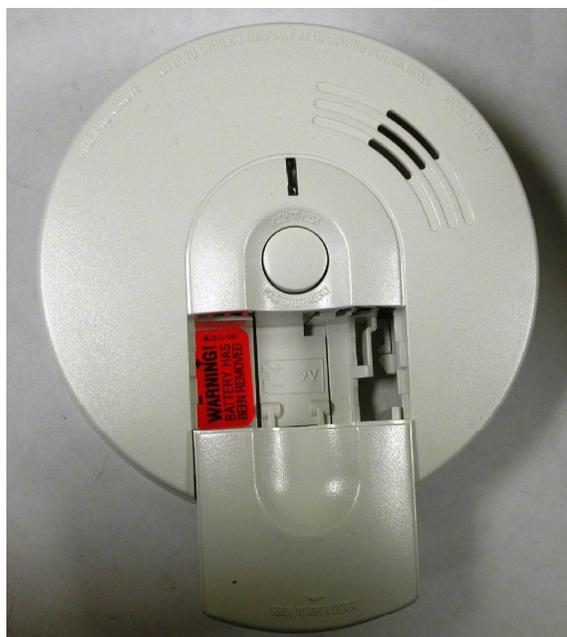
**Figure 19.3** This figure shows the exterior cover of an FACI alarm that sounded during multiple nuisance exposures.
