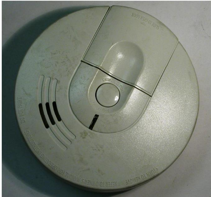
**Figure 22.12** This figure shows the external cover of an FACI alarm that did not sound during exposure to the smoldering to flaming cabinet assembly.
