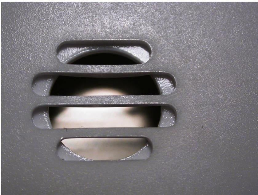
**Figure 16.4** This figure shows a macroscopic view the alarm horn openings of an alarm that did not sound during exposure to smoldering polyurethane fire source. There is no evidence of enhanced deposition around the horn openings as there were on the alarm pictured in Figures 16.1-16.3, which did sound.
