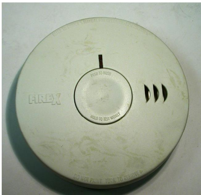
**Figure 22.1** This figure shows the external cover of an FBI alarm sounded during exposure to the smoldering to flaming cabinet assembly.
