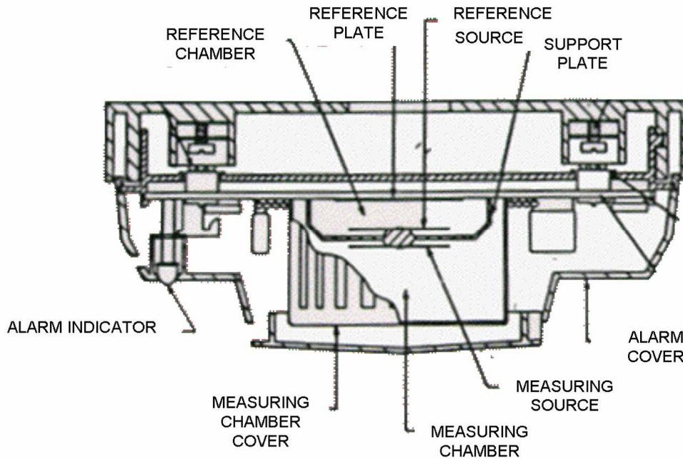
**Figure 2.2 Ionization Smoke Detector Diagram.**
