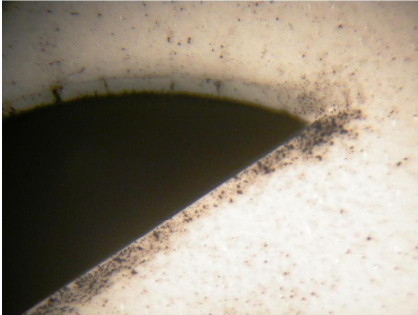
**Figure 17.3** This is a macroscopic view of one of the moon shaped openings of the alarm from Figures 17.2 and 17.3. This alarm sounded during exposure to a flaming polyurethane source. Enhanced soot deposition is visible here along the bottom face and corner of the opening.
