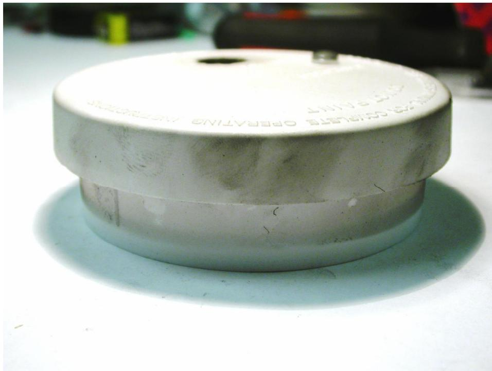
**Figure 14.8 Example of the exterior flow pattern on an FSBI alarm exposed in Experiment 4.2: Flaming Couch Exposure. Note the higher to lower soot density moving from right to left on the alarm cover, signifying smoke flow from right to left across the alarm.**
