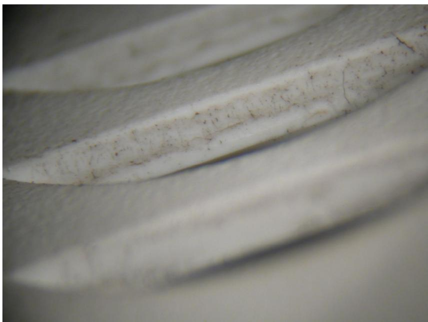
**Figure 7.32** This figure displays soot deposited on the vertical face of an FBI alarm that did not sound during exposure to flaming polyurethane. The deposition does not display any of the characteristics of enhanced deposition seen in Figure 7.31.
