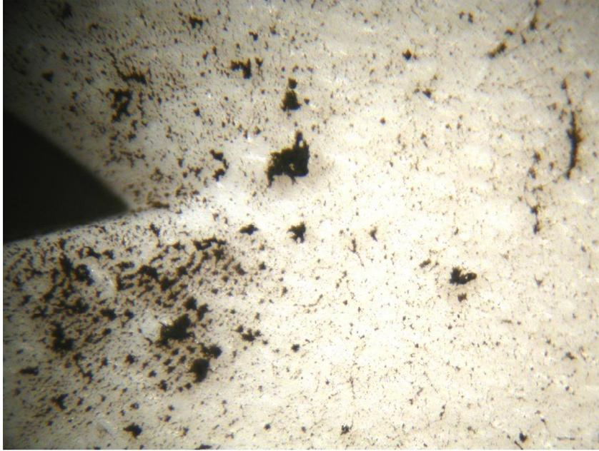
**Figure 21.3 This is a microscopic view of the corner of one of the alarm horn openings from Figure 21.2. Enhanced soot deposition is evident from the larger soot agglomerates and higher deposition density near the opening.**
