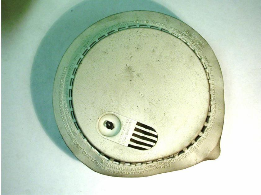
**Figure 23.17** This is the external cover of an FGBI alarm did not sound during exposure to the flaming couch fire. The cover was distorted by the elevated temperatures of the upper layer.
