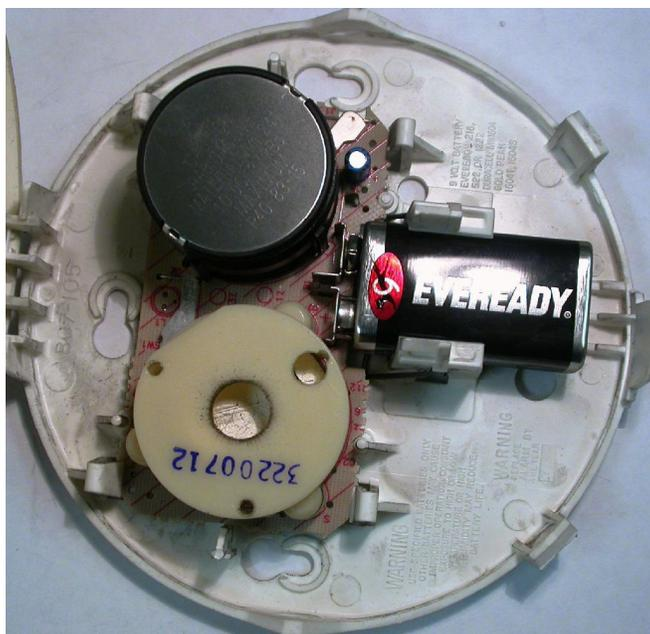
**Figure 17.11** This figure shows the interior of the same FGBI alarm seen in Figure 17.10. Enhanced soot deposition is visible on the exterior face of the alarm horn opening.
