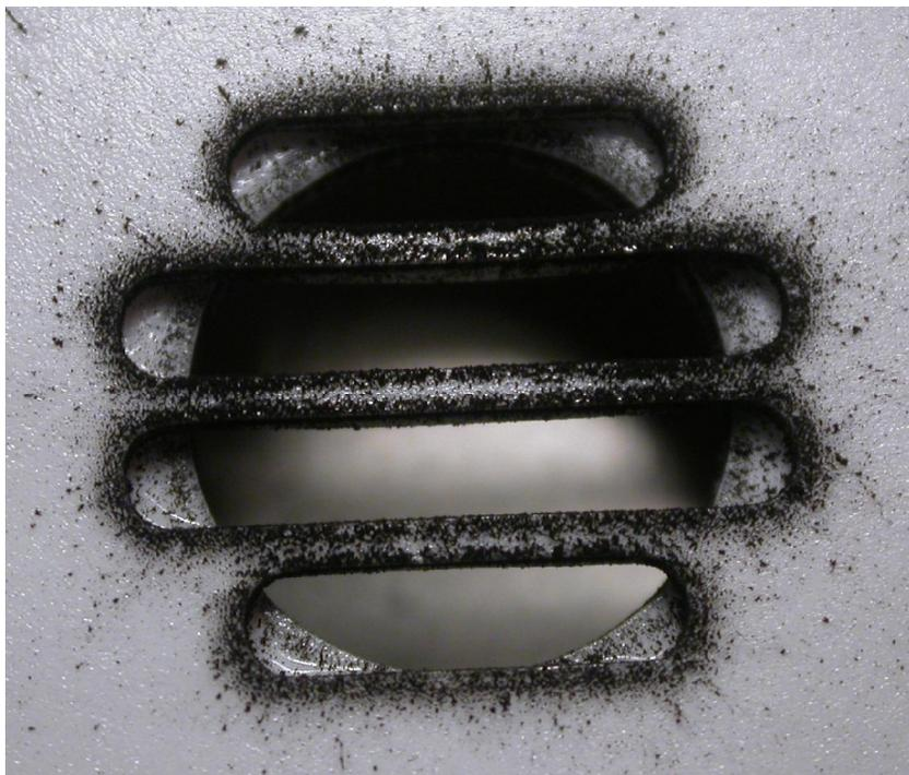
**Figure 7.27** An example of macroscopically observable enhanced soot deposition on the external face of an FSBI alarm. This is representative of the result of an alarm sounding during exposure to a flaming polyurethane exposure.
