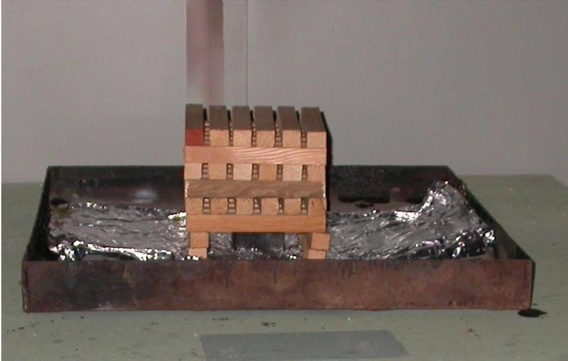
**Figure 6.6 Wood Crib source prior to Experiment 1.4.**
