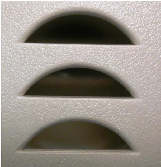
**Figure 18.2** This is a macroscopic view of the alarm horn openings pictured in Figure 18.1. The alarm sounded during the exposure, but does not show evidence of enhanced soot deposition on the exterior of the cover.
