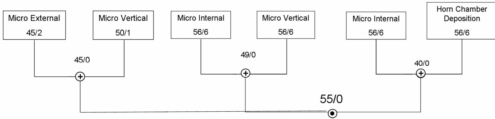
**Figure 8.1 The positive identification heuristic. Combining the observations from the blind study using the heuristic results in 55 alarms correctly identified as having sounded and 0 alarms incorrectly identified as having sounded.**
