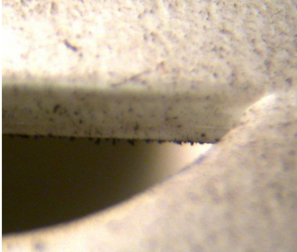
**Figure 7.16 Vertical face of the alarm pictured in Figure 7.15. This alarm did not sound but displayed potentially misleading depositions. There is no pattern on the vertical face and the deposition on the internal face can be seen hanging into the horn opening.**
