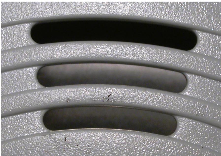
**Figure 18.10** This figure contains a macroscopic view of the alarm horn openings from the alarm pictured in Figure 18.9. This alarm sounded but does not show evidence of enhanced soot deposition on the surface.
