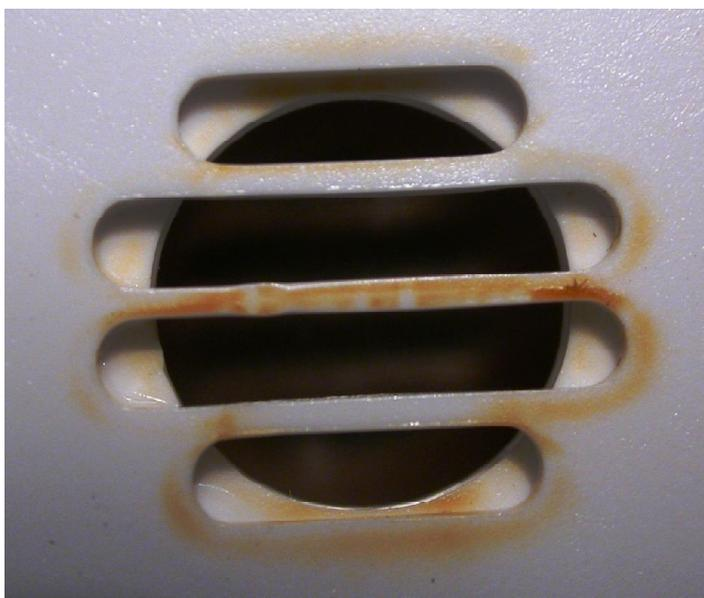
**Figure 16.2** This figure shows a macroscopic view of the exterior face of the alarm horn openings in Figure 16.1. This alarm sounded during exposure to a smoldering polyurethane fire source. Tarry enhanced soot deposition is visible around the horn openings.
