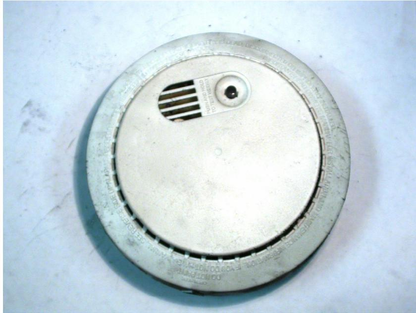
**Figure 21.15** This figure shows the external cover of an FGBI alarm that sounded during exposure to a flaming box with cups fire.
