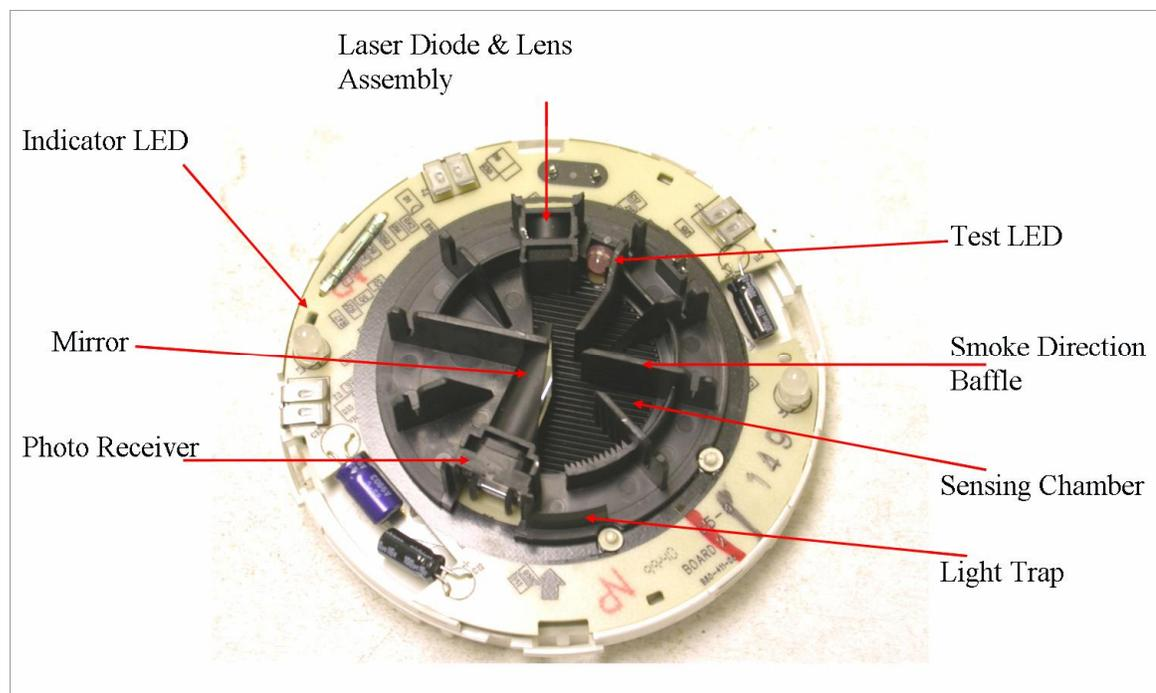
**Figure 2.1 Anatomy of a photoelectric smoke detector.**
