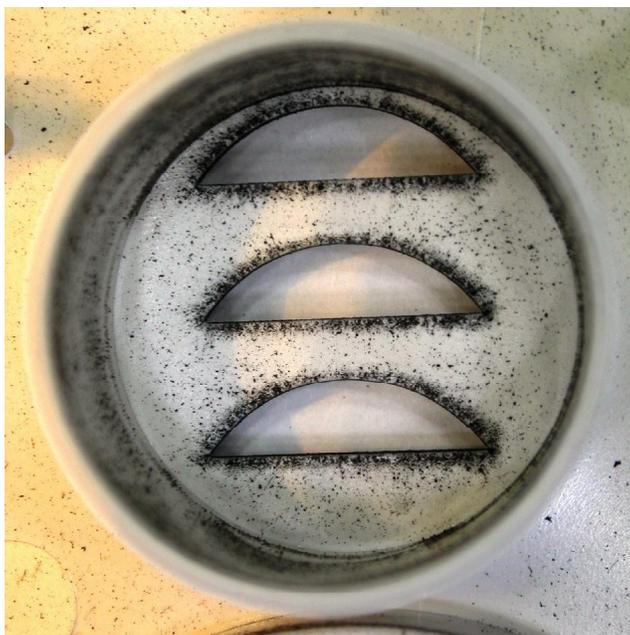
**Figure 17.6** This figure contains a macroscopic view of the interior face of the alarm horn opening of the alarm pictured in Figures 17.1-17.5. Visible is the enhanced soot deposition around the horn openings and the deposition density of equal or greater inside the horn chamber than outside the horn chamber.
