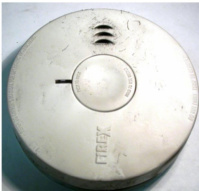
**Figure 21.1** This figure shows the exterior cover of an FBI alarm that sounded during exposure to a flaming box with cups fire. Enhanced soot deposition is visible around the horn openings.
