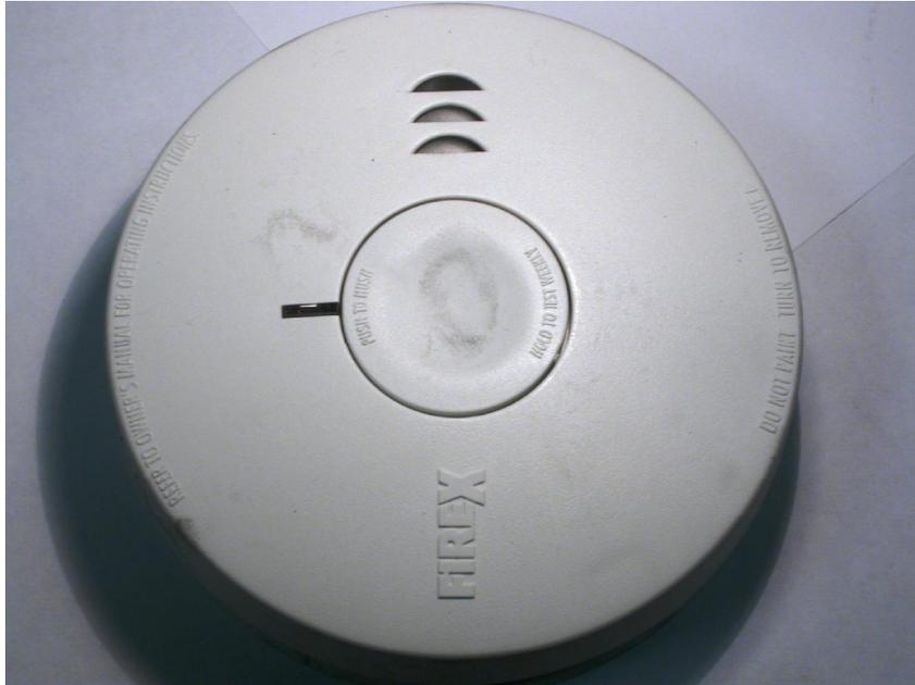
**Figure 13.1** This figure shows an overall view of the exterior of the alarm cover. Some ambient soot deposition is apparent on the alarm cover. There is not however enough soot to determine the direction of bulk flow past the alarm.
