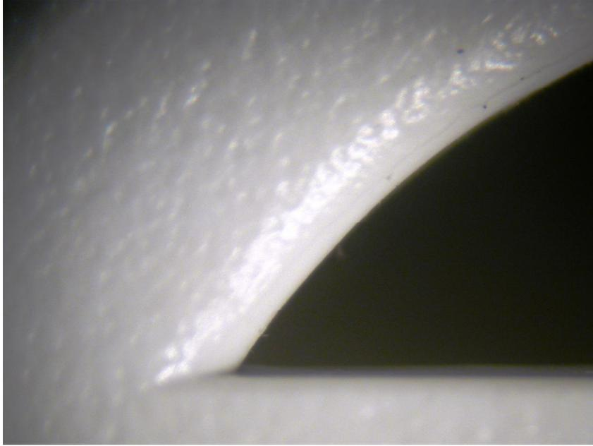
**Figure 18.3** This is a microscopic view of the alarm horn openings of Figure 18.2. There is no evidence of enhanced soot deposition on the vertical surface. This case did not present sufficient evidence to yield a determination.
