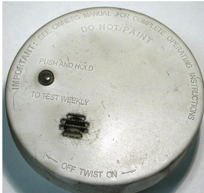
**Figure 23.19** This figure shows and FSBI alarm that sounded during exposure to the flaming couch fire. Enhanced deposition indicative of alarm sounding is visible in around the horn openings.
