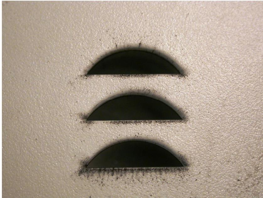
**Figure 17.2** This figure shows a macroscopic view of the exterior face of the alarm horn openings of the same alarm in Figure 17.3. This alarm sounded during exposure to a flaming polyurethane fire source. Enhanced soot deposition is visible in places around each of the moon-shaped openings.
