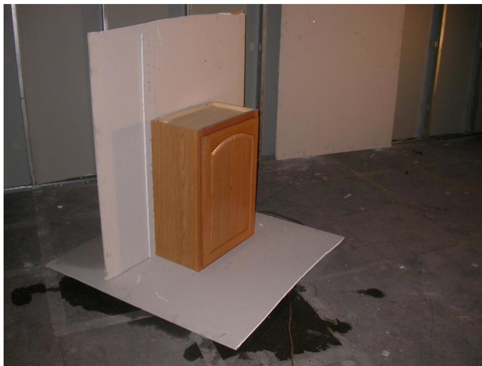
**Figure 6.19 Pre-test Cabinet Assembly burned in Test 4.1. A 500W cartridge heater was placed six inches from the floor between the dry-wall and the cabinet back. The assembly smoldered, finally transitioning to flames**
