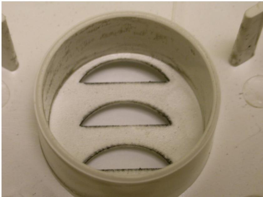
**Figure 13.10** This figure contains a macro view of the inside surface of the smoke alarm horn chamber. There is a ring of darker soot around each of the alarm horn openings. At the magnification shown the soot deposition on the internal surfaces of the alarm horn chamber appears greater than or equal to the ambient soot deposition outside the horn chamber.
