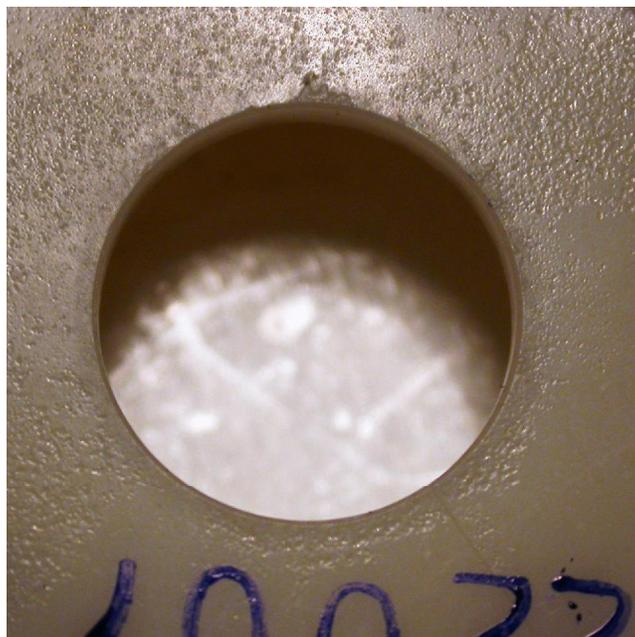
**Figure 18.12** This is a macroscopic view of the alarm horn opening of the alarm pictured in Figure 18.11. This alarm sounded during exposure to a flaming wood fire but does not show evidence of enhanced soot deposition.
