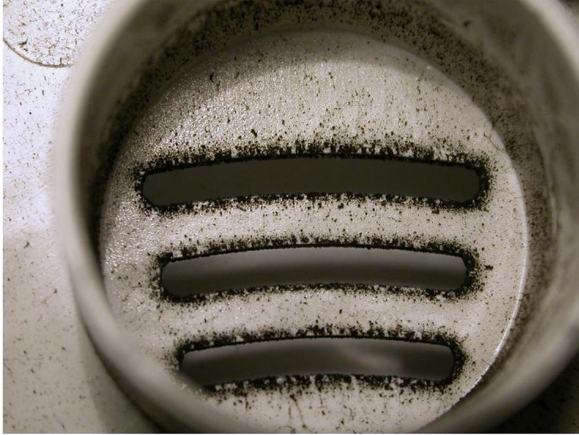
**Figure 23.9** This figure shows the internal face of the alarm horn openings from Figure 23.8. The enhanced soot deposition is more developed on the internal face than the external face, evidence of the alarm sounding. There is also more soot deposited inside the horn chamber than outside.
