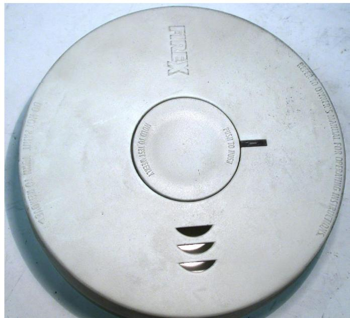
**Figure 21.6** This figure shows the exterior cover of an FBI alarm that did not sound during exposure to a flaming box with cups fire. Enhanced soot deposition is not visible around the horn openings.
