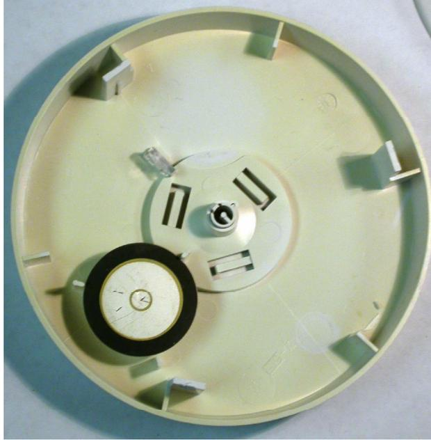
**Figure 16.9** This figure shows the interior of a smoke alarm cover that sounded during exposure to a smoldering polyurethane source. The cover shows staining characteristic of exposure to a smoldering fire source.
