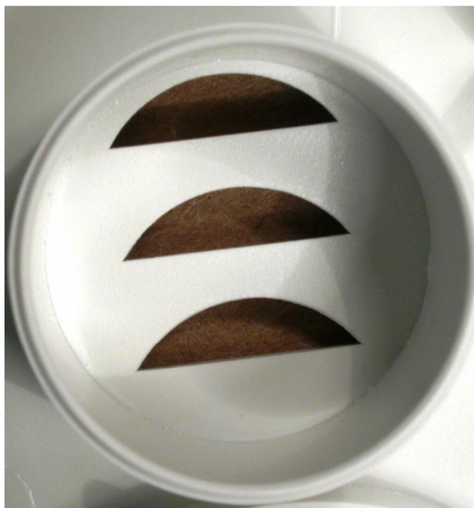
**Figure 0.8 Interior of FBI Smoke Alarm Horn Opening.**
