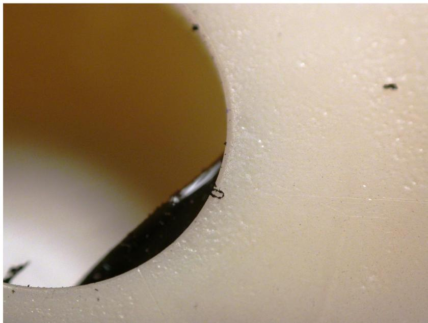
**Figure 21.22** This is a microscopic view of the horn opening pictured in Figures 21.20 and 21.21. this alarm did not sound and shows no evidence of enhanced soot deposition.
