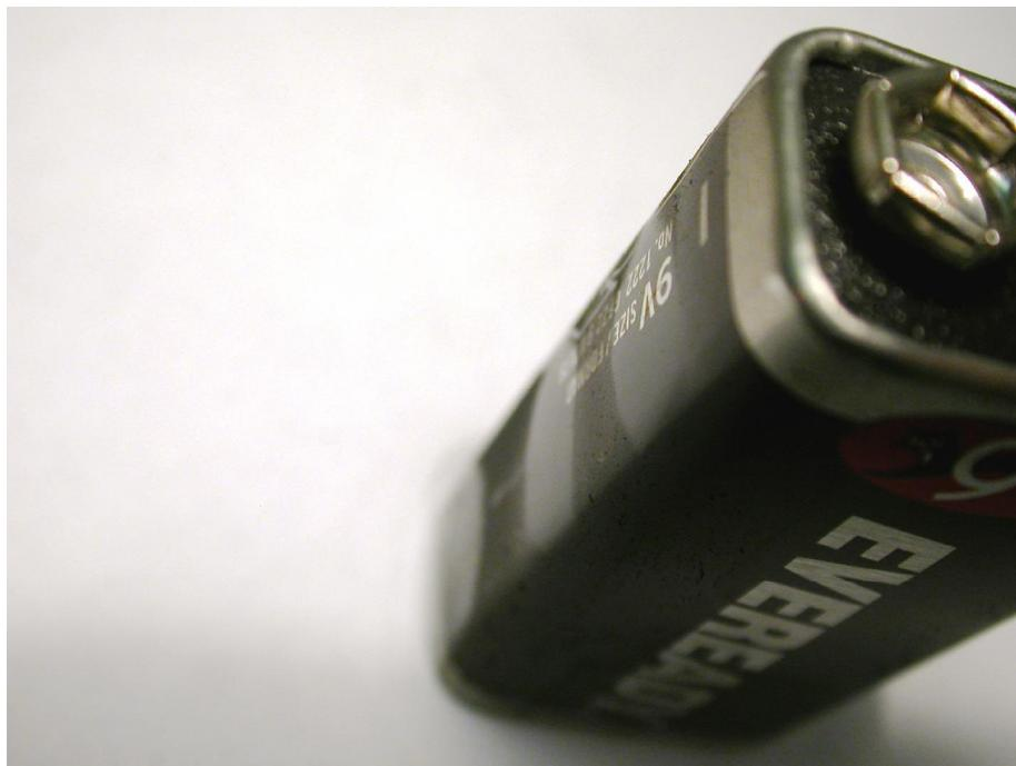
**Figure 14.3** The outline of the battery arms in the soot deposited on the battery installed in an alarm exposed to the flaming couch in Experiment 4.2.
