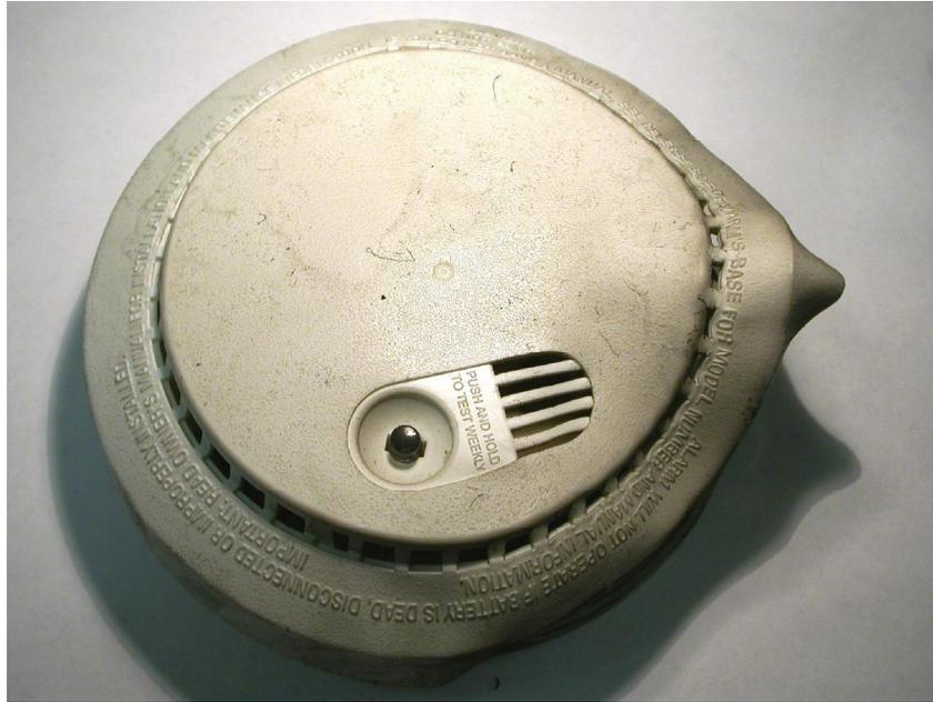
**Figure 23.13** This figure shows the external cover of the an FGBI alarm that sounded during exposure to the flaming couch section. The alarm cover was distorted by the elevated temperatures of the upper layer.
