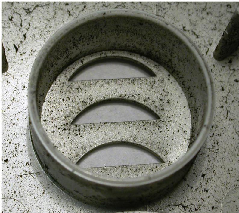
**Figure 7.26** This figure contains the horn chamber to the alarm that sounded during the same exposure as Figure 7.24. Notice the larger soot agglomerates and higher density of soot within this horn chamber than in Figure 7.24. Also, the density within the horn chamber is of equal or greater density to that outside the chamber.
