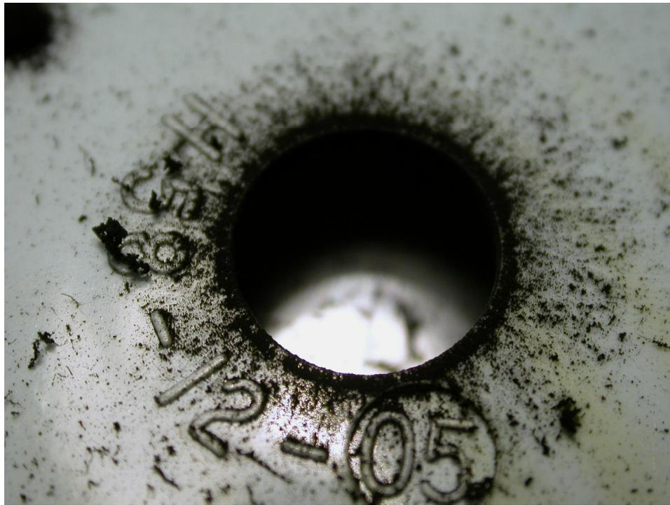
**Figure 0.17 Radial Pattern on the exterior face of an FACI horn opening.**
