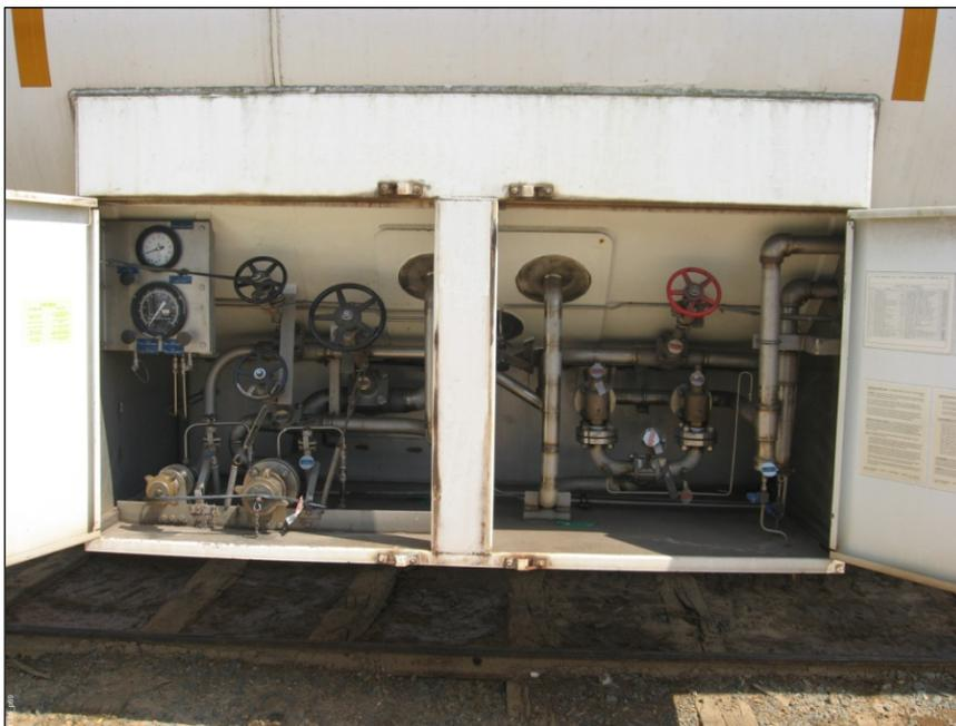
**Typical Cryogenic Liquid Tank Car Fittings Compartment**
