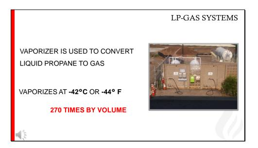
A vaporizer is used to warm the liquefied propane converting it to a vapor gas when there is a demand for large quantities of the vaporized gas. Remember, propane starts to vaporize at - 42°C or -44° F and expands at 270 times by volume.
