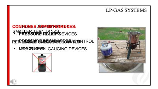
Cylinders are upright and tend to be smaller than tanks. They must conform to DOT requirements 49 CFR and CFR 178. Cylinders are refillable, however, cylinders below one pound capacity are non-refillable.
