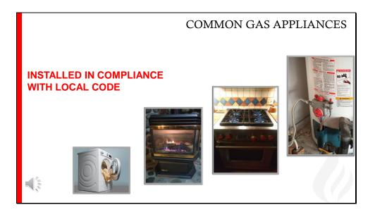
Other common fuel system appliances are water heaters, cooking stoves, fireplaces and clothes dryers. Each will have some type of ignition system and a gas control valve. Approved appliances, accessories and equipment must meet gas code requirements. Each appliance must be used with the type of gas for which it was designed and installed according to local code requirements.
