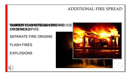
During fire or explosion events, disrupted fuel gas systems can provide additional fuel and can greatly change or increase fire spread rates, or can spread fire to areas of the structure that would not normally be burned. The flames issuing from broken fuel gas lines, called flares, can spread fire and burn through the structure.
