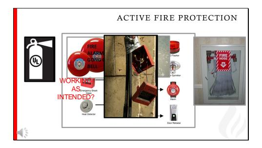
Active fire protection systems are characterized by items and/or systems, which require a certain amount of motion and response in order to work. Examples include portable fire extinguishers, standpipe and hose, fire alarms and sprinkler systems. Are they in place and working as intended? Have they been serviced as required? Are there signs of tampering?
