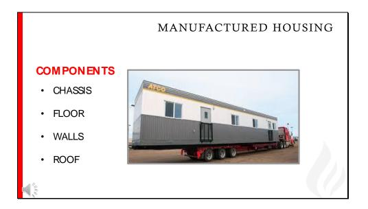
Manufactured homes have four components. They are the chassis, floor system, wall system and the roof system. The interior finish is fire-resistive and will perform similarly to regular residential construction in a fire.
