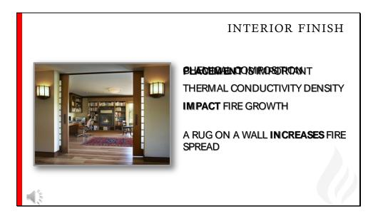
Placement of materials and total fuel loads or fuel package in a room are important. Chemical composition, thermal conductivity, and density impact fire growth and speed. Thermoplastics can greatly increase heat release rates.
