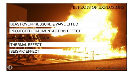
An explosion is a gas dynamic effect that, under ideal conditions, will manifest in an expanding spherical heat and pressure wave front which produces the damage characteristics of explosions. There are five major effects of explosions.
