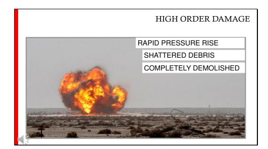
High-order damage results from relatively high blast loads specifically from a rapid rate of pressure rise. The characteristics of high-order damage include shattered walls, roofs and structural members. The building may be completely demolished. Small pulverized debris is often thrown over considerable distances, possibly a hundred or more metres.
