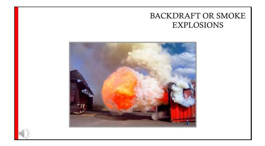
It is common for fires in rooms or other containers to become oxygen depleted which results in the generation of flammable gases due to incomplete combustion. The opening of a door or window allows air to be mixed with the gases. The gases then ignite and burn sufficiently fast to produce low-order damage. This is termed backdraft or smoke explosion. A good example of a smoke explosion can be seen in the following video.
