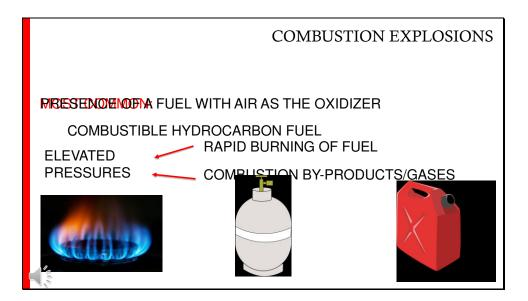
The most common explosions fire investigators encounter are caused by the burning of a combustible hydrocarbon fuel like natural gas, propane or gasoline. A combustion explosion is characterized by the presence of a fuel with air as the oxidizer. Elevated pressures are created by the rapid burning of the fuel and production of combustion by-products and gases. The reaction can accelerate to the point where an explosion occurs.
