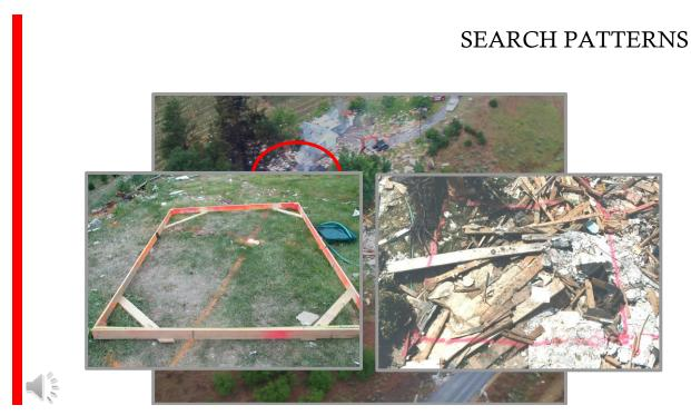
In this case, the single family home that exploded was originally located inside the red circle. The debris field stretched over hundreds of metres including several well used roads. The areas on both sides of the roads were secured and debris on the roads was thoroughly examined and then the roads were re-opened to traffic.
