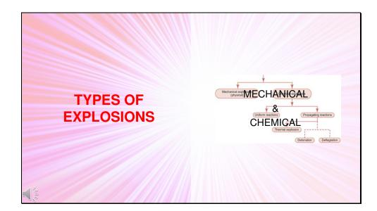
The two major types of explosions routinely involving fire investigators are mechanical and chemical. Each has subtypes which are differentiated by the source or mechanism by which the overpressure is produced.
