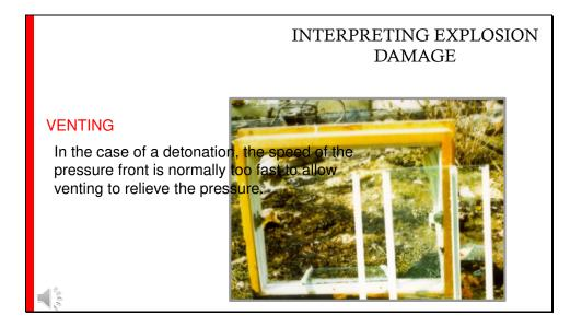
The nature of **the venting** of the containment has varying effects on explosion damage. A length of pipe may rupture in the centre allowing the gas to vent.
