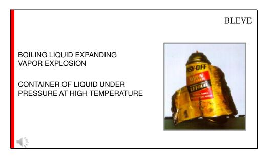
A frequent subtype of mechanical explosion encountered by fire investigators is the boiling liquid expanding vapor explosion, commonly referred to as a BLEVE. A BLEVE is an explosion involving a container of liquid under pressure at temperatures above its atmospheric boiling point. The containers may range in size from a small aerosol like that in this photograph to a much larger container like the one shown in the following video.
