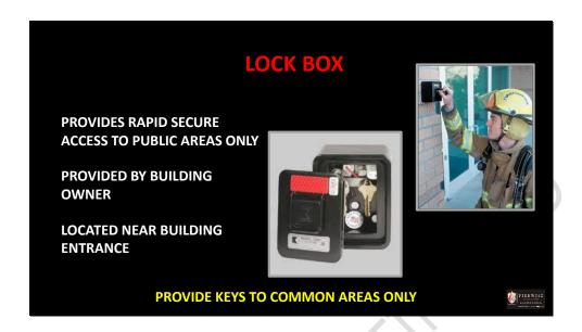
Many Fire Departments rely on a security key lock box system to enter property quickly and safely during an emergency response. The property owner purchases the Lock Box and mounts it near the main building entrance. Lock boxes should never contain keys other than for the main lobby entrance, common areas, roof access, stairwells, firefighters' elevator, or other 'public' areas in the building.
